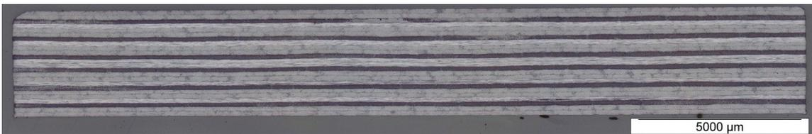
Figure 4.9 Photomicrograph of polished cross-section of open-hole compression specimen without interlaminar defects
