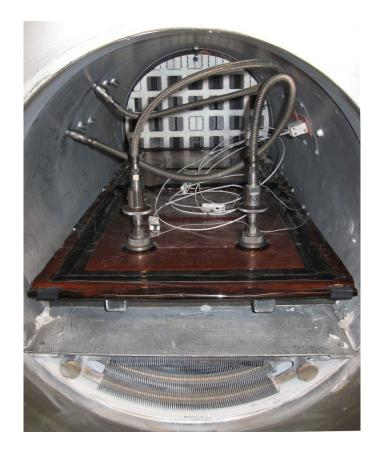
Figure 4.7 Illustration of vacuum bagged laminate in high-temperature autoclave
