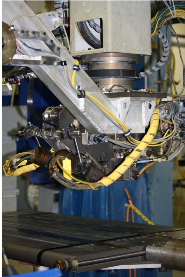
Figure 6.3 Dual-torch automated fiber placement system (photo courtesy of Automated Dynamics)
