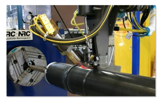
Figure 5.2 6-axis gantry-type fiber placement system equipped with the thermoplastic fiber placing head (photo courtesy of the National Research Council Canada)
