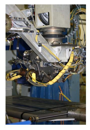
Figure 6.3 Dual-torch automated fiber placement system (photo courtesy of Automated
