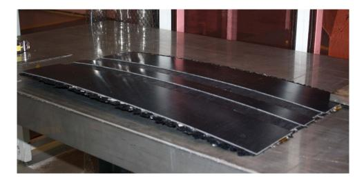
Figure 6.8 Illustration of warped test panel after fiber placement
