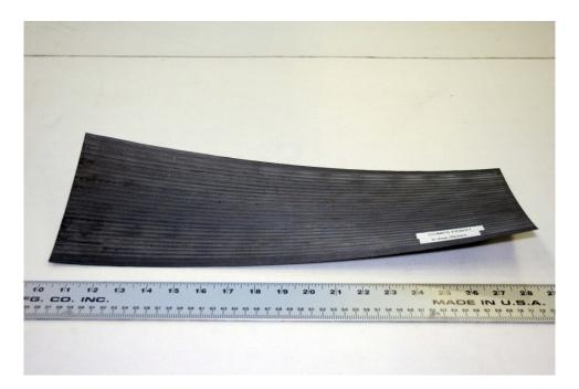
Figure 4.13 Illustration of warped fiber placed unidirectional laminate
