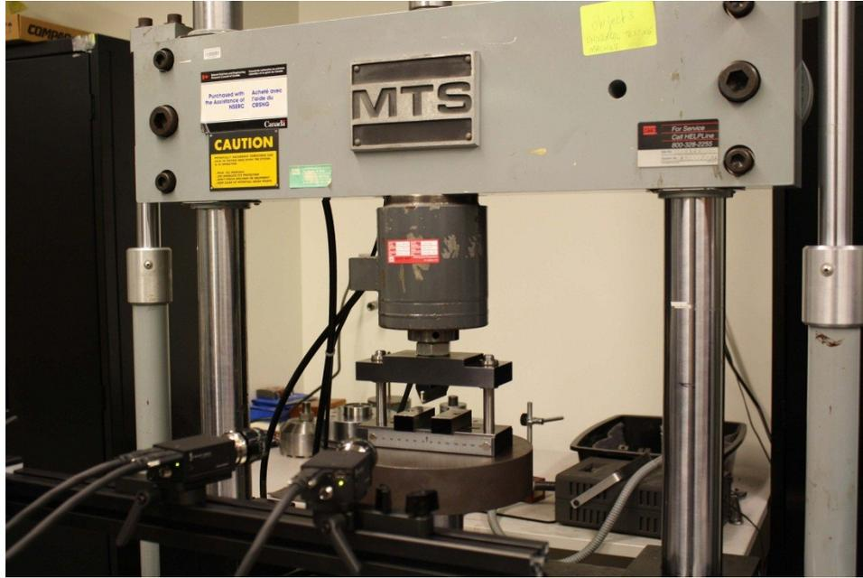
Figure 5.6 Test setup for 3D image correlation measurements
