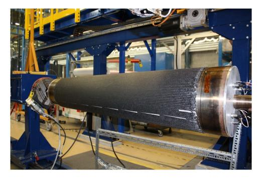
Figure 3.1 Illustration of gaps highlighted in white between two sections on a 0° ply (photo courtesy of the National Research Council Canada)
