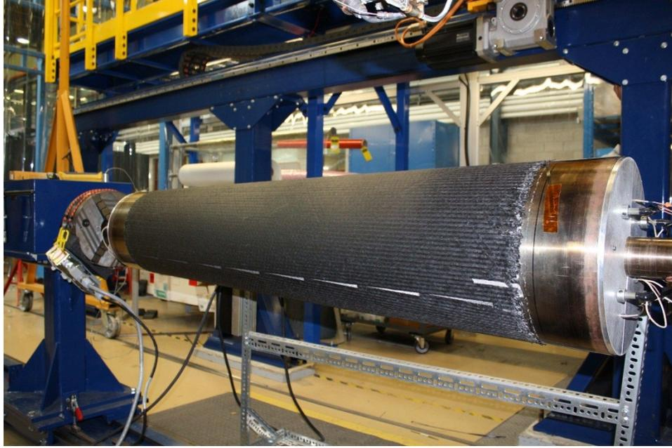
Figure 3.1 Illustration of gaps highlighted in white between two sections on a  $0^\circ$  ply
