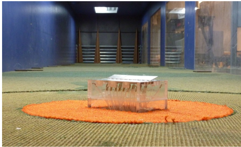
Figure 4.4.6 View of building model with panels placed on the turntable at 135^\circ wind direction
