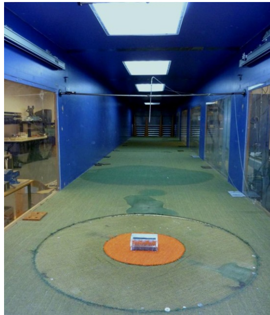
Figure 4.2.2 Front View of the Boundary Layer Wind Tunnel with the building model in position
