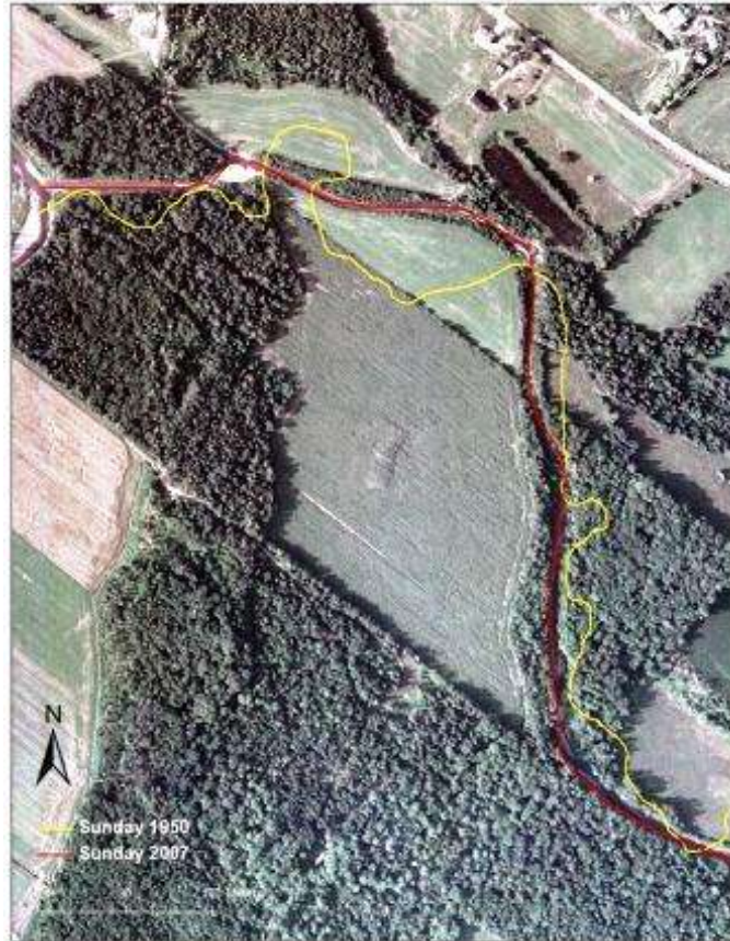
Figure 5.3 Channel paths in 1950 and 2007 overlaid on a satellite image from 2007. The channel has been displaced up to 100 meters in the downstream most reach.
