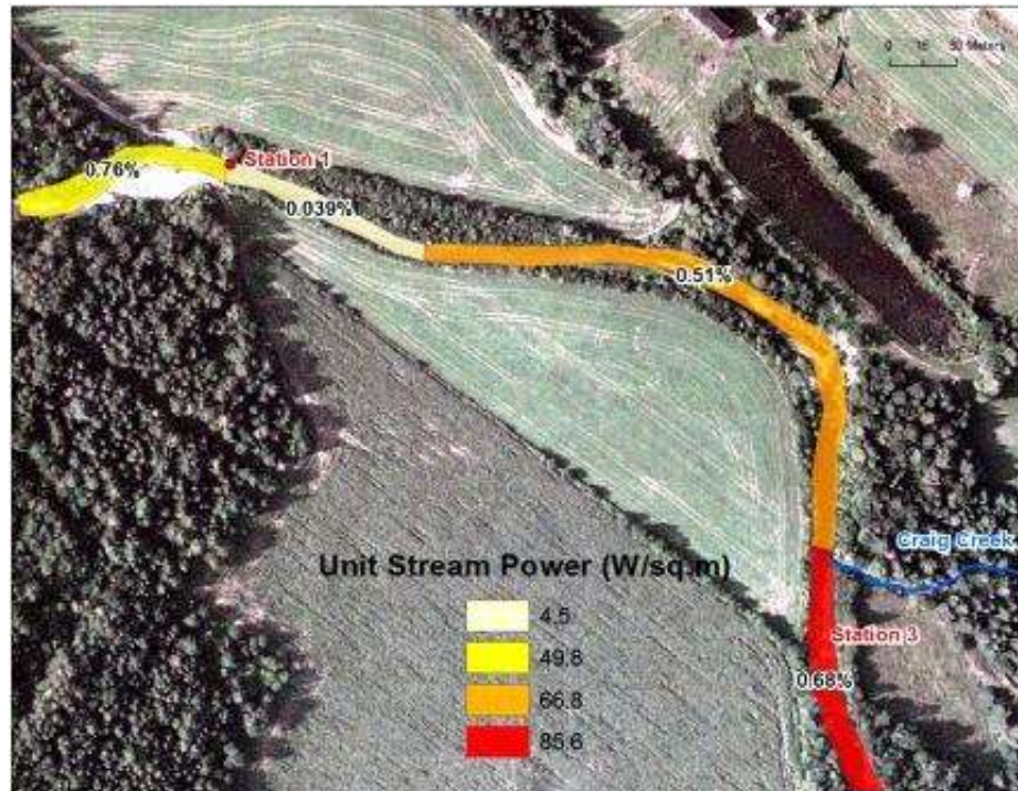
Figure 5.13 Unit stream power at bankfull stage ( 14.7 \text{ m}^3/\text{s} ) in the study reach, calculated using zone averaged width and water surface slope (indicated for each zone).
