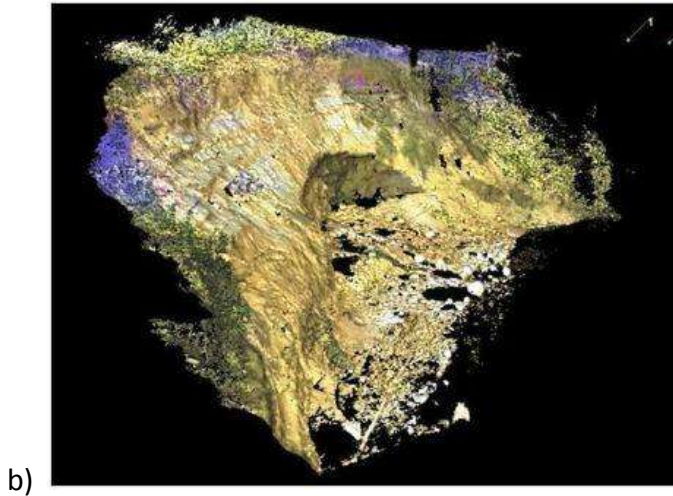
Figure 5.16 Side view of the lidar generated point cloud in a) 2009 and b) 2010 of the bank in Figure 5.15 with vegetation removed, looking upstream from the right bank.
