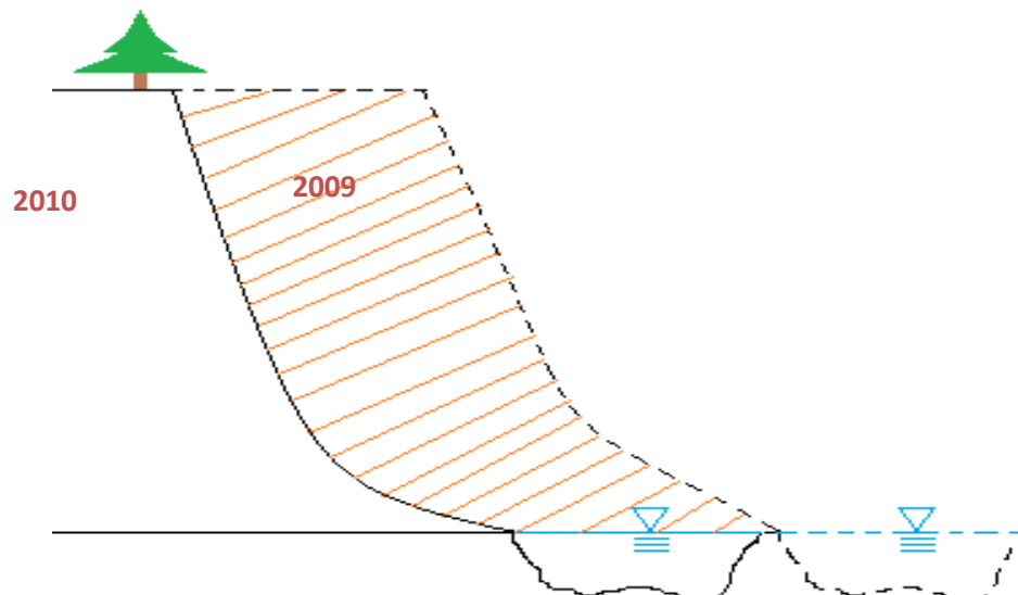
Figure 5.17 Schematic representation of the bank regression for the bank shown in Figure 5.15.
