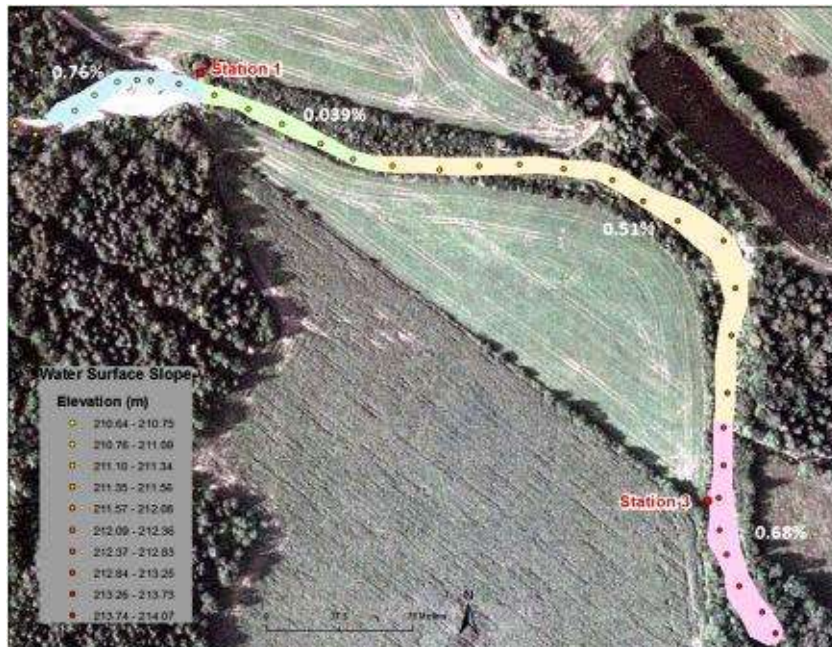
Figure 5.7 Study reach with water surface elevation points measured November 7 th 2010 (which corresponds to the medium discharge) for the four slope zones (see Figure 5.6).
