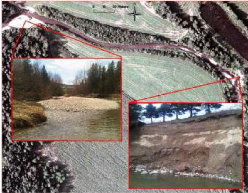
Figure 4.2 Problematic mid-channel bar and eroding bank, downstream Sunday River
