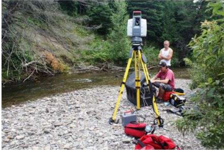
Figure 4.10 Leica Scan Station 2 in operation on the Sunday River.
