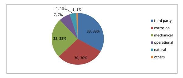
Figure 2-2 Percentages of Oïl Pipeline Failure Causes (Davis, et al., 2010)
