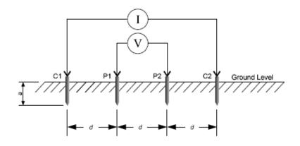
Figure 0-6 Wenner 4 Pin Test test (Lightning and Surge Technologies)
