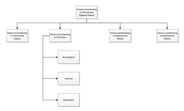
Figure 2-3 Types of factors Contributing to Pipeline Failure (Muhlbauer, 2004)
