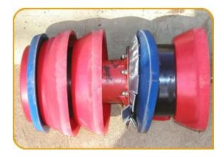
Figure 0-9 A Gauging Pig After An Internal Run (Pig Tek Limited, 2010)
