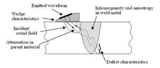
Figure 0-7 The Ultrasonic Technique (Komura, et al., 2009)
