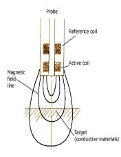
Figure 0-8 Eddy Current Technique (Efunda, 2011)
