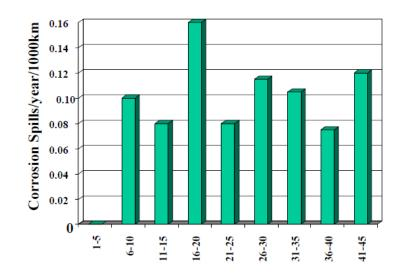
Figure 2-4 Age of Pipeline at Time of Spill (Henderson, et al., 2001)
