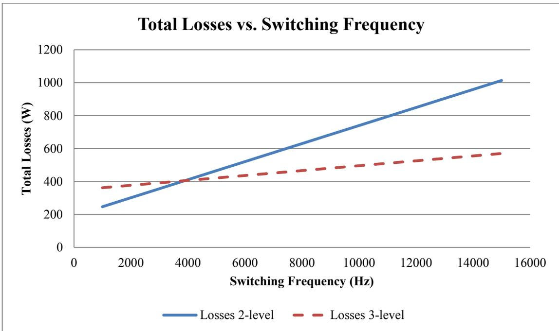
Figure 3.19: Total Losses as a Function of Switching Frequency for Two- and Three-level Inverters for a Torque of 127 Nm and a Speed of 7500 RPM
