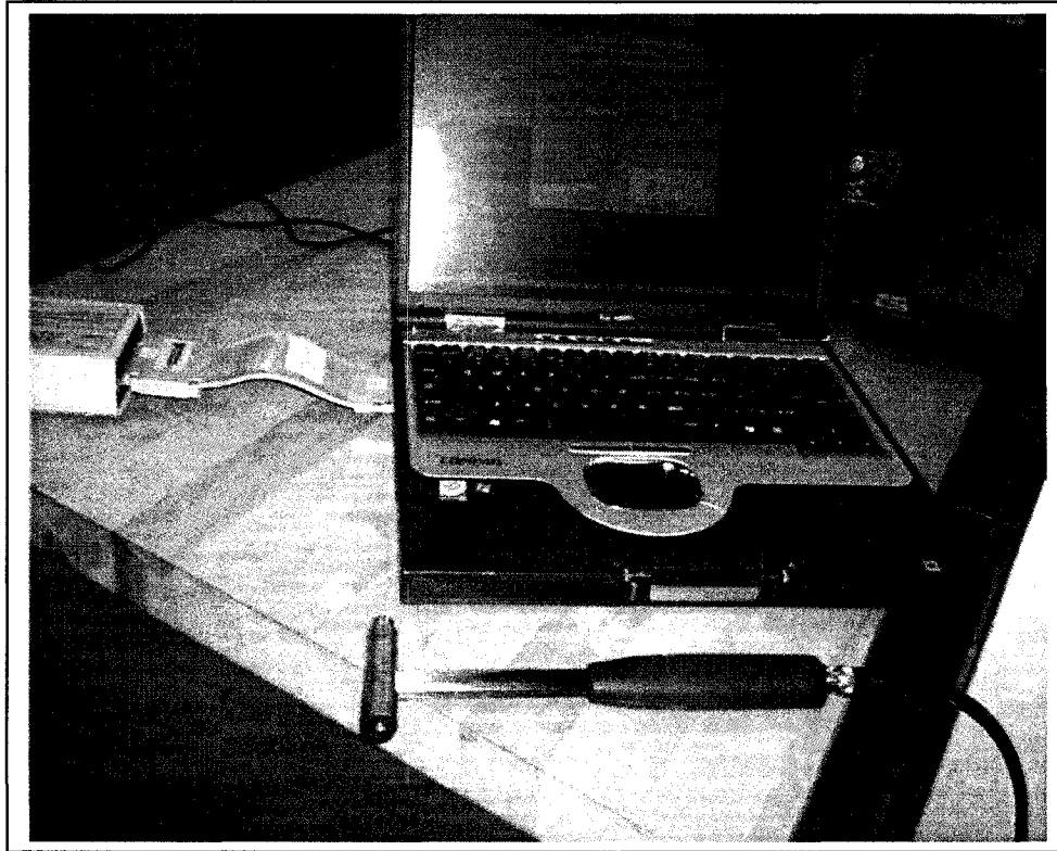
Figure 6.7: Hammer with Data acquisition system
