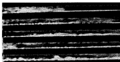
Annular flow pattern ( x = 0.0371 ) (Liquid from the top-wall)
