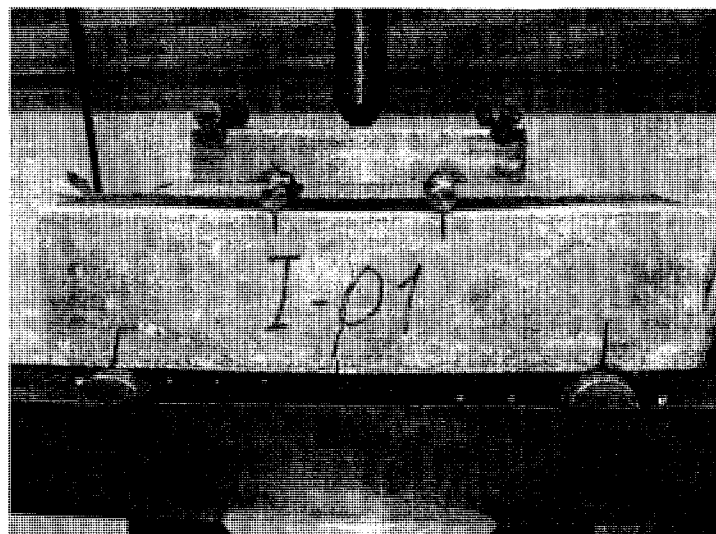
Figure 3.5—Image from the Set-up of Specimens for Flexural Test, Third-Point Loading.
