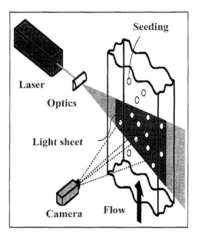
Figure 4.1. Diagrammatic view of principle of operation of PIV technique (Software user's guide; Dantec Dynamics, 2000).
