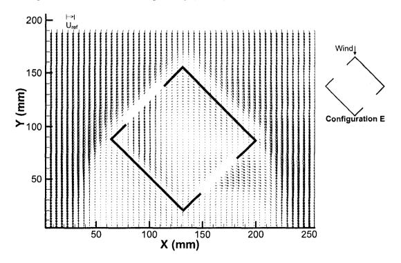
Figure 4.22. Plan view of mean velocity vector field at opening mid-height for configuration E with 10% wall porosity ( $\theta = 45^{\circ}$ ).
