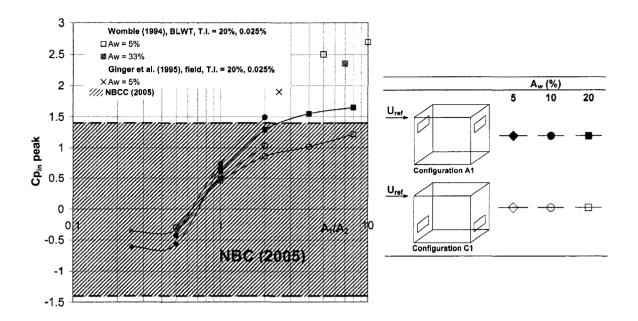
Figure 5.22. Peak internal pressure coefficients for configurations A1 and C1 with  $A_w = 5\%$ , 10%, and 20%, different inlet-to-outlet ratios, and 20% blockage - comparison with previous studies and NBCC (2005).
