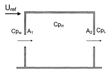
Figure 3.1. Schematic representation of wind-driven cross-ventilation.
