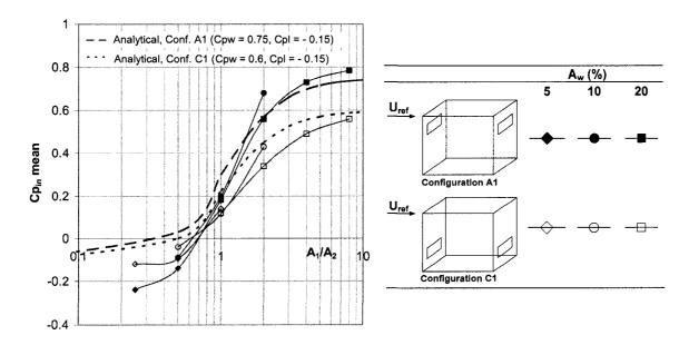
Figure 5.21. Mean internal pressure coefficients for configurations A1 and C1 with  $A_w = 5\%$ , 10%, and 20%, different inlet-to-outlet ratios, and 20% blockage – comparison with analytical results.
