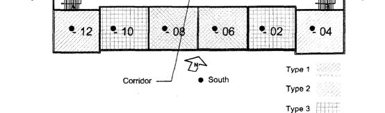
Figure 6.3. The airflow network nodes for a typical floor.
