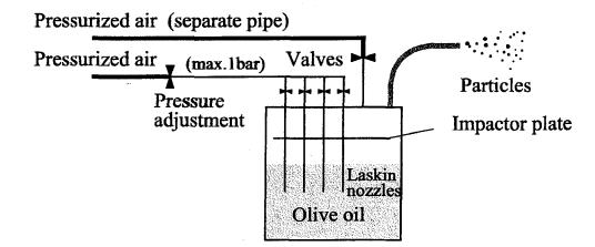
Figure 4.8. Principle of operation of seeding generator (Software user's guide; Dantec Dynamics, 2000).
