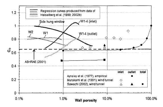
Figure 2.5. Discharge coefficients as a function of wall porosity (rectangular openings, windows).
