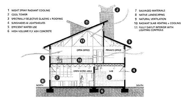
Figure 1.1. Concept of cross-ventilation system (Brager, 2006).
