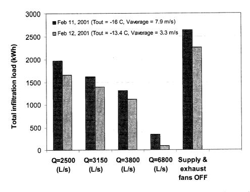
Figure 6.12. Total infiltration load (kWh) for February 11 and 12, 2001 for different ventilation scenarios and supply flow rates.
