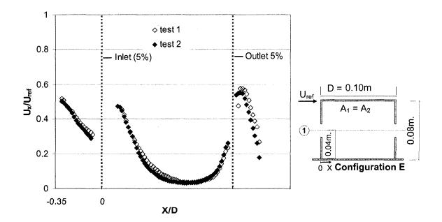
Figure 4.13. Profile of velocity component on the centre-line directly between the inlet and outlet opening (cross-section 1) based on PIV measurements on a vertical plane: Repeatability test for configuration E with 5% wall porosity.
