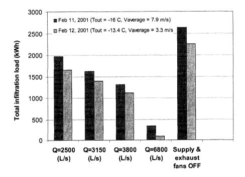
Figure 6.9. Total infiltration load (kWh) for February 12, 2001.
