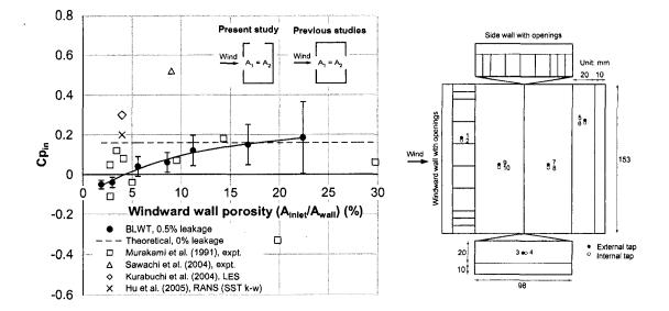
Figure 5.10. Internal pressure coefficients for cross-ventilation with  $A_1 = A_2$  and  $\theta = 0^\circ$ .
