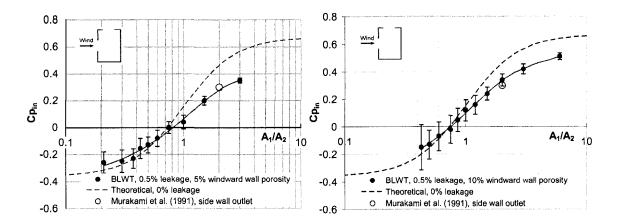
Figure 5.11. Internal pressure coefficients for cross-ventilation with different inlet-tooutlet ratios, 5% and 10% windward wall porosity.
