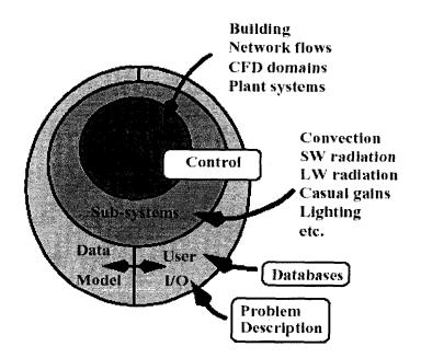
Figure 2.9. The ESP-r integrated simulator (Hensen, 1991).
