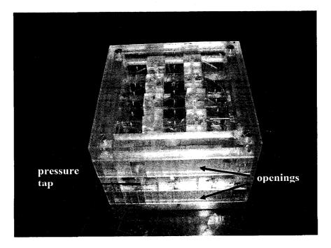
Figure 5.2. The flat roof building model.
