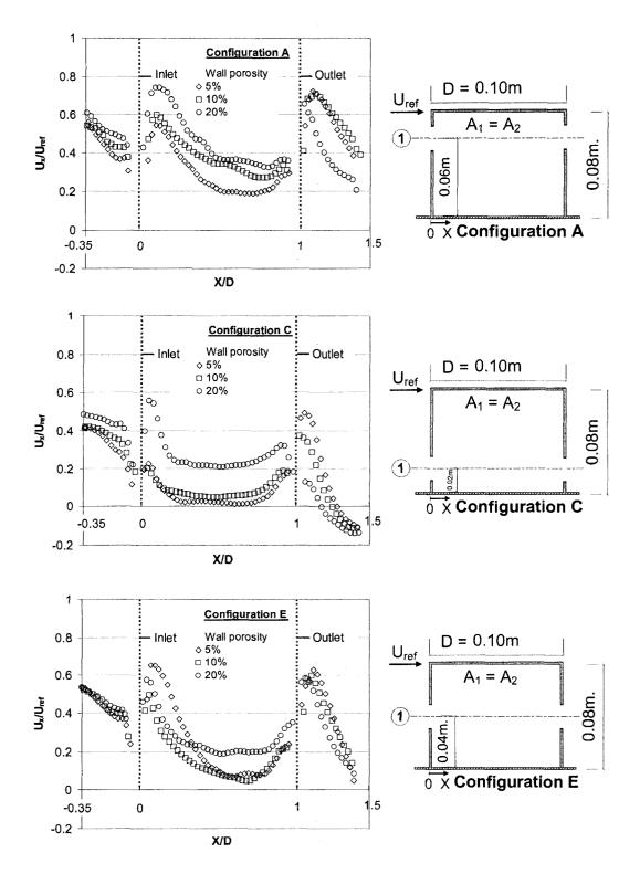
Figure 4.23. Profiles of velocity component on the centre-line directly between the inlet and outlet opening (cross-section 1) for configurations A, C, and E based on PIV measurement on a horizontal plane.
