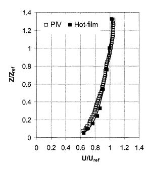
Figure 4.12. Comparison between hot-film and PIV measurements for empty tunnel velocity profiles (reference height = building height = 0.08 m).
