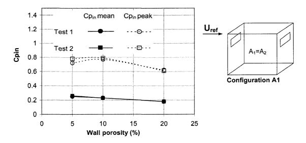
Figure 5.8. Internal pressure coefficients measured during repeatability tests.
