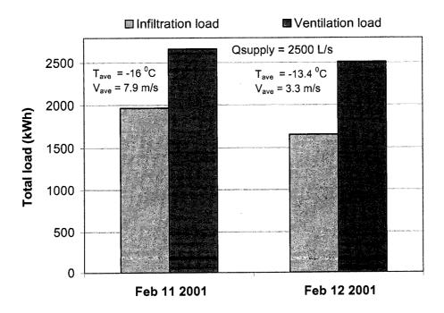
Figure 6.13. Total infiltration load and ventilation (kWh) for February 11 and 12, 2001 for Qsupply = 2500 L/s (37% of the design flow rate).
