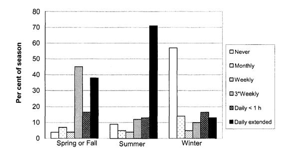
Figure 1.2. Window opening data (after CMHC, 2004).
