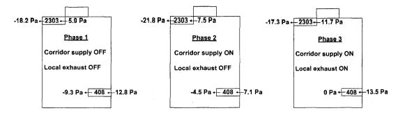
Figure 6.4. Envelope ( $\Delta P_{envelope}$ ) and corridor ( $\Delta P_{corridor}$ ) pressures for suites 408 and 2303.
