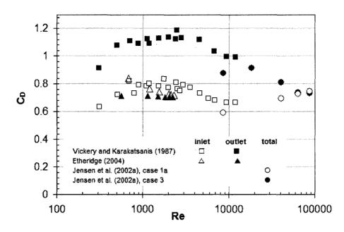
Figure 2.7. Discharge coefficients as a function of Reynolds number of the flow through the opening.
