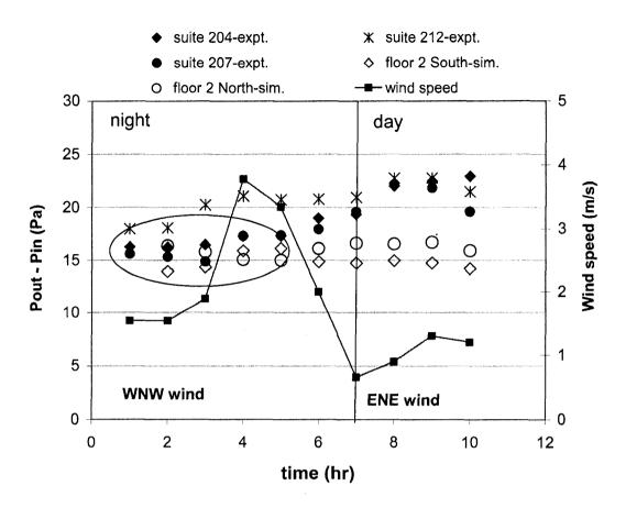
Figure 6.10. Simulation and monitoring data for the building envelope pressure below the NPL height- 2<sup>nd</sup> floor, South façade- during a cold winter day with low wind speeds (February 12, 2001).
