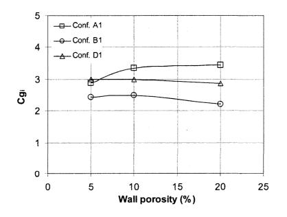
Figure 5.17. Internal gust effect factors as a function of wall porosity for configurations A1, B1, and D1 with 5% blockage.
