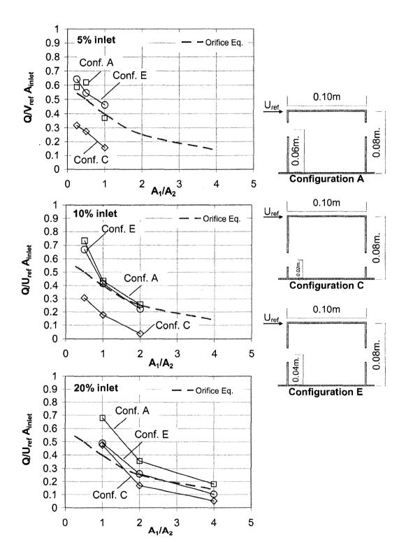
Figure 4.25. Non-dimensional airflow rate at the inlet as a function of inlet to outlet ratio for configurations A, C, and E with 5, 10, and 20 % windward wall porosity ( $\theta = 0^\circ$ ) - results based on PIV measurements on a horizontal plane.
