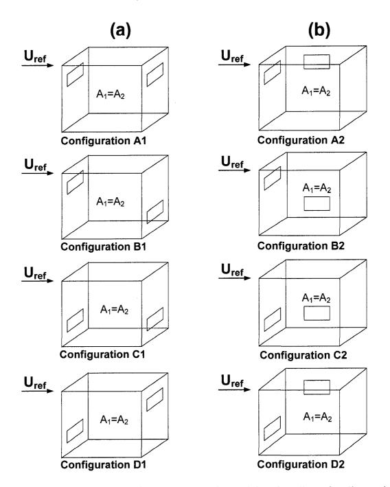
Figure 5.3. Opening configurations considered for studying the effect of wall porosity and opening location on ventilation flow rates; (a) Leeward outlet, configurations A1 and C1: symmetric openings, configurations B1 and D1: non-symmetric openings; (b) Side wall outlet, configurations A2 and C2: symmetric openings, configurations B2 and D2: non-symmetric openings.
