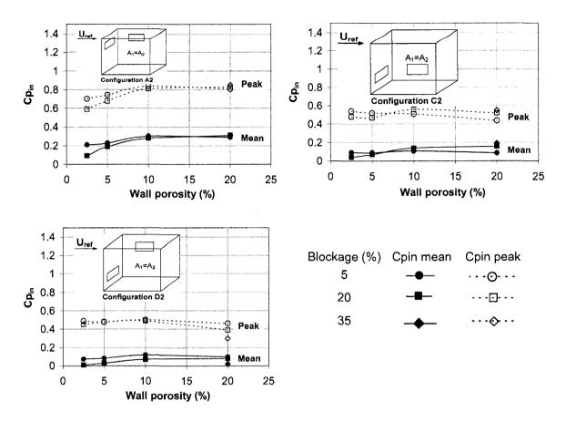
Figure 5.24. Mean and peak internal pressure coefficients for configurations A2, C2, and D2 with different blockage ratios.
