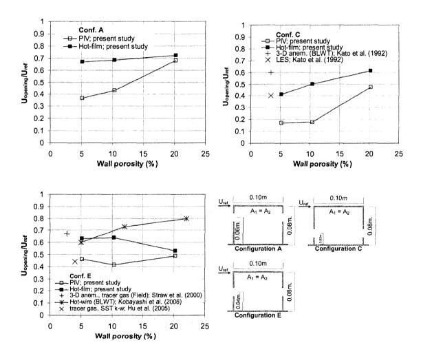
Figure 4.15. Inlet normalized velocity, measured on a horizontal plane for configurations A, B and E by using PIV and hot-film anemometry, compared with previous experimental and computational data.
