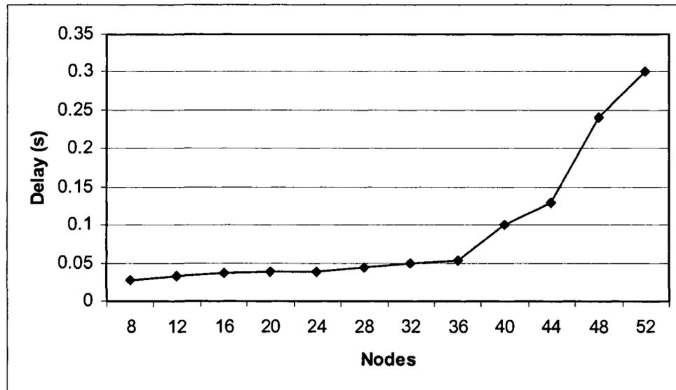
**Figure 8.4. Average delays with different number of nodes**
