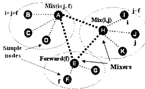
Figure 4.6. A scenario of a mixing operation
