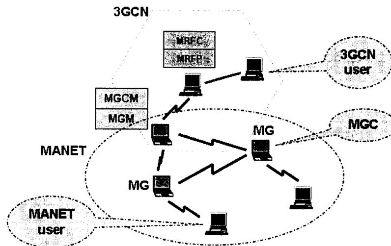
Figure 8.18. MCN test bed architecture
