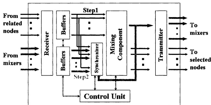
Figure 4.8. Mixer core functional architecture
