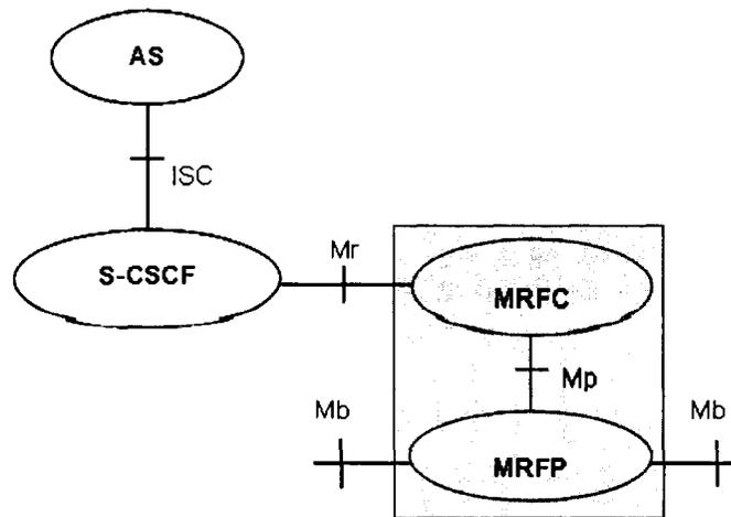
**Figure 3.6. Architecture of the MRF**
