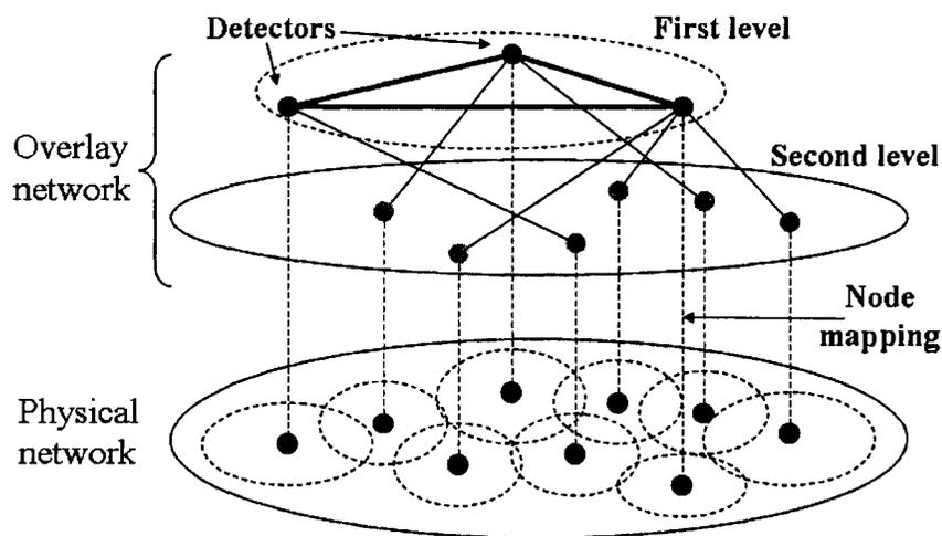
Figure 6.7. Overlay-based failure detection architecture
