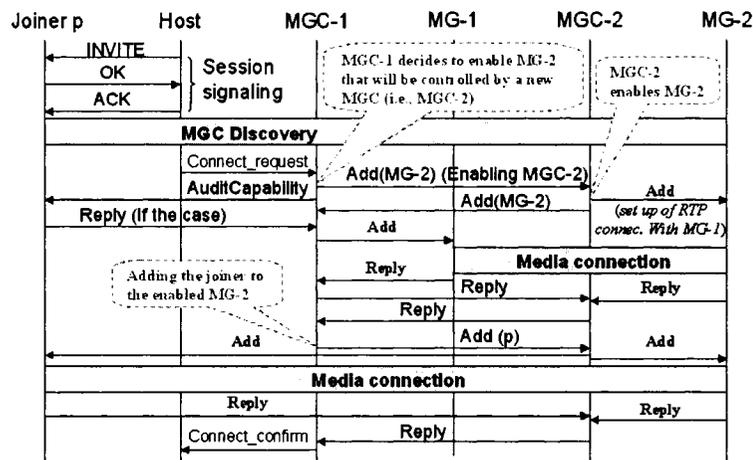
Figure 5.8. Enabling a new MGC and a new MG
