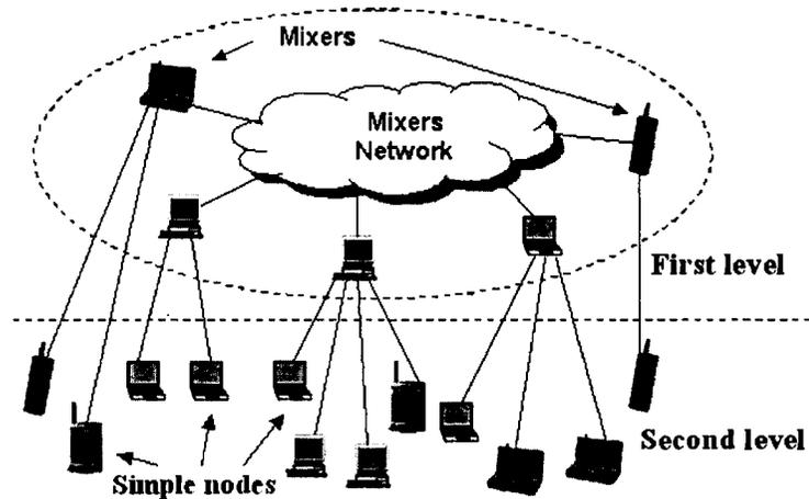
**Figure 4.5. Two-level overlay network for mixing**
