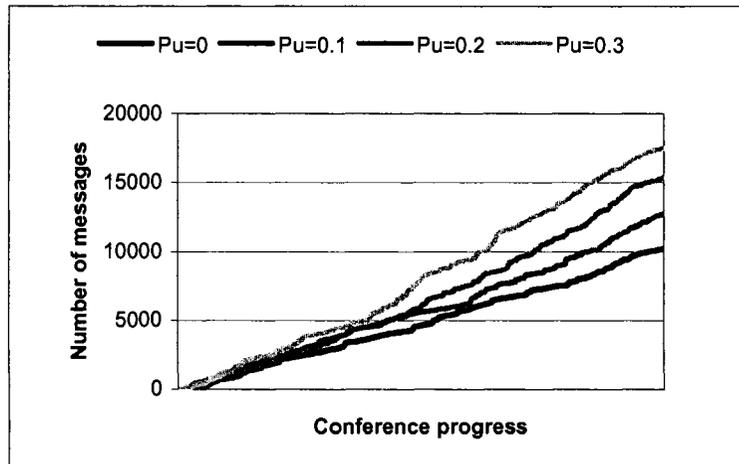
**Figure 8.8. Media signaling protocol reaction to different network situations**
