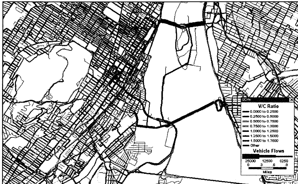
Figure 4.3 Montreal traffic assignment in 2013 with 20% intensification in subway TAZs and 40% modal shift
