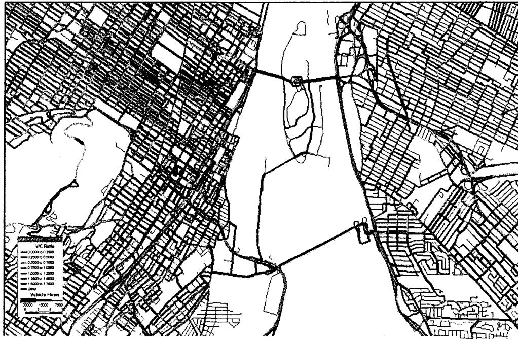
Figure 4.1 Example of the traffic assignment results for the base year 2003
