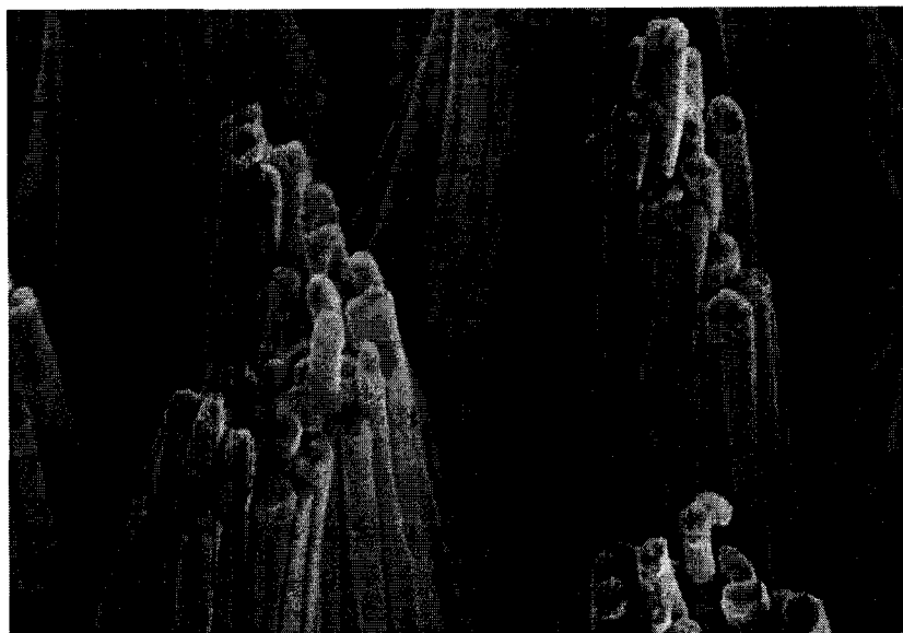
Figure 5.14. SEM micro-graph of silver- nanowires, grown by 180 minutes electrodeposition with a constant current of 1mA.
