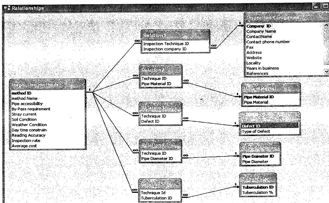
**Figure 4-5: Schema of the developed Database**
