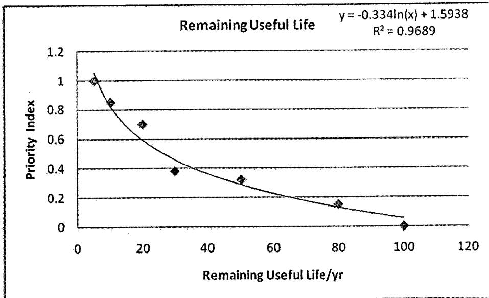
**Figure 8-4: Priority Index Function for Remaining Useful Life**
