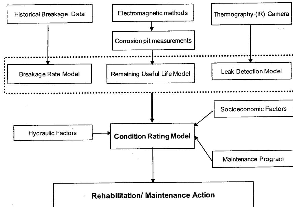
**Figure 8-1: Layout of the Developed Condition Rating Model**
