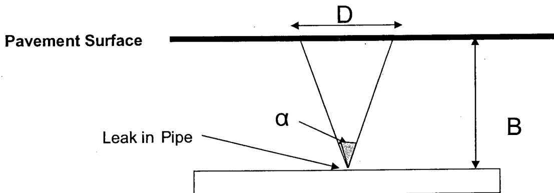
**Figure 5-12: Virtual Cone That Indicates Leak Location**
