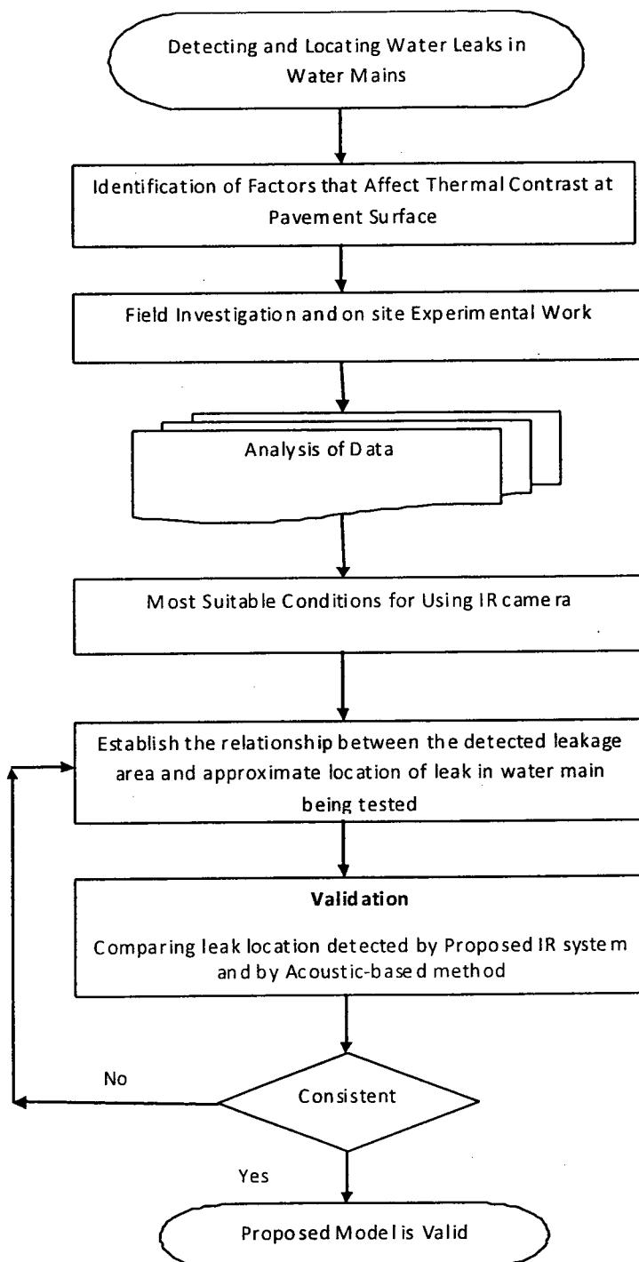
**Figure 3-4: Layout of System Development**
