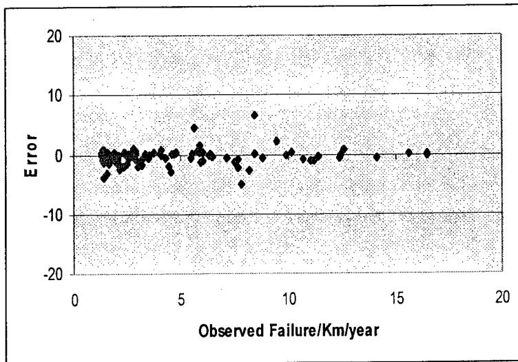
**Figure 7-5: GRNN model prediction versus observed sample**
