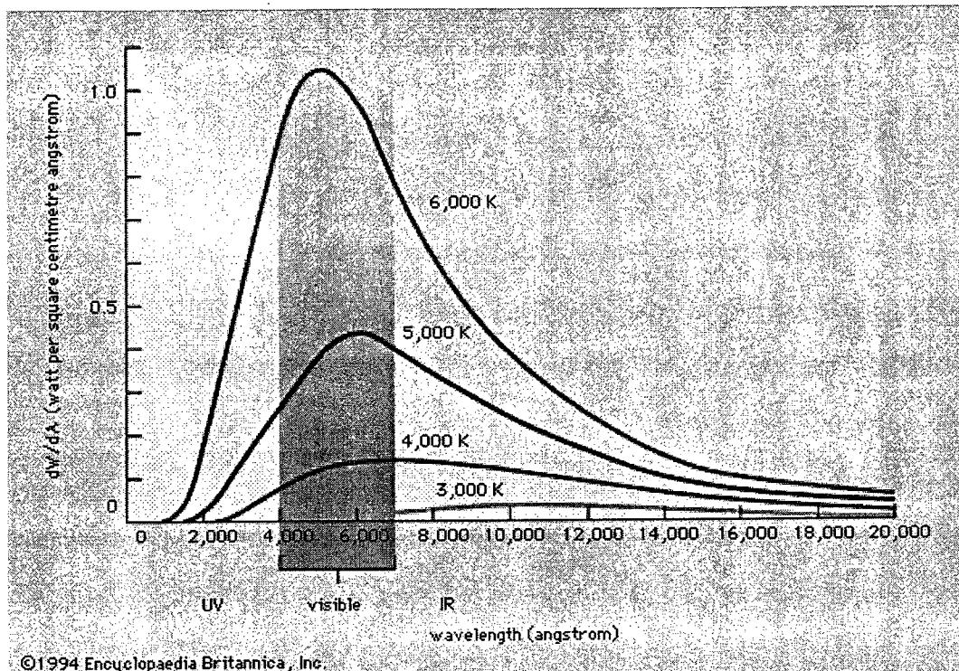
**Figure 2-5: Radiation from a Black Body at Various Temperatures**
