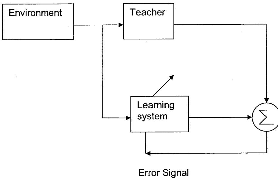
**Figure2-6: Block diagram of a learning with a teacher (supervised)**
