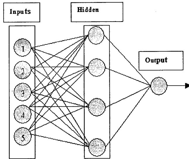
**Figure 2-7: Typical Architecture of a Back Propagation Neural Network**
