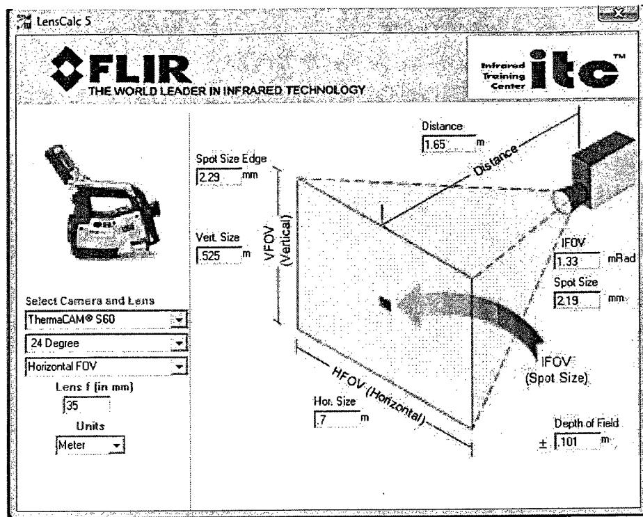
**Figure 5-9: Area Detected Using 24° Lens/ 1.65 m Distance**
