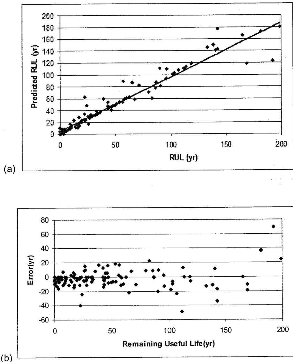
**Figure 6-7: GRNN Model Prediction Versus Observed Sample**
