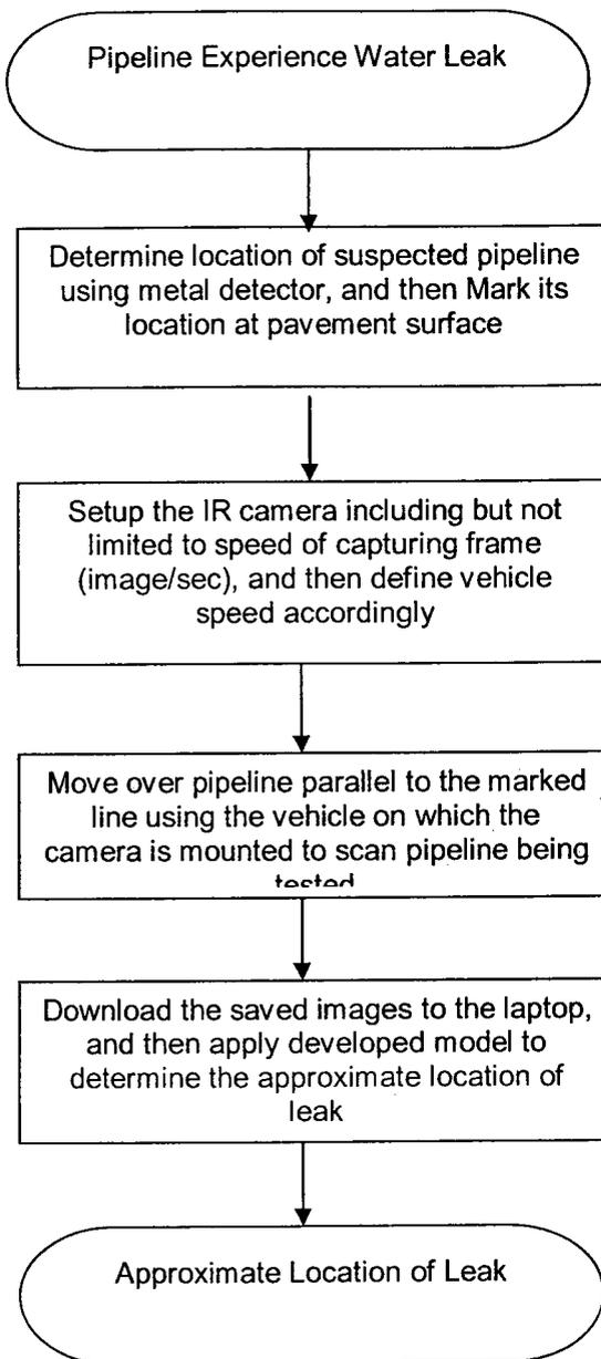
**Figure 5-15: Steps of Detecting Water Leak Using the Proposed Methodology**
