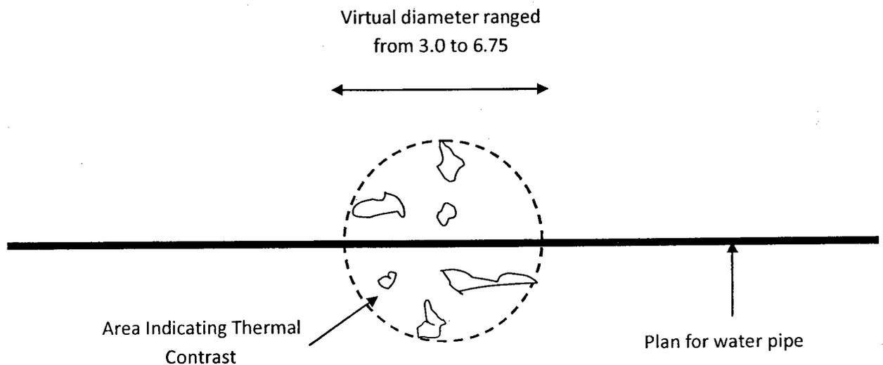
**Figure 5-8: Water Leak Indicating Thermal Contrast at Pavement Surface**
