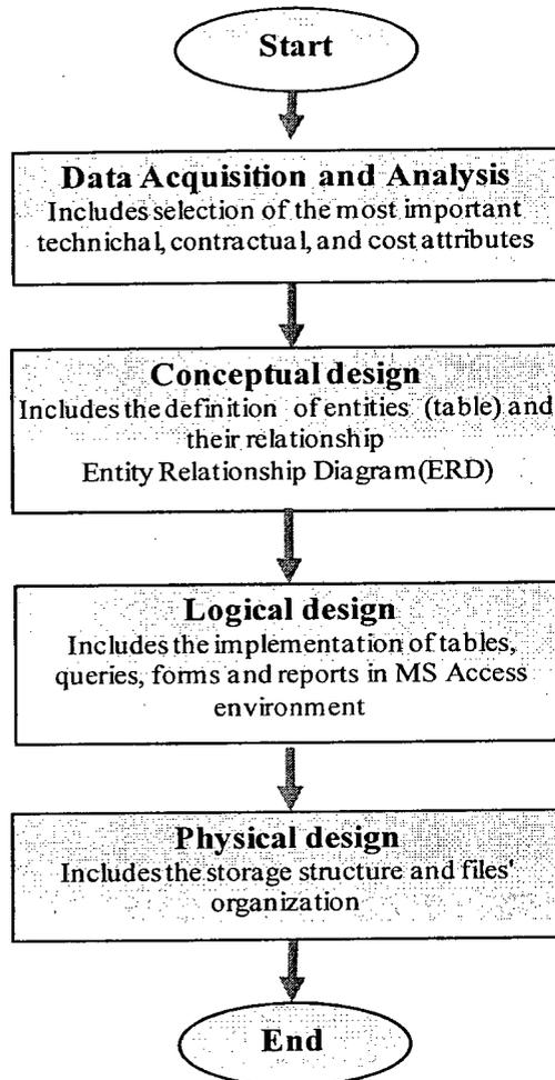
**Figure 4-2: Database Management System Design Process**
