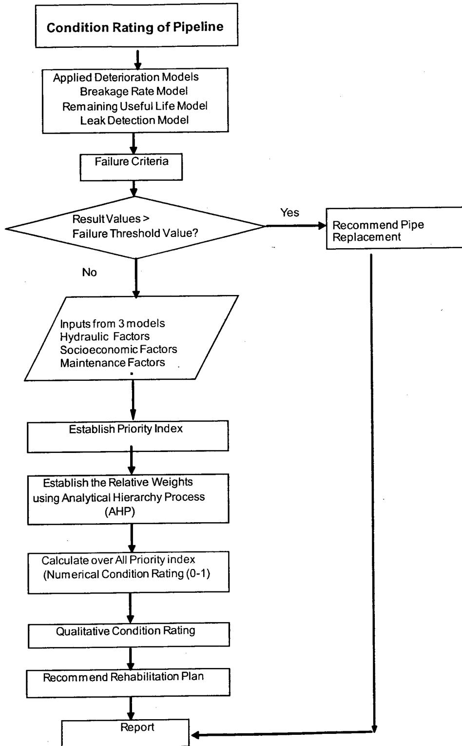
**Figure 8-3: Flow Chart for Model Methodology**
