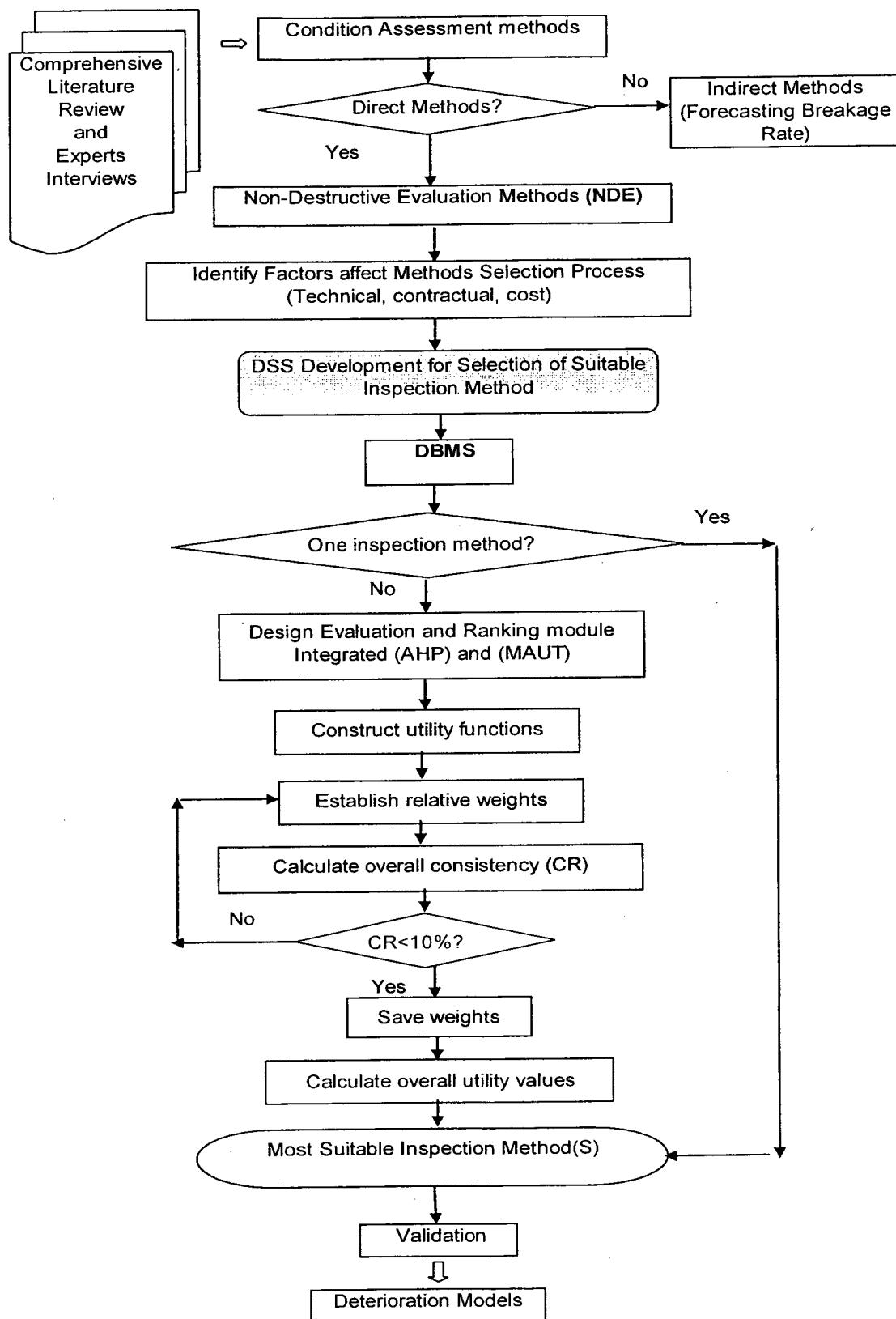
**Figure 3-3: Methodology of the Development of the DSS**
