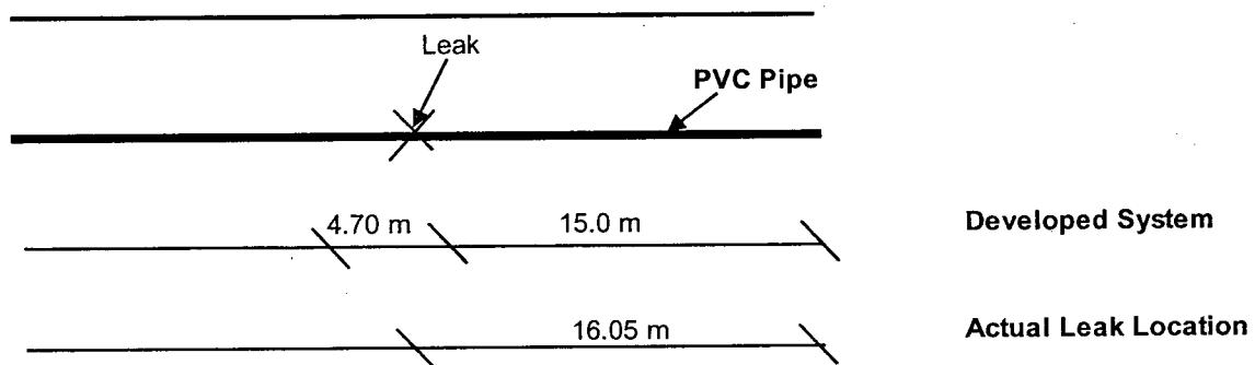
**Figure 5-11: Comparison between Leak detected Using Developed System for PVC Pipe and Actual Location of Leak**
