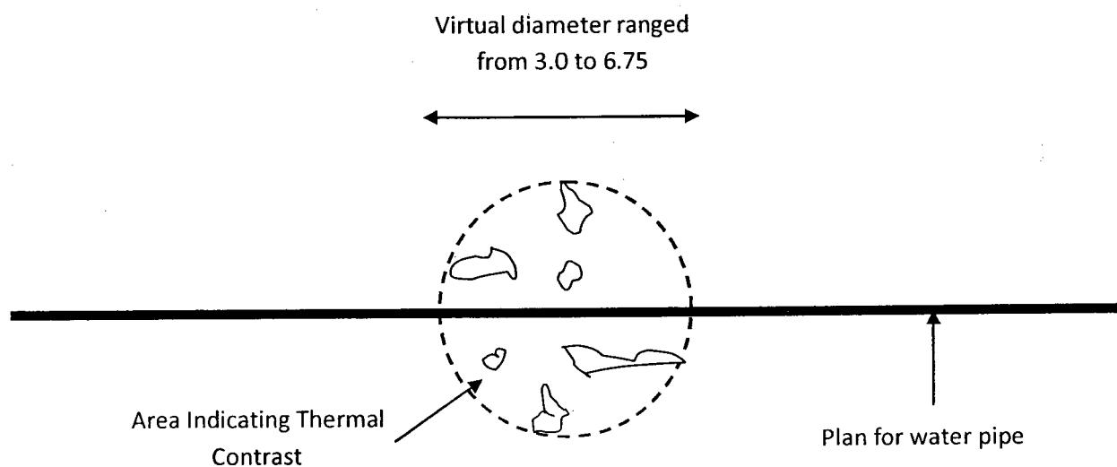
**Figure 5-8: Water Leak Indicating Thermal Contrast at Pavement Surface**
