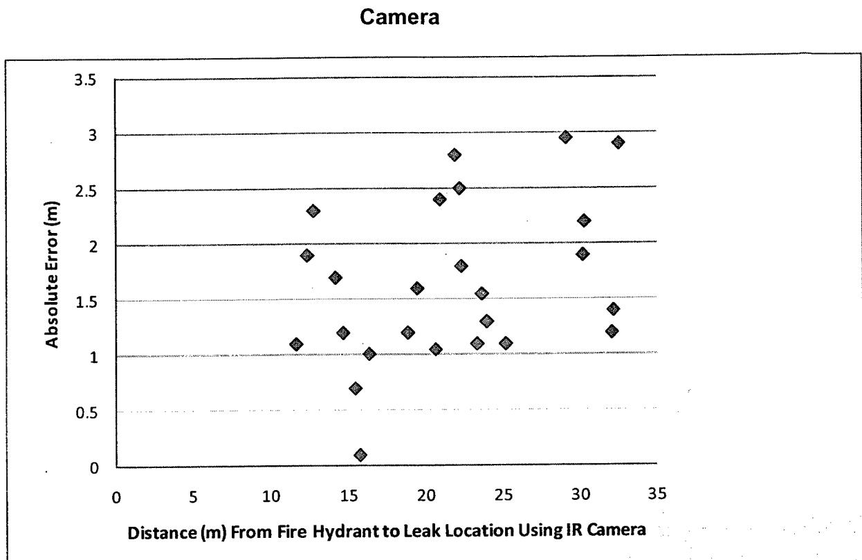
**Figure 5-14: Absolute Error (m) Using IR Camera**
