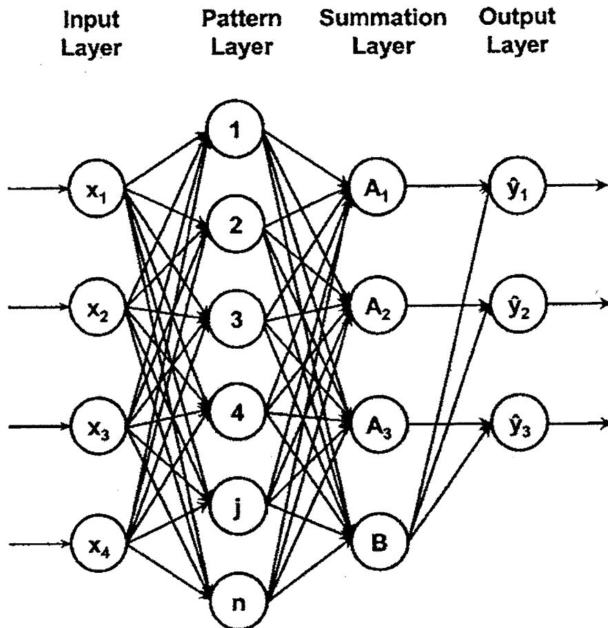
Figure 2-9: The GRNN Model Architecture
