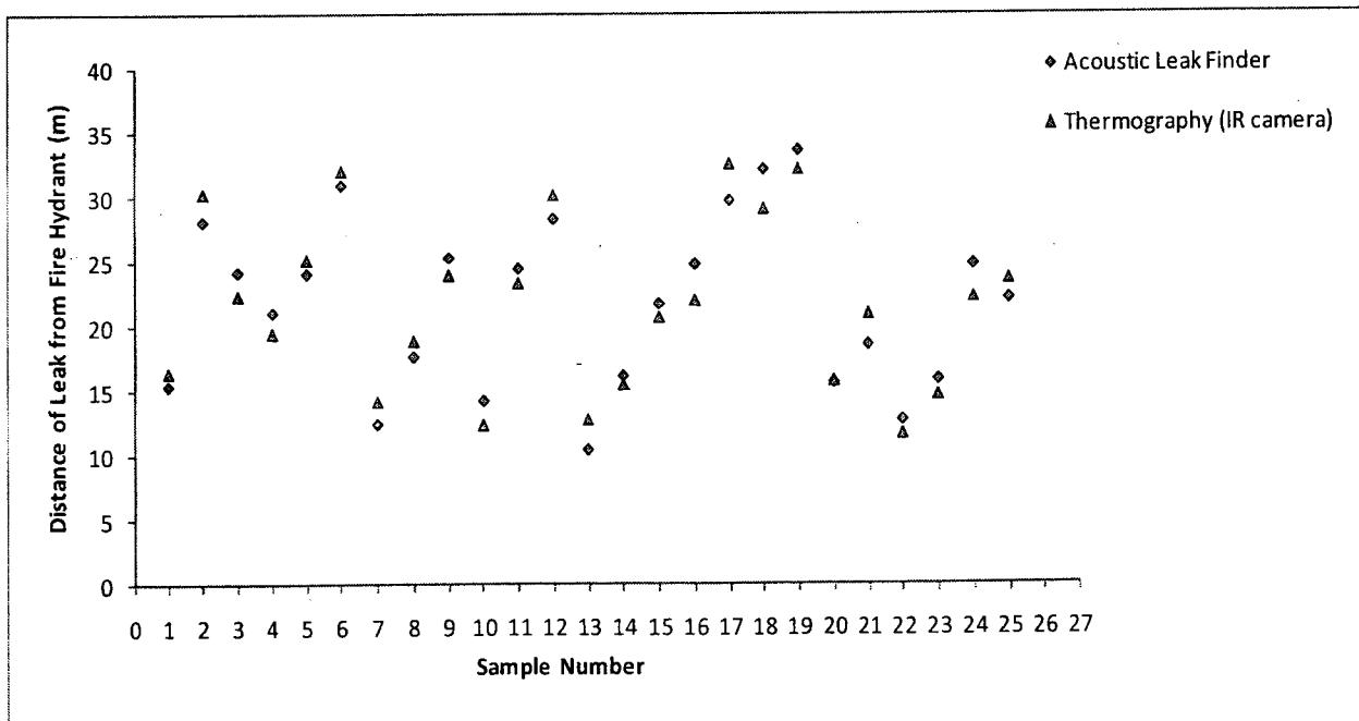
**Figure 5-13: Leak Locations (m) using Acoustic Leak Finder Verses IR**
