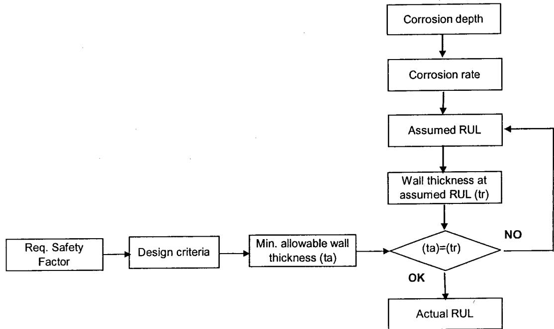
**Figure 6-2: Flow Chart for Preparation of Output Values (RUL)**
