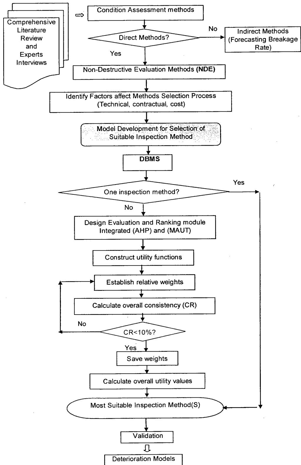
**Figure 4-1: Flow Chart for Selection of Inspection Methods**
