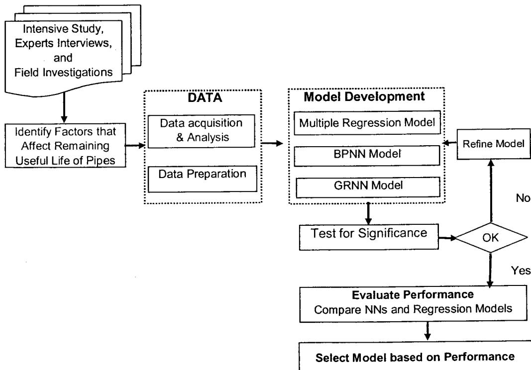
Figure 3-5: Methodology of Remaining Useful Life Model
