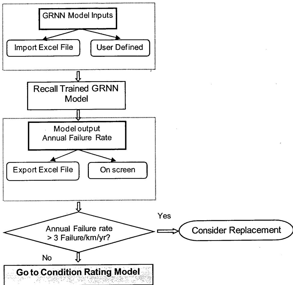
**Figure 7-7: Model Input/ Output Diagram**
