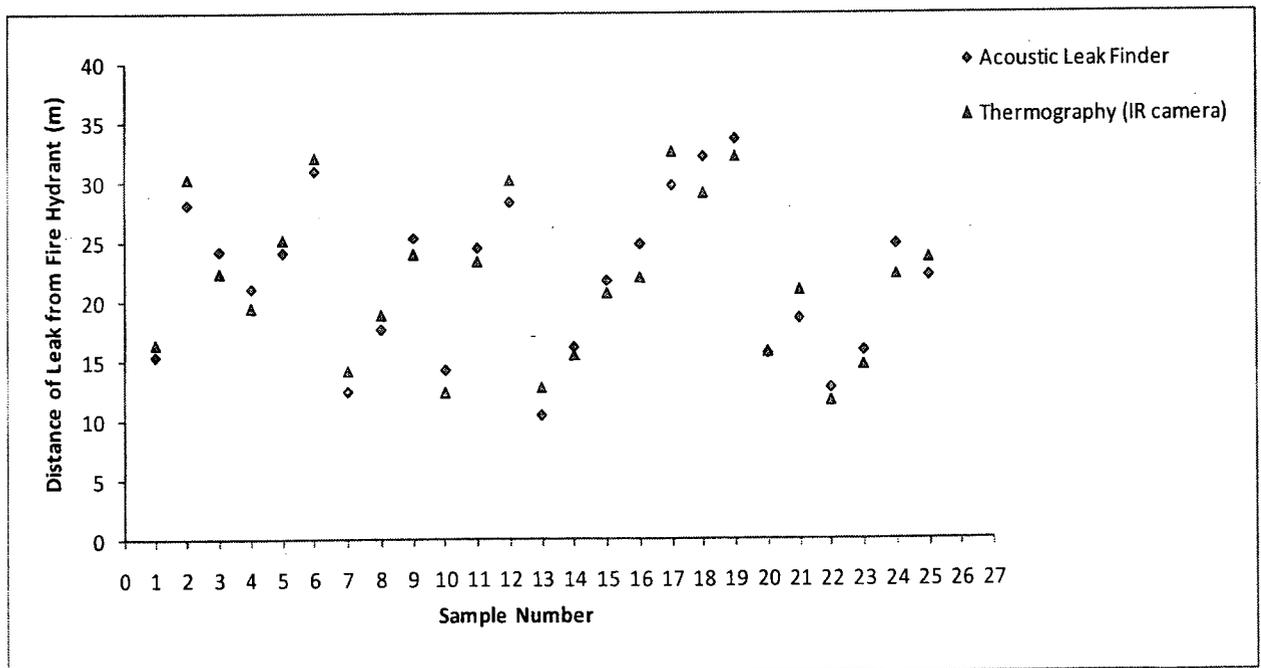
**Figure 5-13: Leak Locations (m) using Acoustic Leak Finder Verses IR Camera**
