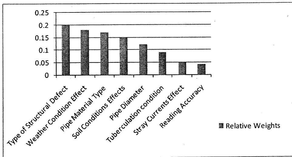
**Figure 4-11: Relative Weights for Technical Requirements**
