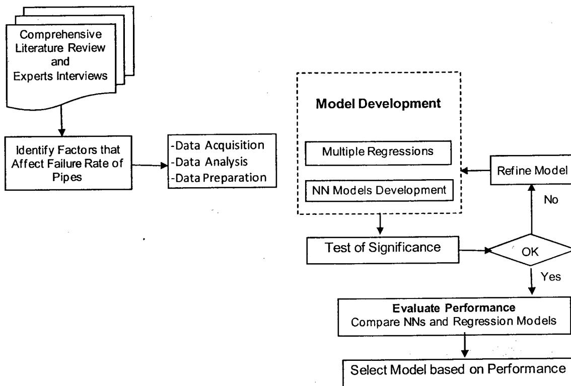
**Figure 3- 6: Methodology for Failure Rate Model Development**
