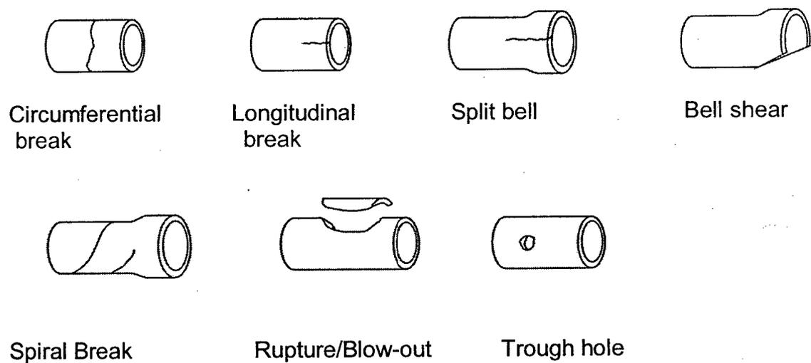
**Figure 2-1: Types of Breaks of Water Mains (National guide 2003)**
