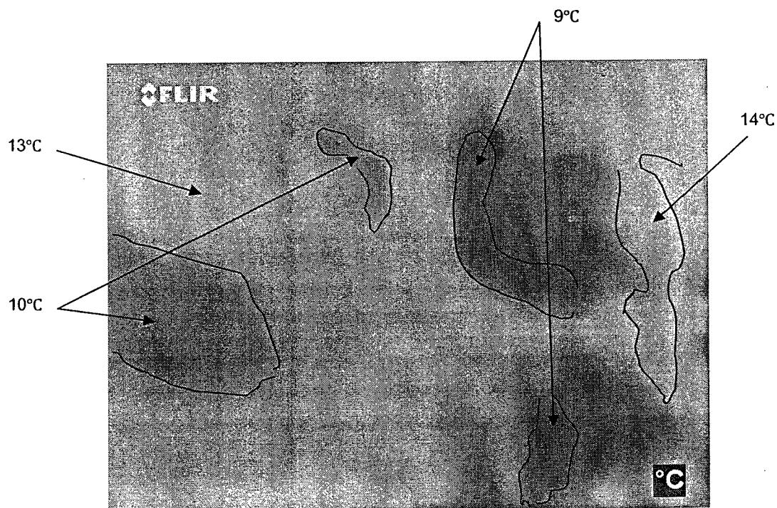
**Figure 5-7: Water Leak Detected in Fall**
