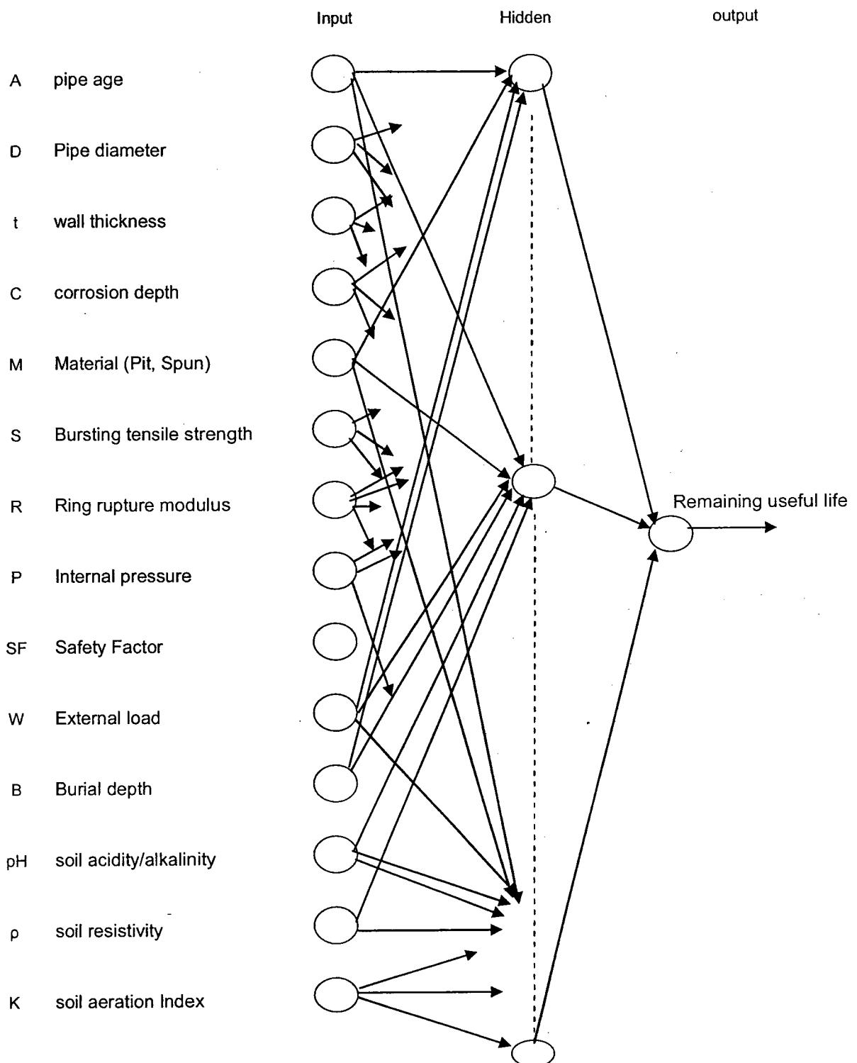
**Figure 6-4: Input/ Output Diagram for the Neural Network**
