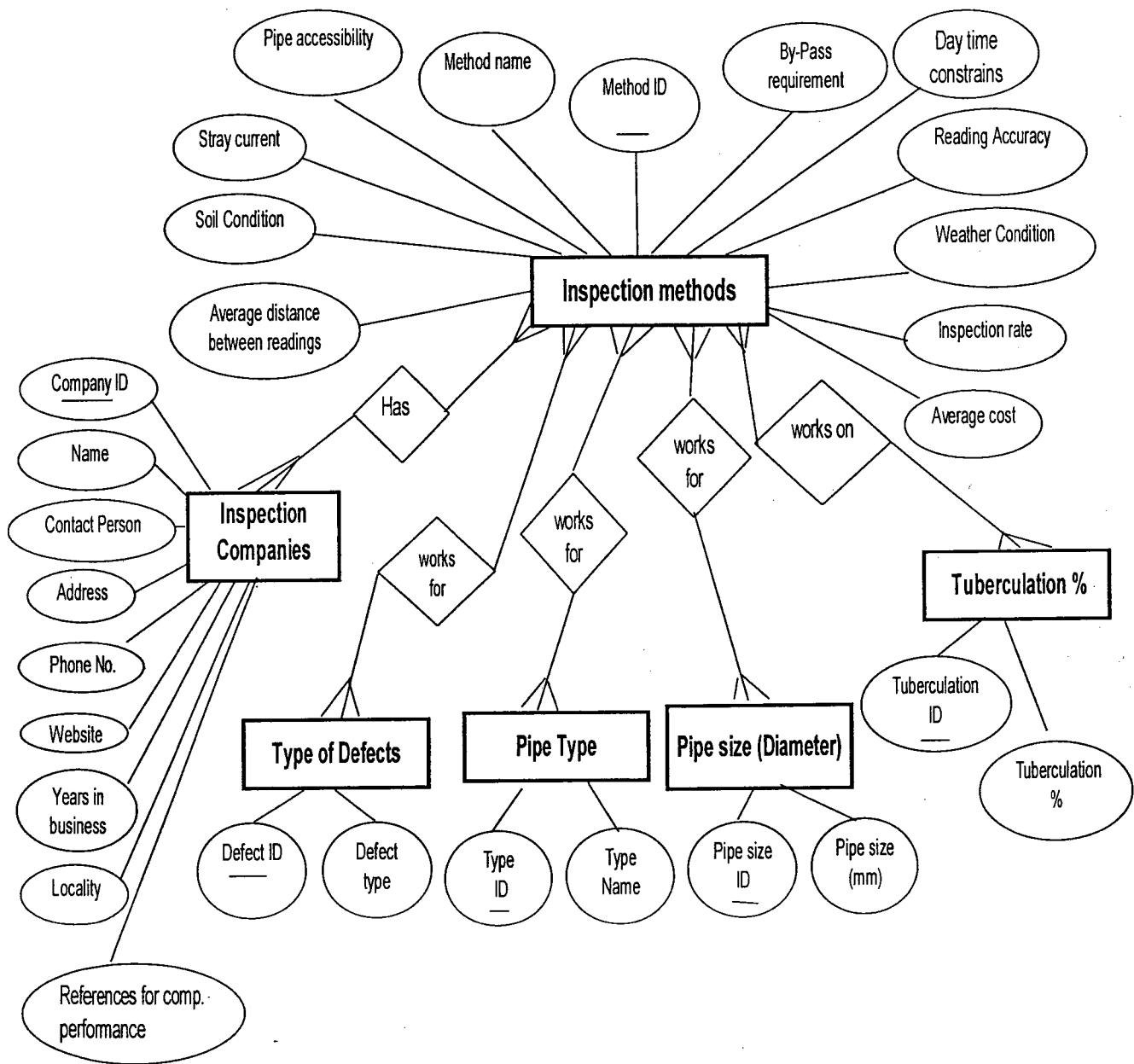
Figure 4-3: Entity Relation Diagram (ERD)
