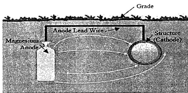
**Figure 2-11: Galvanic Anode Cathodic Protection (Waters 2001)**
