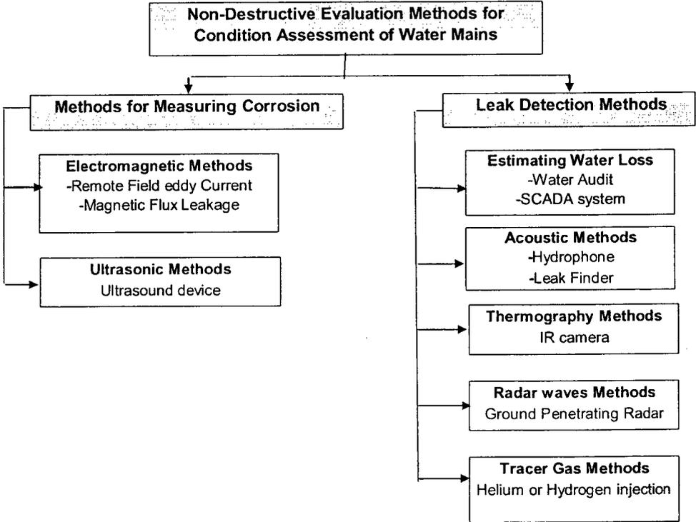
**Figure 3-2: Non-Destructive Evaluation Methods of Water Mains**
