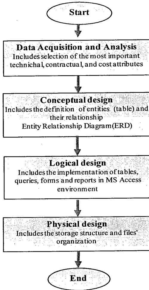
**Figure 4-2: Database Management System Design Process**
