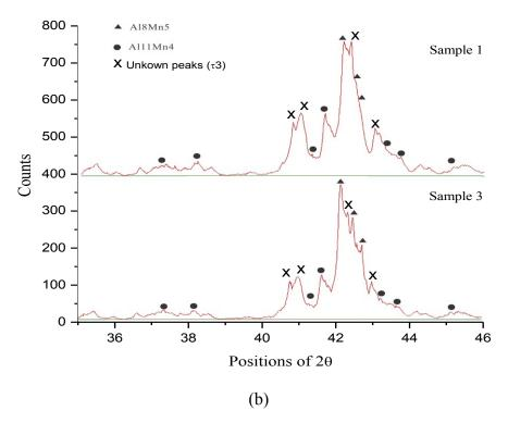
Figure 4.17: (a) Comparison of phase relations among three samples; (b) XRD comparison between samples 1 and 3.
