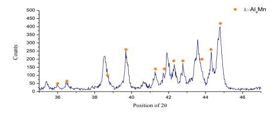
Figure 4.8: XRD pattern of post-DSC sample 1 (only Al<sub>4</sub>Mn peaks are labeled to simplify the comparison).
