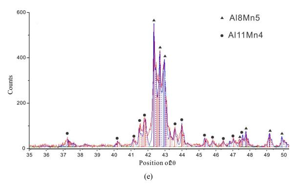
Figure 4.18: (a) BSE image of sample 1; (b) BSE image of sample 2; (c) XRD pattern of sample 1; (d) XRD pattern of sample 2; (e) XRD pattern of sample 3.
