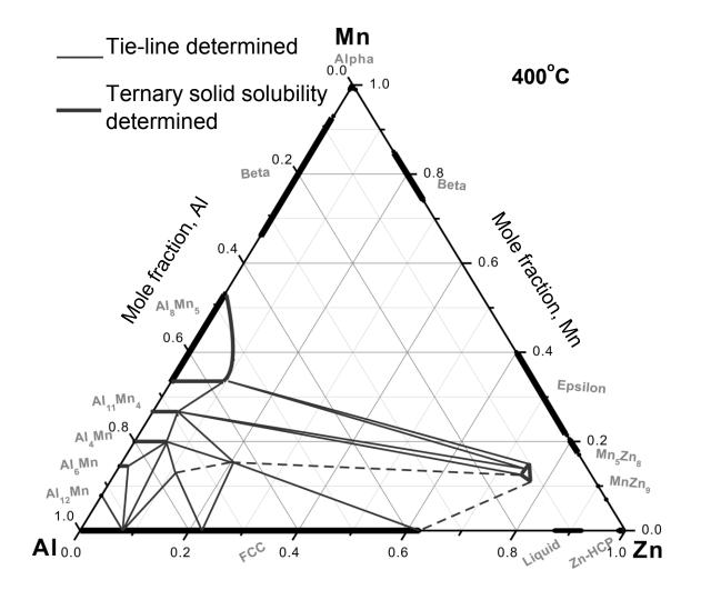
Figure 4.19: Tie lines determined by key samples technique.
