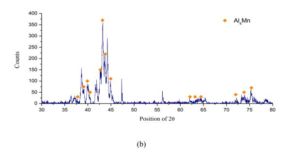
Figure 4.9: (a) XRD pattern of as-cast sample 5 (only Al<sub>4</sub>Mn peaks are labeled); (b) XRD pattern of as-cast sample 1(only Al<sub>4</sub>Mn peaks are labeled).
