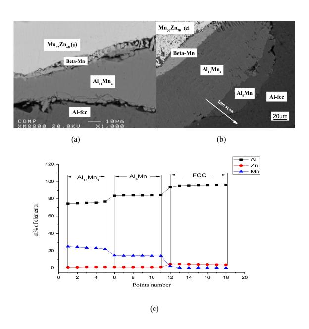
Figure 4.6: (a) BSE image of diffusion couple Al/Mn<sub>32</sub>Zn<sub>68</sub>; (b) BSE image of diffusion couple Al/Mn<sub>30</sub>Zn<sub>70</sub>; (c) composition profile of line scan in diffusion couple Al/Mn<sub>30</sub>Zn<sub>70</sub>.
