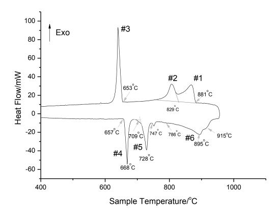
Figure 4.24: DSC spectra of sample 1.
