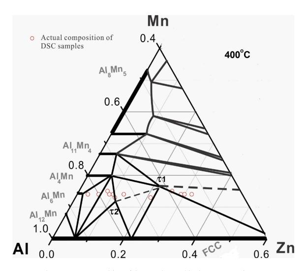
Figure 4.21: Composition of the samples used in the DSC experiments.
