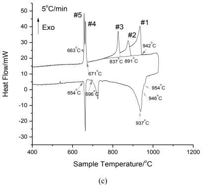
Figure 4.22: (a) DSC results of sample 6 under 15°C/min; (b) DSC results of sample 6 under 10°C/min; (c) DSC results of sample 6 under 5°C/min.
