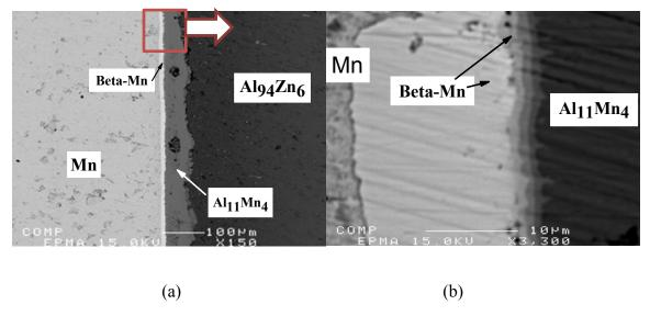
Figure 4.4: (a) BSE imagine of diffusion couple Mn/Al<sub>94</sub>Zn<sub>6</sub>; (b) magnified structure of the area of interest.
