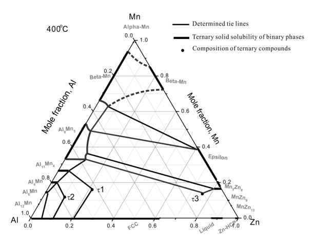
Figure 4.7: Determined phase relations of Al-Mn-Zn system obtained from diffusion couples annealed at 400°C for 4 weeks.
