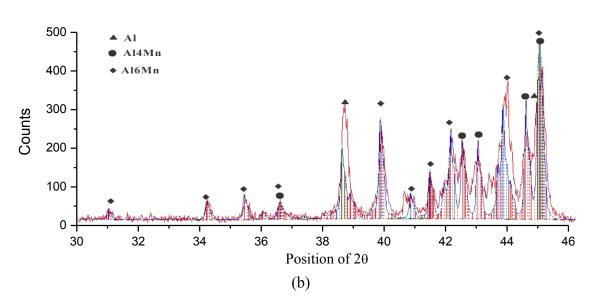
Figure 4.26: (a) XRD pattern of post DSC sample 1; (b) XRD pattern of post DSC sample 2.
