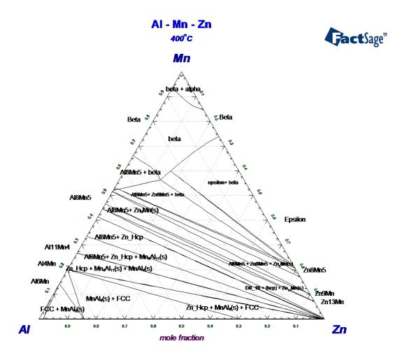
Figure 1.2: Preliminary calculation of the 400°C isothermal section of the Al-Mn-Zn ternary system.
