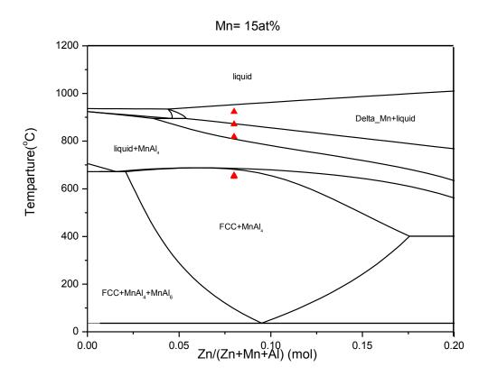
Figure 4.29: Calculated vertical section at 15 at% Mn with transformation temperature at 0°C/min cooling rate of sample 5.
