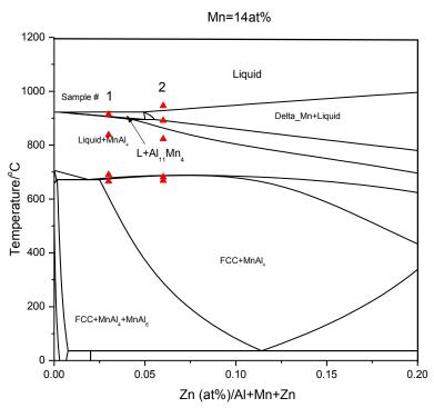
Figure 4.25: Calculated vertical section at 14 at% Mn with transformation temperature at 0°C/min cooling rate of samples 1 and 2.
