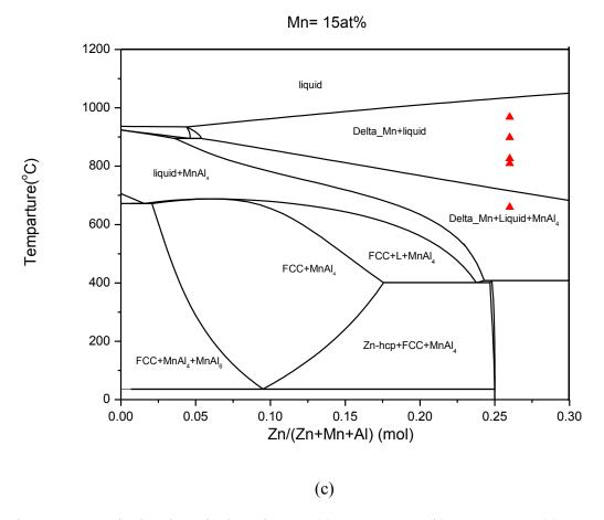
Figure 4.32: Calculated vertical sections at (a) 13 at% Mn; (b) 14 at% Mn; (c) 15 at% Mn; with transformation temperature at 0°C/min cooling rate of (a) sample 8; (b) sample 9, 10 and 11; and (c) sample 12.
