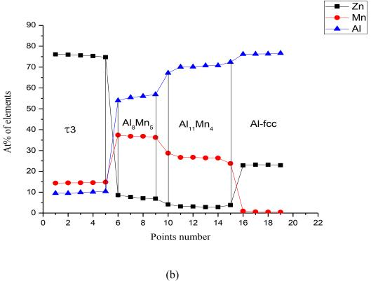
Figure 4.3: (a) Magnified microstructure of diffusion couple Al/Mn<sub>13</sub>Zn<sub>87</sub>; (b) composition profile of line scan in Al/Mn<sub>13</sub>Zn<sub>87</sub> diffusion couple.
