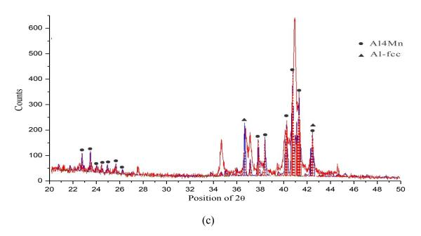
Figure 4.14: (a) XRD pattern of annealed sample 1; (b) XRD pattern of annealed sample 2; (c) XRD pattern of annealed sample 6.
