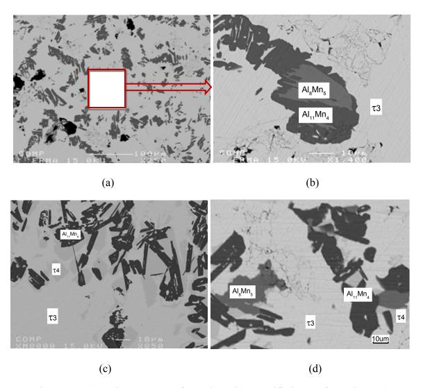
Figure 4.16: (a) Microstructure of sample 1; (b) Magnified area of sample 1; (c)
