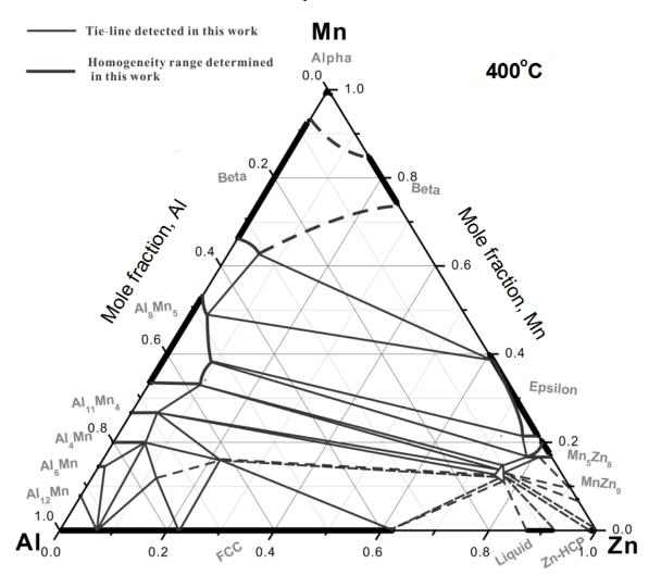
Figure 4.20: Isothermal section of Al-Mn-Zn ternary system at 400°C constructed by diffusion couples and key samples.
