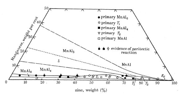
Figure 2.14: The optimized surface of primary separation by [82].
