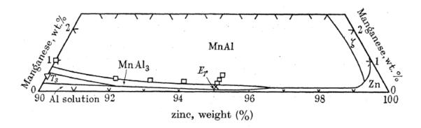
Figure 2.13: The optimized surface of primary separation by [82].
