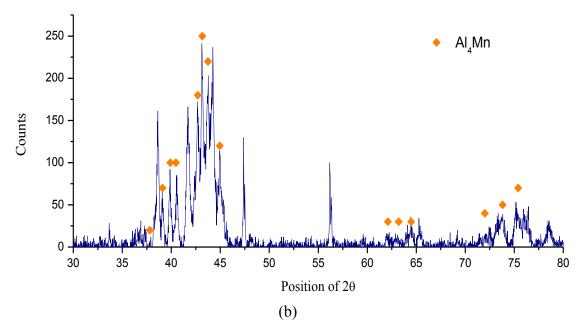
Figure 4.10: (a) XRD pattern of annealed sample 1(only Al<sub>4</sub>Mn peaks are labeled); (b) XRD pattern of annealed sample 2 (only Al<sub>4</sub>Mn peaks are labeled).
