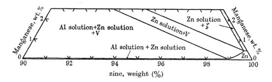
Figure 2.12: partial isothermal section at 350°C obtained by [81].
