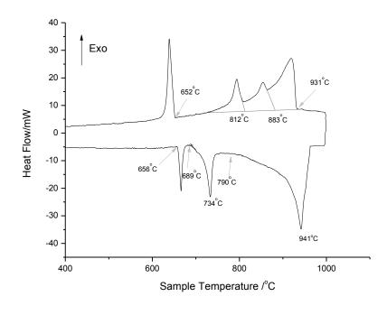
Figure 4.27: (a) DSC spectra of sample 3 at 15°C/min; (b) DSC spectra of sample 4 at 15°C/min.
