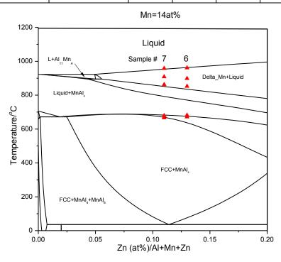
Figure 4.31: Calculated vertical section at 14 at% Mn with transformation temperature at 0°C/min cooling rate of sample 6 and 7.
