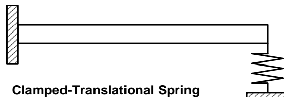
Figure 5.1: Uniform beam clamped at one end with a translational spring attached to the other end of the beam
