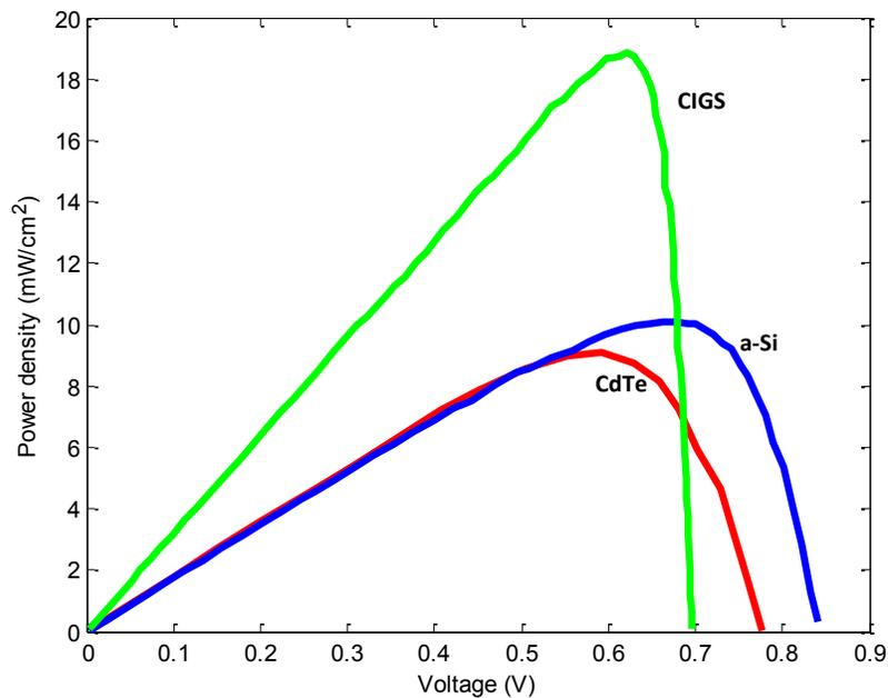
Figure 6.17: Power curves for different types of thin film solar cells
