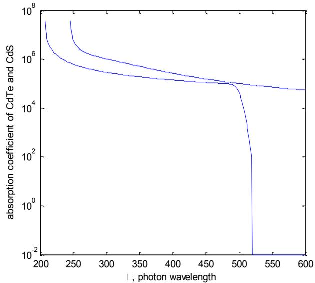
Figure 2.2: Optical absorption coefficient of the CdTe and CdS
