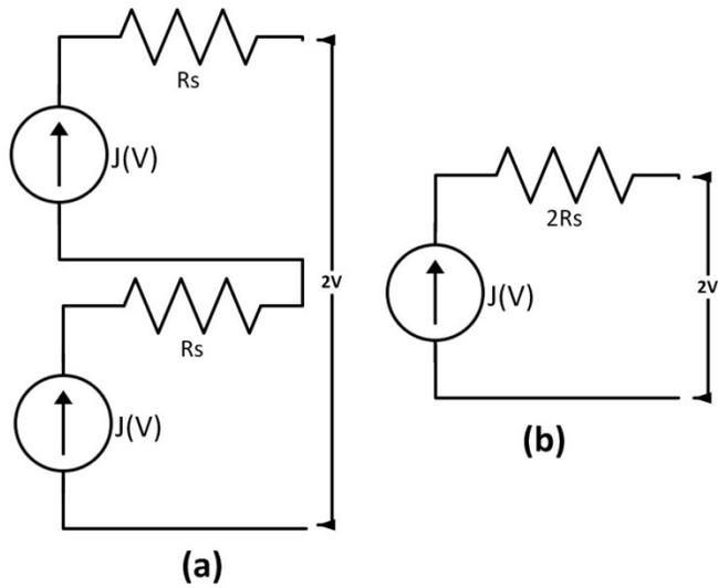
Figure 3.2: (a) 2 solar cells in series and (b) their equivalent circuit
