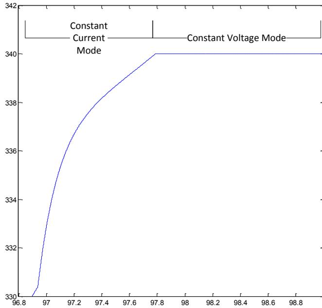
**Figure 6.12: Voltage Vs SOC (%) profile**
