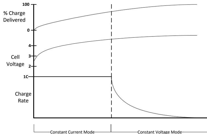
**Figure 6.10: Typical C-V Charge Profile [32]**
