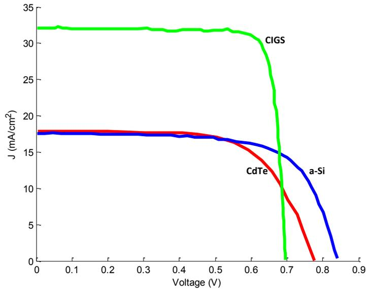
Figure 6.18: current voltage characteristics for different types of thin film solar cells
