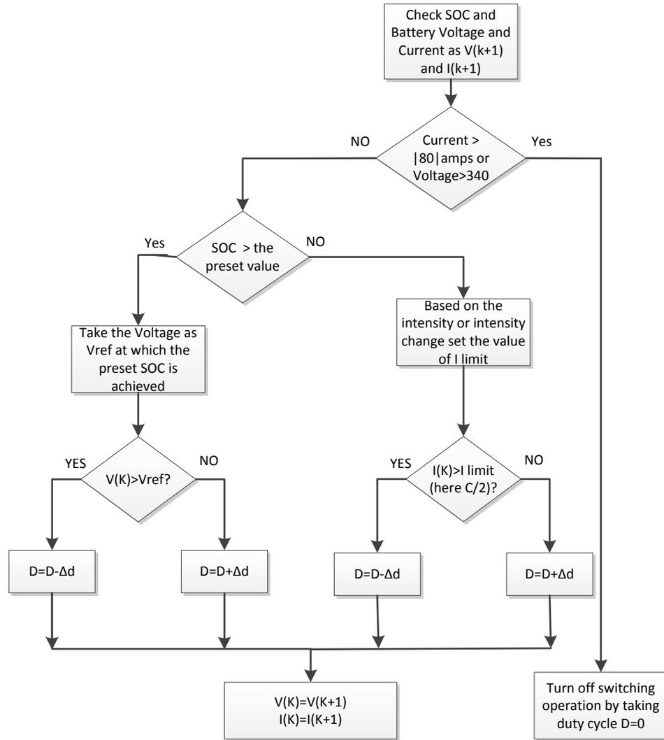
**Figure 5.1: Battery charging algorithm with over charge and over discharge protection**
