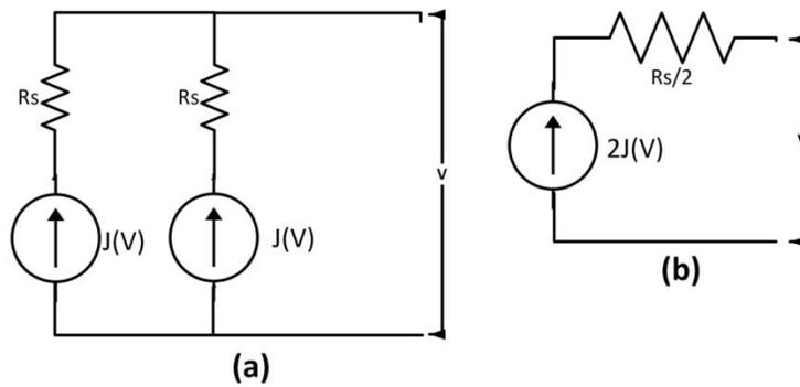
Figure 3.3: (a) 2 solar cells in parallel (b) their Equivalent circuit
