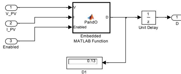
Figure 3.6: Simulink block diagram for MPP
