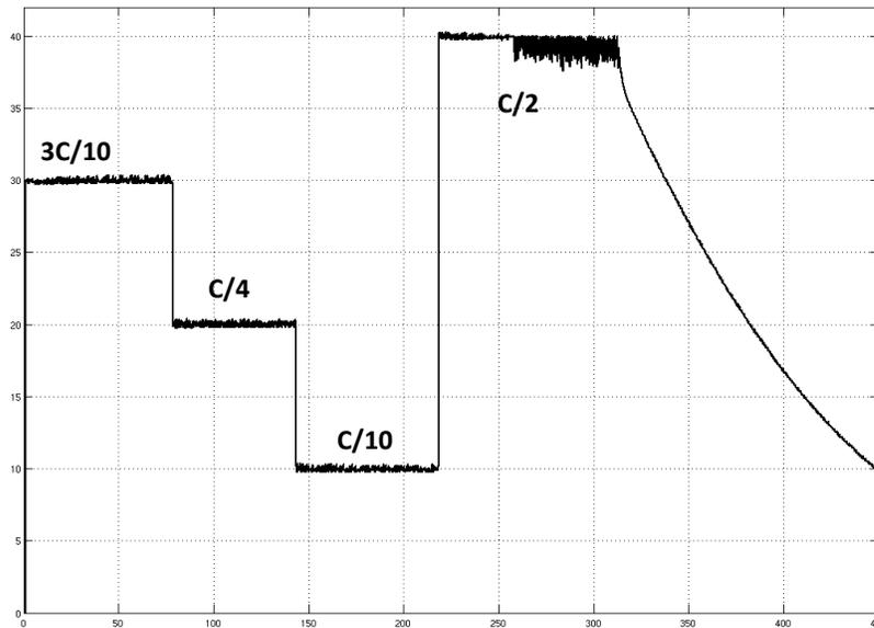
**Figure 6.15: Charging current in different intensity; C/10 constant current in intensity as low as 30%**
