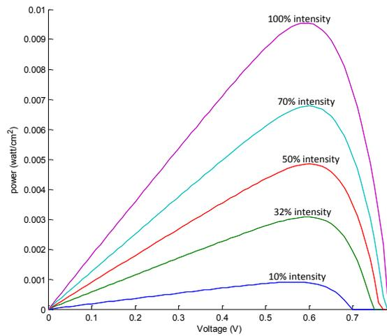
**Figure 2.6: Power vs Voltage characteristics at different intensities**
