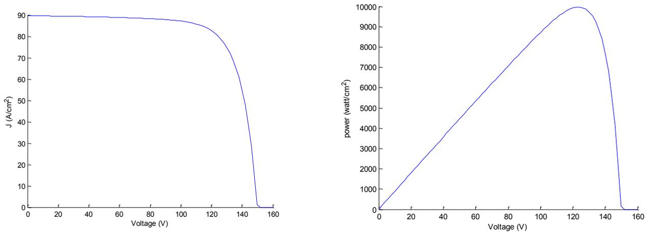
**Figure 6.2: power vs voltage and current vs voltage curve**
