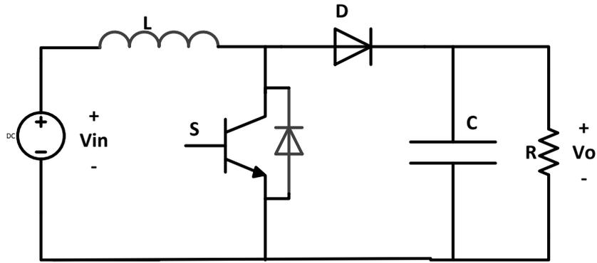
Figure 3.8: DC-DC Boost Converter
