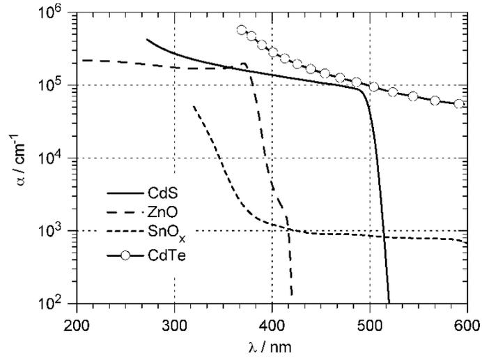
Figure 2.1: Optical absorption coefficient of the absorber, buffer and window layer for CdTe solar cell [8]
