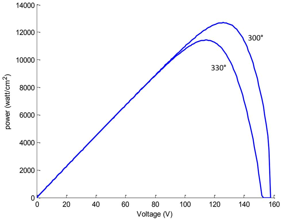
Figure 6.8: temperature effect on power curve
