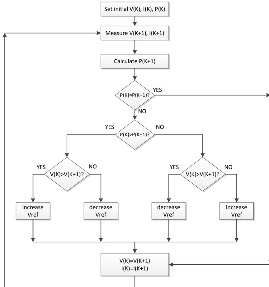
Figure 3.5: Perturb and Observe algorithm flowchart
