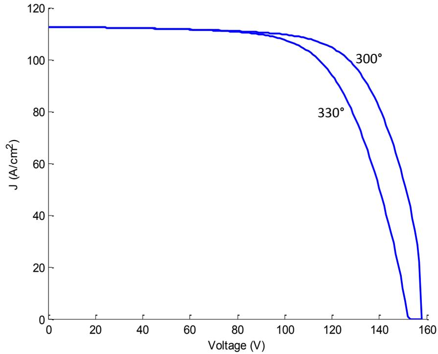
Figure 6.7: temperature effect on current voltage curve
