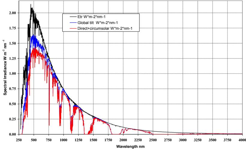
Figure 2.3: Spectral Irradiance Vs wavelengths
