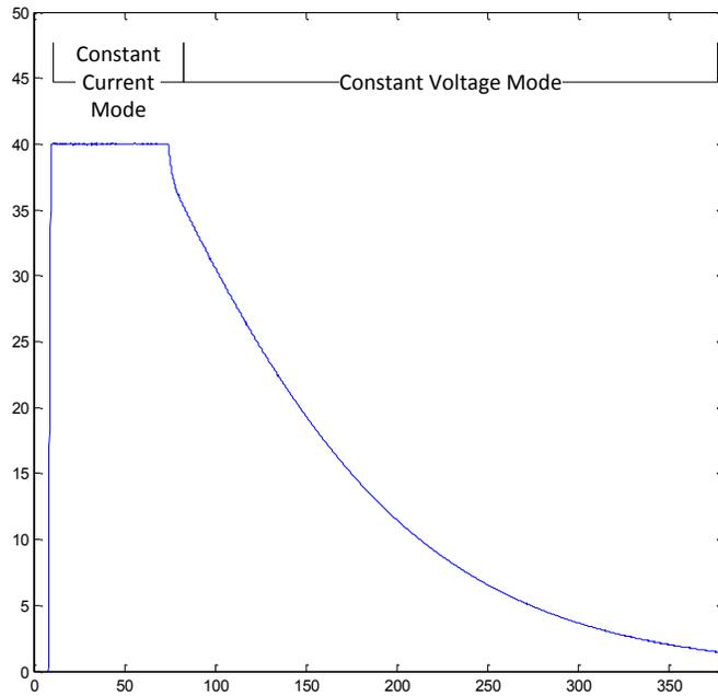
**Figure 6.11: Current Vs time during battery charging**
