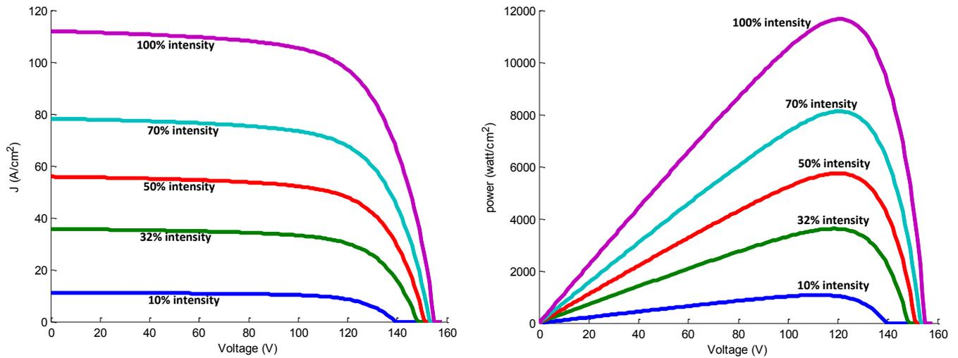
Figure 6.3: current vs voltage and power vs voltage and curve
