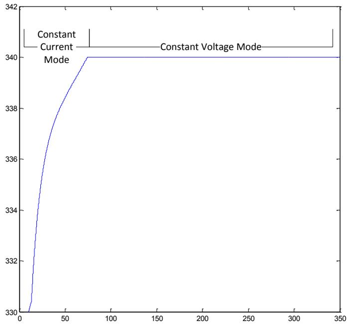
**Figure 6.13: Voltage Vs time during battery charging**
