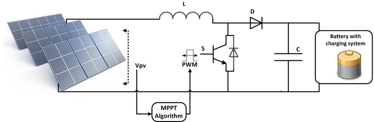
Figure 3.7: dc-dc boost Converter for MPPT
