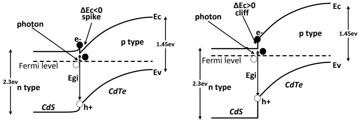
Figure 1.3: Energy band diagrams of CdS/CdTe solar cell structure.
