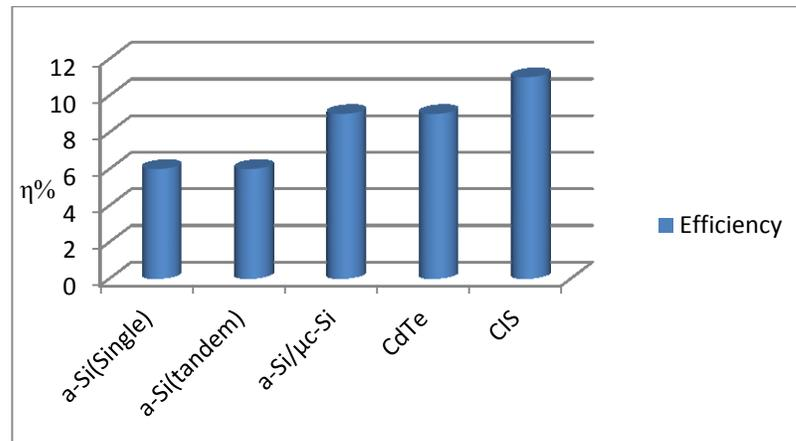
Figure 1.4: Efficiency of different type of thin film solar cells (2006)
