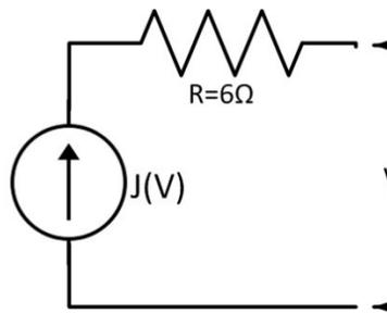
**Figure 2.4: A single solar cell**
