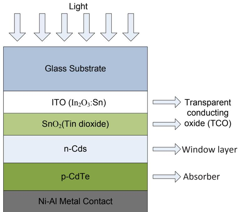
Figure 1.1: Device structure of Thin Film CdS/CdTe solar cell
