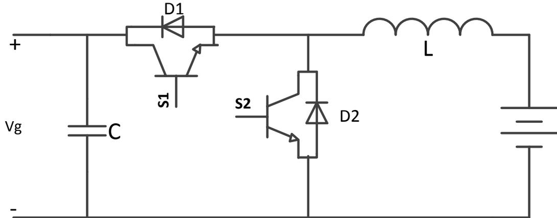
**Figure 5.2: DC-DC Buck converter with two-quadrant switches capable of bidirectional power flow**
