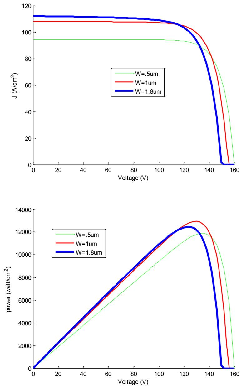
Figure 6.4: Current and Power - voltage characteristics of a CdTe solar cell varying CdTe layer thickness.
