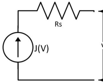
Figure 3.1: A single solar cell
