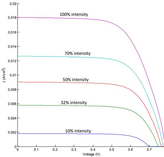
Figure 2.5: Current Voltage characteristics at different intensities
