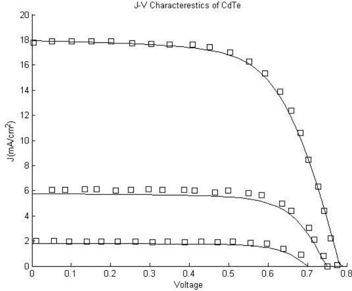
**Figure 6.1: Current Voltage characteristics with experimental data**
