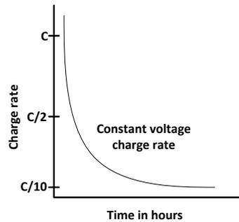
**Figure 4.1: Charging rate VS time in Constant Voltage Charging [29]**
