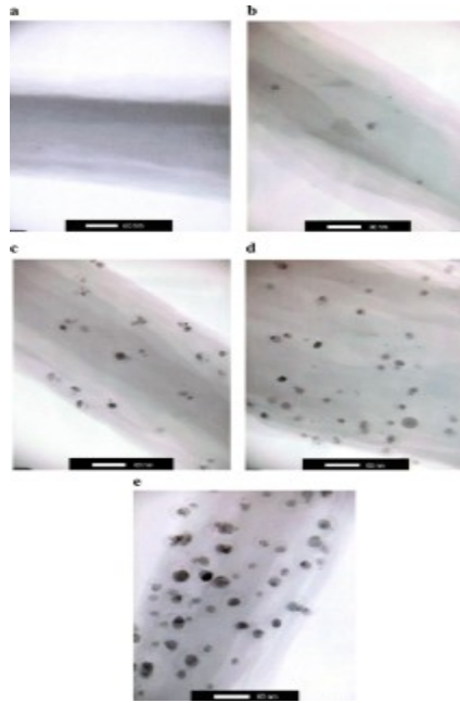
Figure 1.7. TEM images of the cellulose acetate nanofibers containing 0.5 wt% \text{AgNO}_3 at UV irradiation time (a) 0 min, (b) 10 min, (c) 60 min, (d) 120 min, and (e) 240 min [20].
