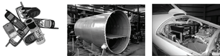
Figure 4 Source (e.g. cell phone), Path Loss (Fuselage), and Victim (e.g. avionic system)
