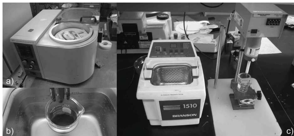
Figure 29 Vacuum mixer (a), solvent/particles in ultrasonic bath (b), mixing equipment (c)
