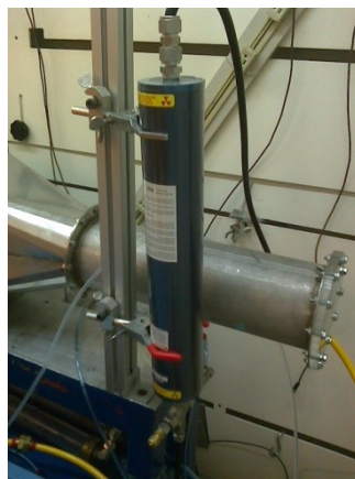
Figure 3-4: Generation system: Kr-85 electrostatic neutralizer
