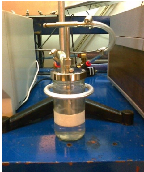
Figure 3-2: Generation system: 6-jet Collison Nebulizer
