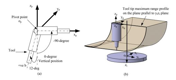
Figure 4. 5- (a) Unsymmetrical limits of spindle rotation & (b) Tool tip maximum range profile on the plane parallel to  $y_t z_t$ -plane.
