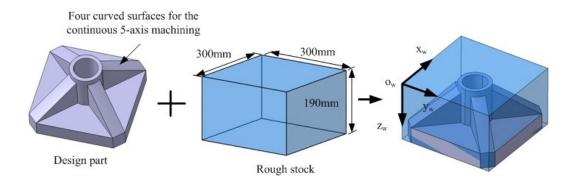
Figure 4.22-Design part (bracket for holding the pipe) and the rough stock.
