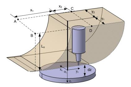
Figure 4.4- x and y travel limits in the table coordinate system 'ot'
