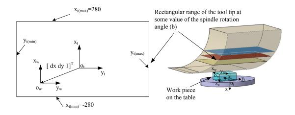
Figure 4.7- Rectangular range at some value of the spindle rotation along with the setup parameters.
