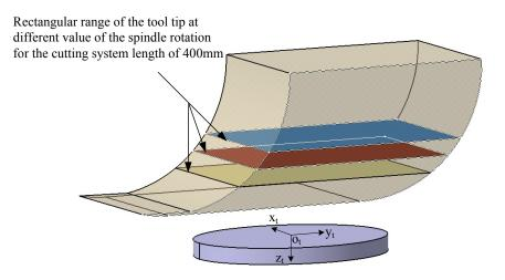
Figure 4. 6- Rectangular range for the different values of the spindle rotation
