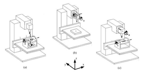
Figure 1.1- Types of 5-axis milling machines: (a) Table-rotating/tilting type (b) Spindle-rotating /tilting type (c) Table/spindle –tilting type
