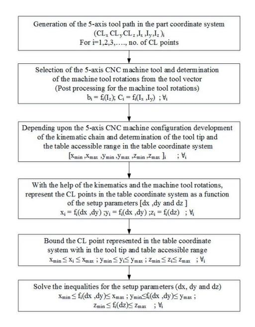
Figure 4.2- Basic methodology for finding the feasible setup parameters.
