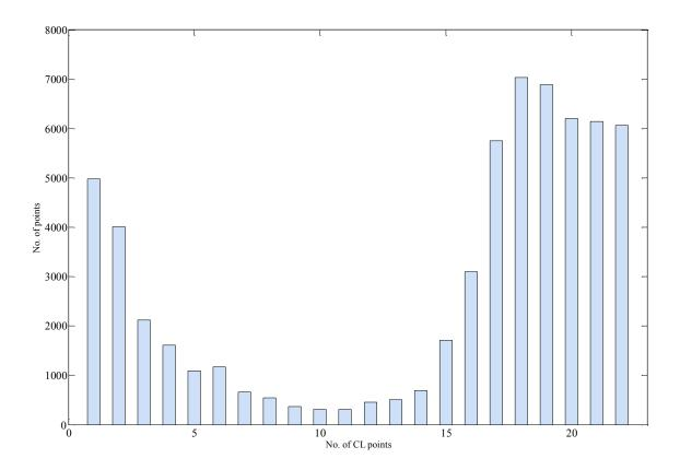
Figure 3.12- No. of points determined from the orthogonal range of the tool holder by Kd-tree structure of 30672 sample points, when tool length is 56.4476mm.
