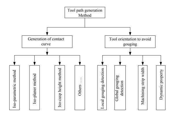
Figure 1.3-Tool path generation method research topics for 5-axis machining
