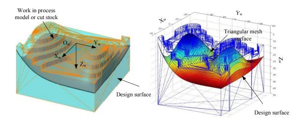
Figure 3.4- Tessellated triangular representation of the in-process work piece model
