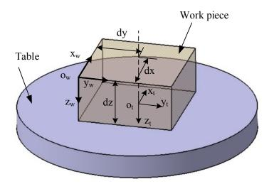
Figure 4.1- Standard setup parameters of a part on the machine table
