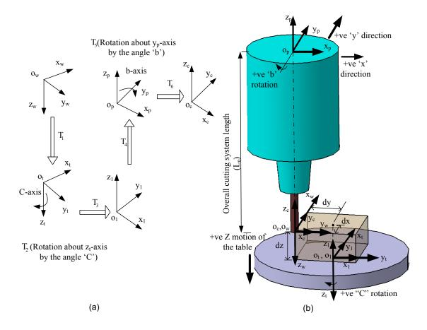
Figure A1- Configuration of DMU 60-T along with the reference coordinate systems
