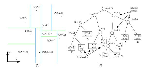
Figure 3.6- (a) Bisecting of the data points (b) Kd-tree data structure
