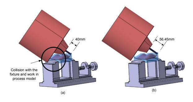
Figure 3.13- At  $3^{rd}$  tool path and  $20^{th}$  cutter location with machine rotations of C= -26.49° b=52.74° (a)Collision of cutting system with the fixture and work in process model with tool length of 40mm. (b) No collision with the tool length of 56.45mm.
