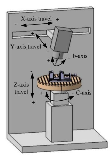
Figure 1.2- Configuration of DMU 60T 5-axis milling machine
