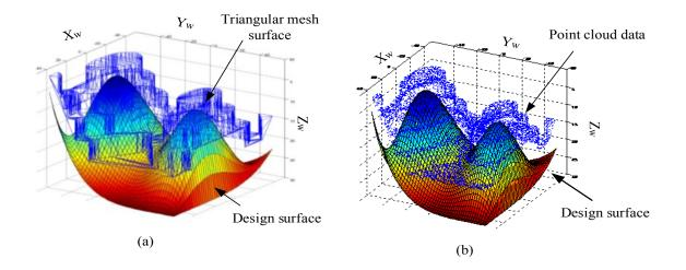
Figure 3.5- (a) Triangular mesh surface (b) point cloud data with D=0.5points/mm<sup>2</sup>
