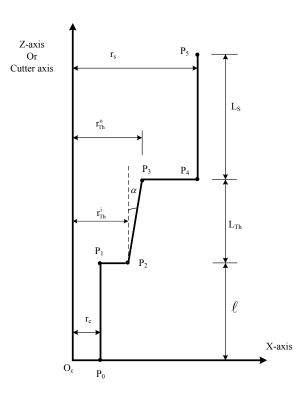
Figure 3.2- Cutting system profile in the cutter coordinate system
