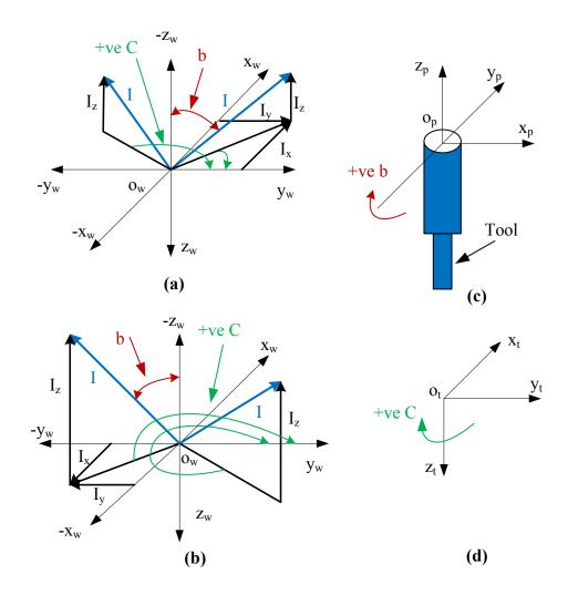
Figure A2- (a) & (b) Positive rotation of the table 'C' for positive rotation of spindle 'b', when tool vector is in different quadrants. (c) & (d) Spindle and table coordinate systems respectively with rotation directions
