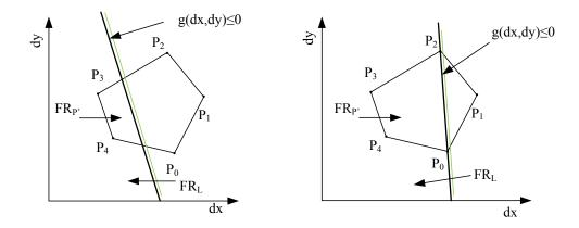
Figure 4.11- Reduction in the feasible region when inequality function is applied or when  $FR_L \cap FR_P = FR_{P'}$
