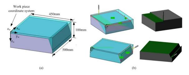
Figure 4.13- (a) Design part with the rough stock. (b) Tool path generation snap shots
