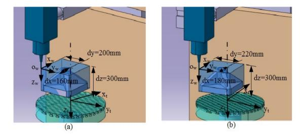
Figure 4.26- (a) Feasible setup of the rough stock. (b) Infeasible setup parameters of the rough stock.
