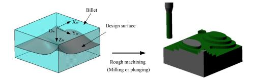
Figure 3.3- In process work piece model after roughing operation
