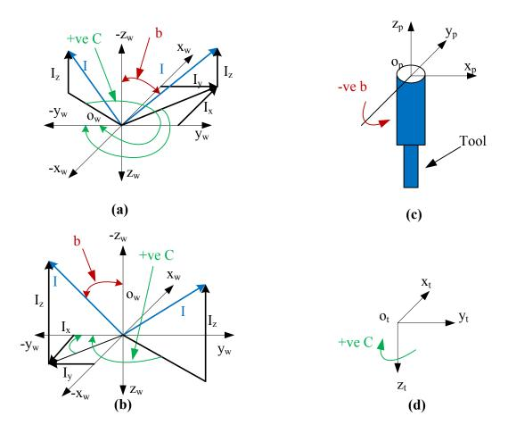
Figure A3- (a) & (b) Positive rotation of the table for the negative rotation of 'b' when the tool vector is in different quadrants. (c) & (d) Spindle and the table coordinate systems respectively with the rotation direction.
