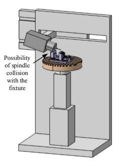
Figure 3.1- Possibility of the spindle collision with the fixture in actual machining environment
