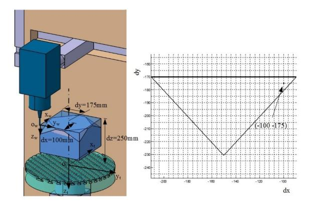
Figure 4.20- Feasible setup of the part on the machine table along with the location of the feasible point inside the final feasible region
