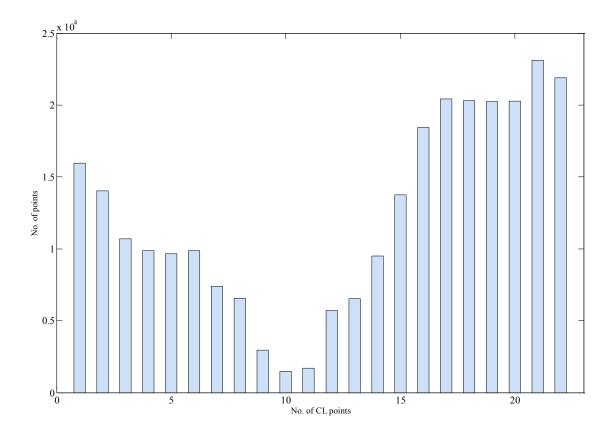
Figure 3.11-No. of points determined from the orthogonal range of spindle by Kd-tree structure of 30672 sample points, when tool length is 40mm.
