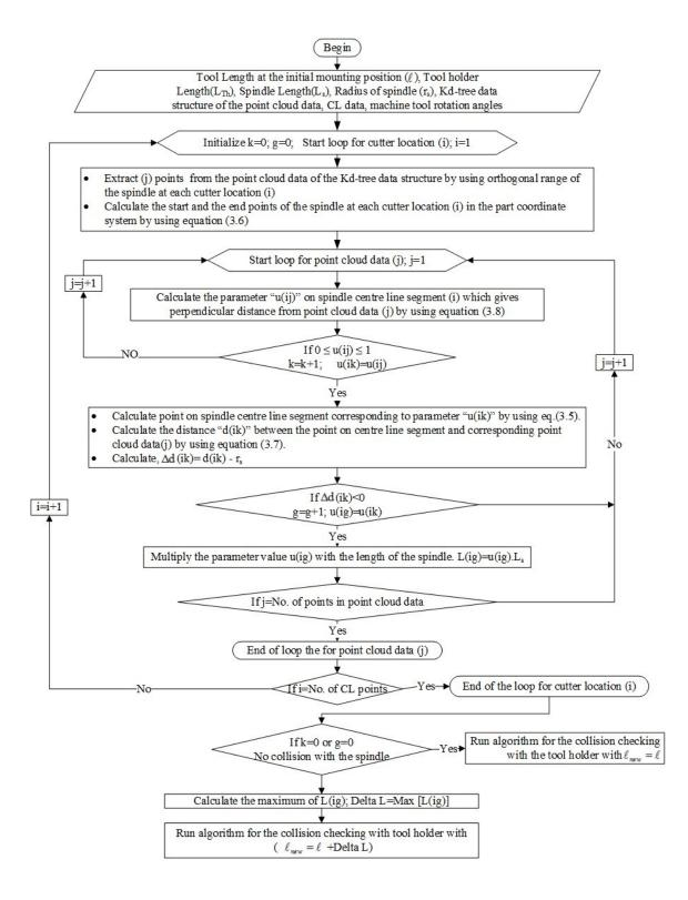
Figure 3.8- Flow chart of the algorithm for the spindle collision detection and removal by the optimum cutter length
