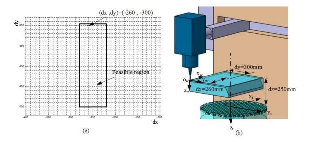
Figure 4.14- (a) Feasible region for selecting the setup parameters. (b) Example of setup the part when setup parameters are selected within the feasible region
