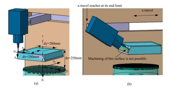
Figure 4.15- (a) Setup of the part when setup parameters are selected from outside the feasible region (b) Snap shot of the simulation showing that further machining is not possible due to the limitation of the x-travel
