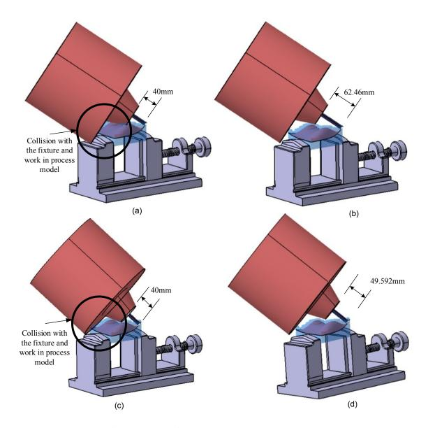
Figure 3. 14-(a) At 2<sup>nd</sup> tool path and 18<sup>th</sup> cutter location with machine rotations of C=-223.477° and b=56.890° collision of the cutting system with the tool length of 40mm. (b) No collision with the tool length of 62.46mm and (c) At 20<sup>th</sup> cutter location with machine rotations of C=-232.22° b=49.15° collision of the cutting system with tool length of 40mm. (d) No collision with the tool length of 49.592mm.
