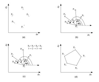
Figure 4.8- (a) Randomly named five vertices of the polygon. (b) Angles measured between the x-axis and the different vectors from the lower left point to the other vertices of the polygon (c) Points arrangement according the ascending order of the 'θ' (d) Final polygon.
