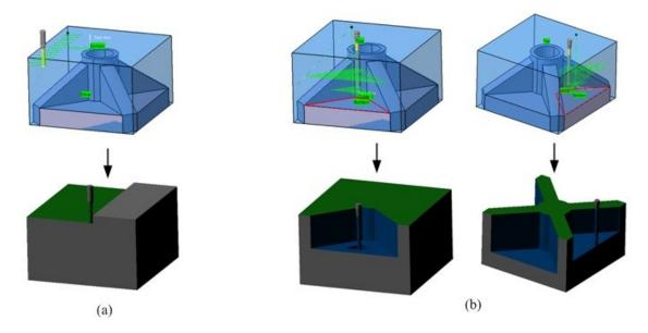
Figure 4.23- (a) Top surface facing (b) Pocketing of the four open islands (bottom faces) with three passes
