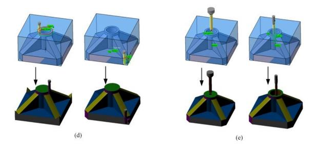
Figure 4.24- (Snap shot contd.): (c) Five axis continuous machining of the top surface of the four supporting ribs with two levels (d) Profile contouring of the cylindrical surface and four edges (e) Drilling and internal pocketing
