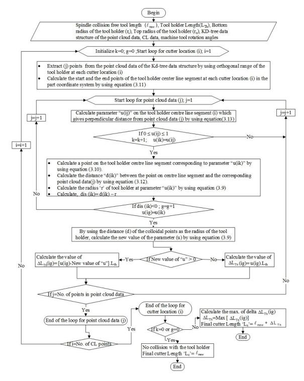
Figure 3.9- Flow chart of the algorithm for the tool holder collision detection and removal by the optimum cutter length
