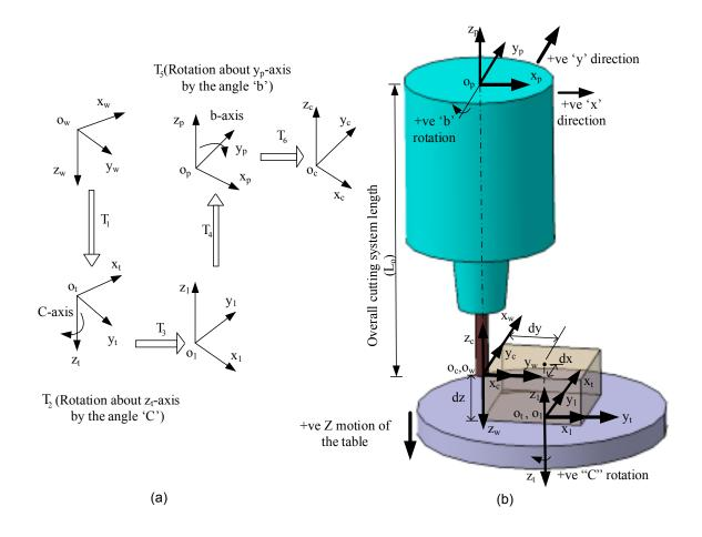
Figure 4.3- (a) Transformation sequence along with the reference coordinate system. (b) Standard setup of the part on the machine table.
