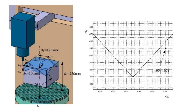
Figure 4.21- Infeasible setup of the part on the machine table along with the location of the feasible point outside the final feasible region.
