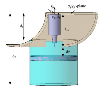
Figure 4.12- Table travel limit along with the machine constants  $d_1$  and  $d_2$
