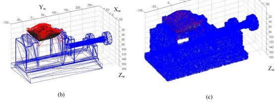
Figure 3.10-(a) Solid model (b) Triangular tessellation representation. (c) Point cloud data representation of the work in process model along with the fixture in part coordinate system.
