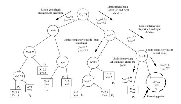
Figure 3.7- Checking procedure for the orthogonal searching query
