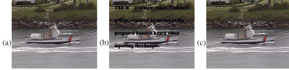
Figure 4.11: a) Original frame. b) Damaged frame. c) Completion result by our method (Frame number 11, MSE=8.16).
