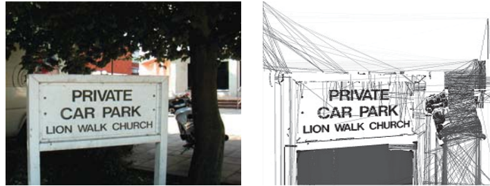
Figure 4.4: The original image and the SWT output using bandlet-based edges are shown at left and right, respectively.
