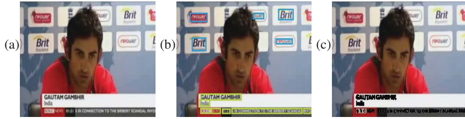
Figure 4.6: Output results of video text detection. a) Original frame. b) Video text detection result. The video text objects are differentiated from the other text objects by another color. c) Detected video text is removed and masked.
