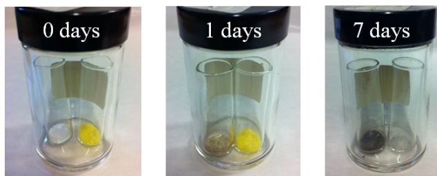
Figure 43. Vapor phase synthesis of 2,5-di(octadecylamino)-1,4-quinone, C18p . With time, the quantity of yellow 1,4-benzoquinone reduces, and white octadecylamine gradually darkens, which indicates a reaction has occurred.
