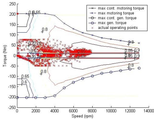
**Fig. 2-9** Traction motor operating points
