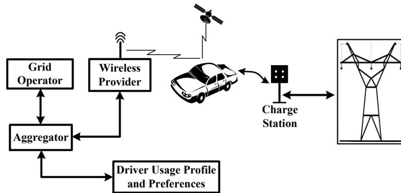
**Fig. 4-2** Schematic diagram of V2G connection
