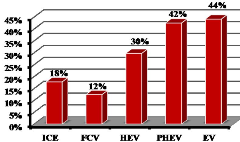
Fig. 2-12 WTW efficiency of different drivetrains
