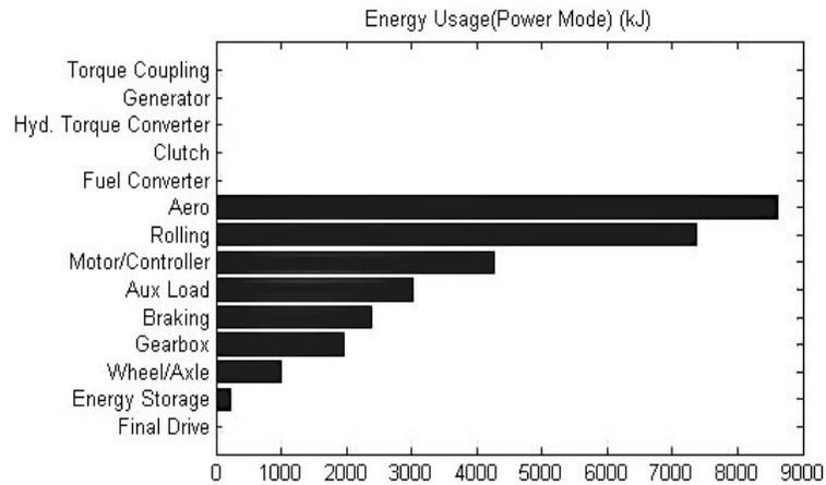
**Fig. 2-11** EV total loss distribution (motoring mode) over driving cycle
