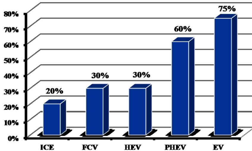
**Fig. 1-7** Average theoretical Back-of-Envelope TTW efficiency of different drivetrains
