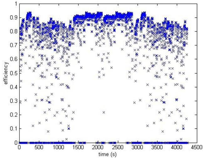
**Fig. 2-10** Motor controller efficiency (motoring mode) during driving schedule
