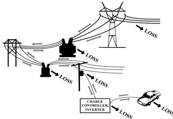
**Fig. 4-4** Energy transmission and conversion losses
