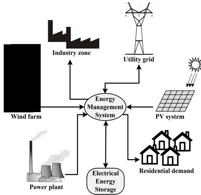
**Fig. 4-5** Virtual power plant structure
