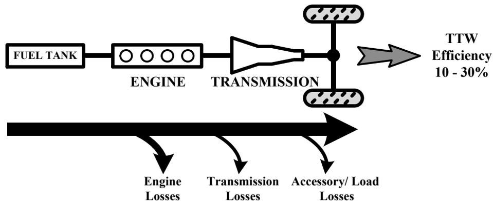
**Fig. 1-2** Schematic diagram of gasoline vehicle drivetrain
