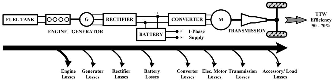
**Fig. 1-5** Schematic diagram of series plug-in hybrid electric vehicle drivetrain
