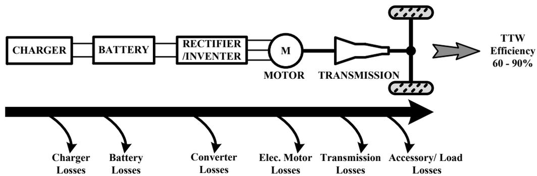
**Fig. 1-6** Schematic diagram of electric vehicle drivetrain
