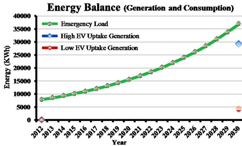
**Fig. 5-9** Energy balance between emergency load and EVs generation in islanded area
