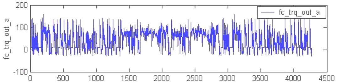
**Fig. 2-4** above: time-aligned vehicle driving speed. Below: engine torque delivery
