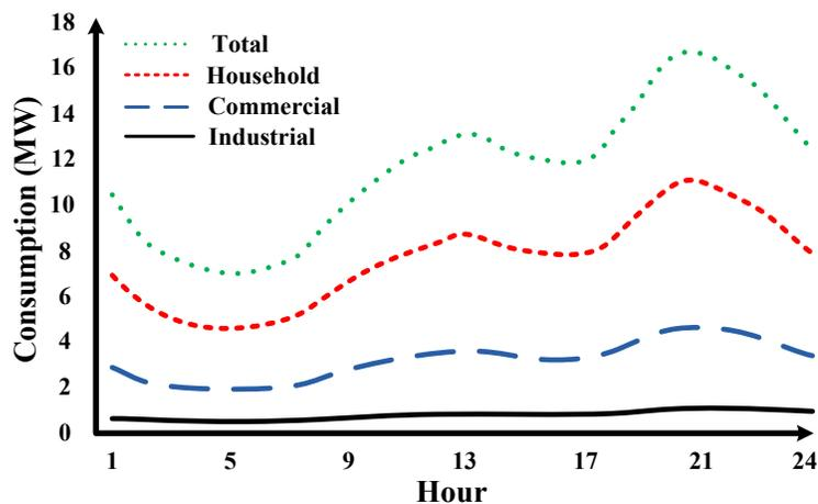
Fig. 4-1 Typical 24 hour load profile
