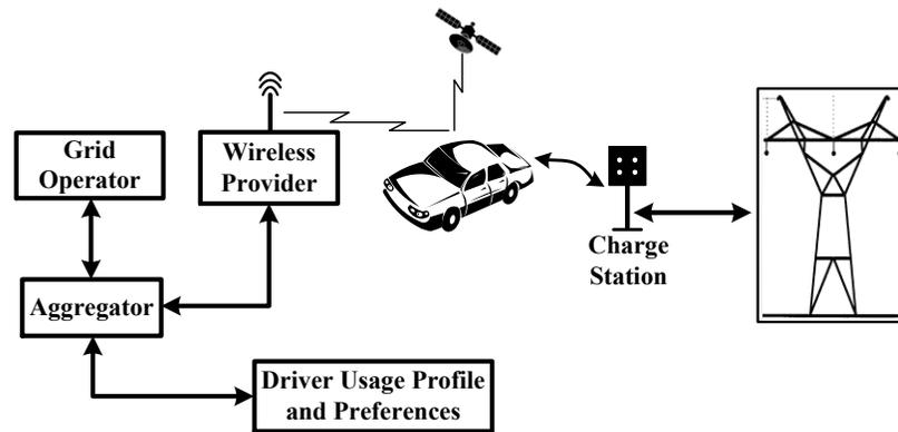
**Fig. 4-2** Schematic diagram of V2G connection
