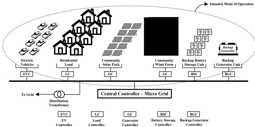
**Fig. 5-1** Future smart microgrid configuration and islanded mode of operation
