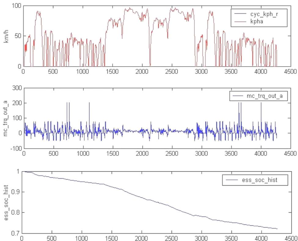
**Fig. 2-8** a. above: drive cycle, b. middle: EV simulated torque delivered by motor over drive cycle (negative during regenerative braking), c. below: state of Li-ion battery charge history during drive cycle
