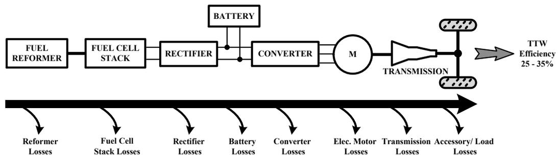
Fig. 1-4 Schematic diagram of fuel cell vehicle drivetrain
