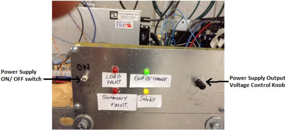
Fig. 4.30 Power supply control interface
