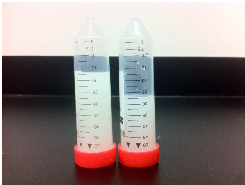
Figure 3.3: Suspension of tungsten oxide nano-powders in a mixture of deionized water and methanol
