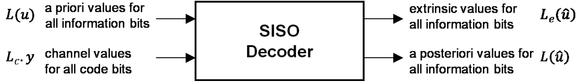
Figure 2.14 “Soft Input, Soft Output” decoder
