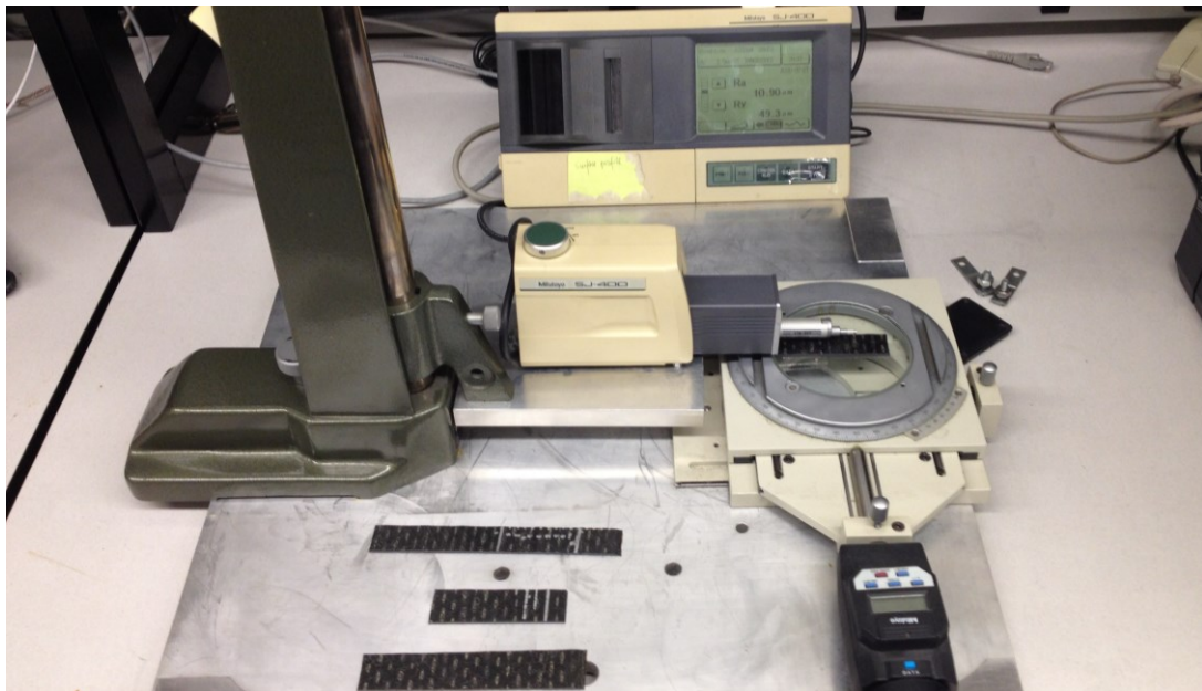
Figure 3.27 Mitutoyo Surftest SJ 400 Profilometer
