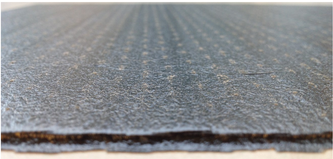
Figure 3.24 Final Sample made by the AFP Process ([0] 16 ) using TC-250 Material
