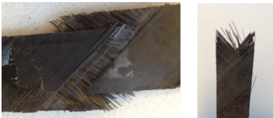
Figure 4.6 In-Plane Shear Test Coupon Failure
