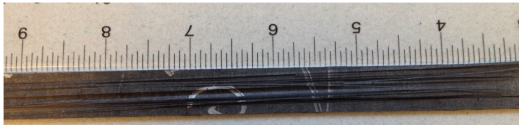
Figure 4.2 Tensile Test coupons (0°) failed under the XGM and SGM Failure Modes respectively
