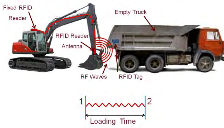
Figure 3-40: RFID reader captured data with excavator
