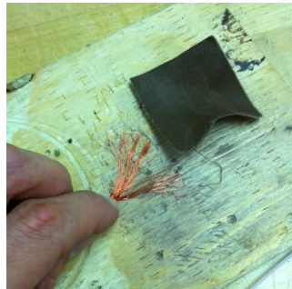
Fig. 4-12 Stripping strands insulation using sand paper
