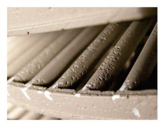
Figure 2.17: The blade erosion [17].
