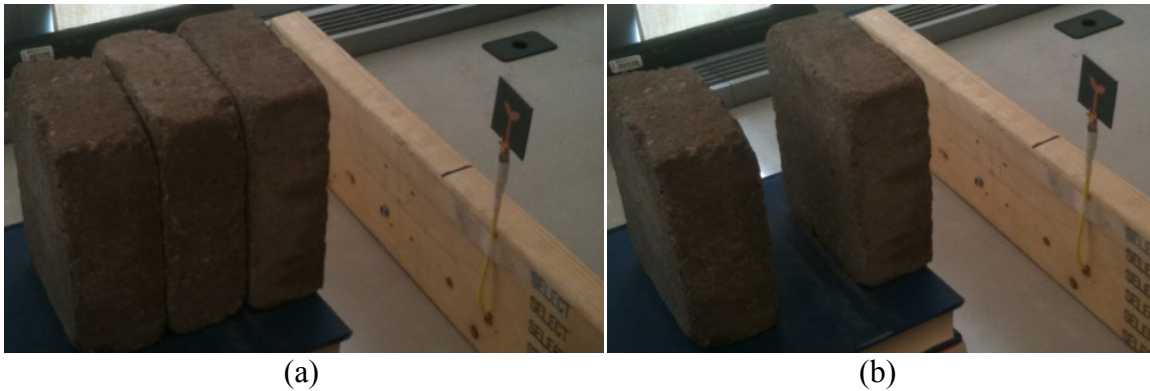
Figure 6.11 Practical measurement arrangements (a) solid sandy brick wall (b) two walls separated by a distance ( d ).
