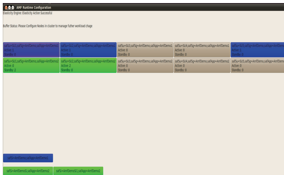
Figure 38 - System Configuration after EE and AMF actions for the workload increase in a SG with N-way-Active redundancy model
