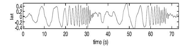
Figure 2.3: Example of two concatenated chirps applied on lateral stick of R-50 UAV helicopter for model identification in hover regime [1]
