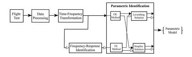
Figure 4.5: Schematic of the parametric SID tool
