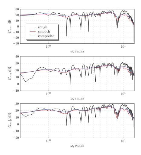
Figure 3.8: Estimated spectral functions for roll motion
