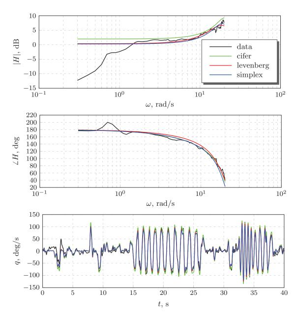
Figure 4.7: Identification results: FE method for short-period dynamics
