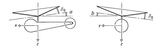
Figure 4.2: Rotor blades flapping motion [4]
