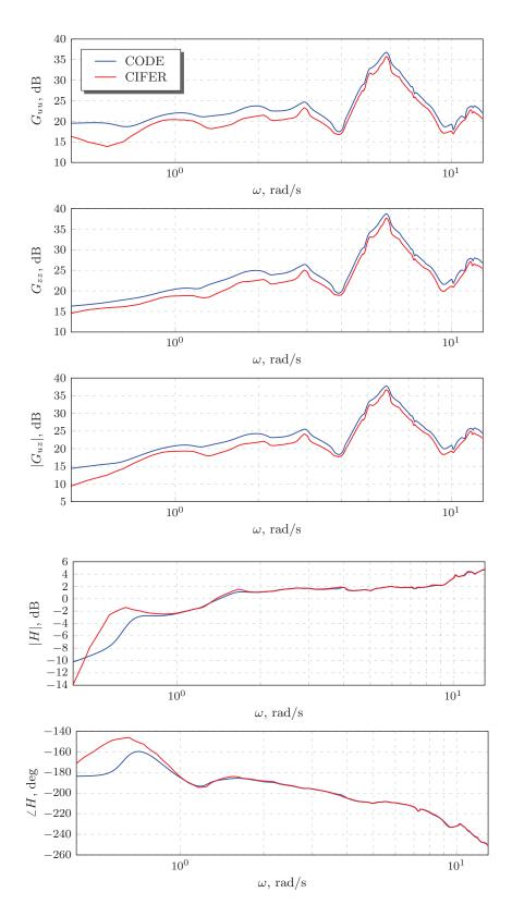
Figure 3.6: Identification results for longitudinal mode
