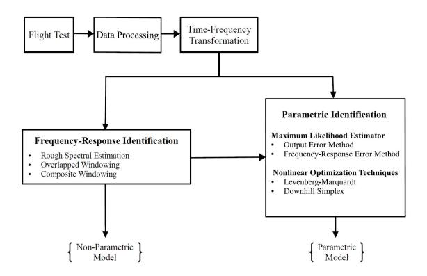
Figure 1.2: Schematic of the developed identification tool
