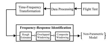
Figure 3.3: Schematic of non-parametric SID tool
