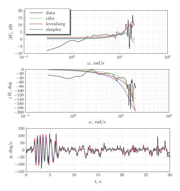
Figure 4.8: Identification results: FE method for roll dynamics
