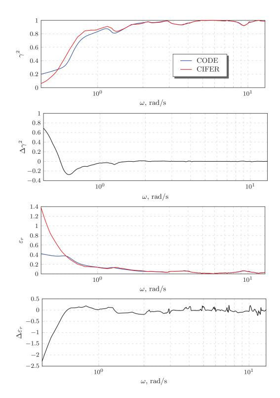
Figure 3.7: Accuracy metrics for longitudinal mode identification
