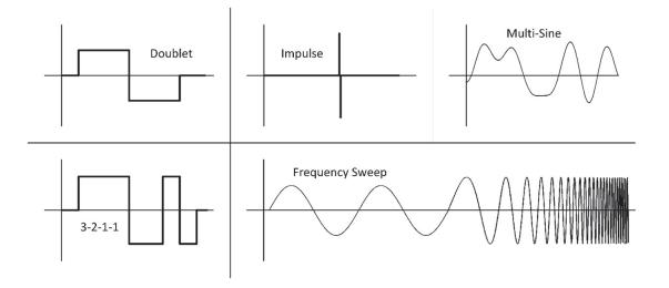
Figure 2.2: Conventional input types used in aircraft system identification
