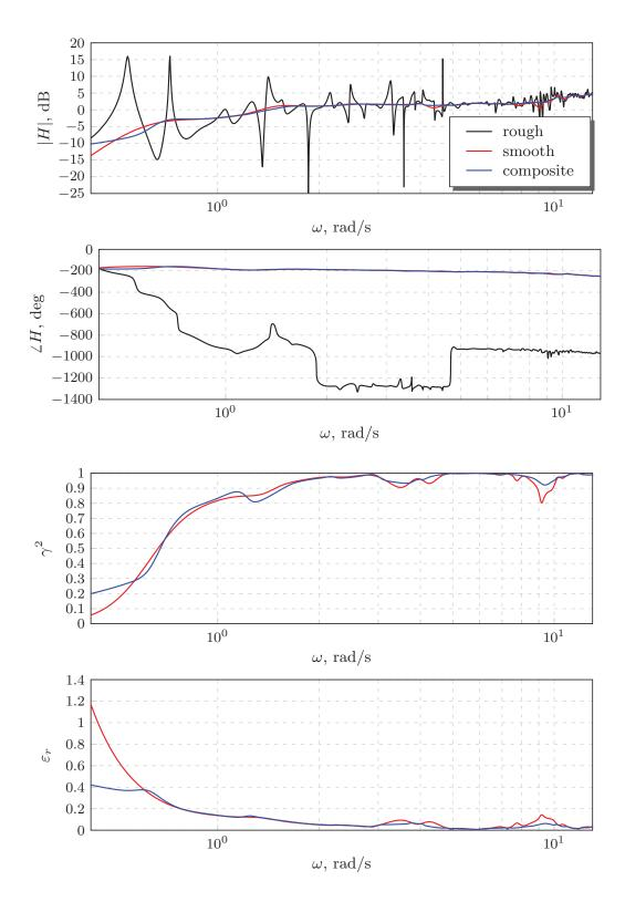
Figure 3.5: Estimated frequency-response function for pitch motion
