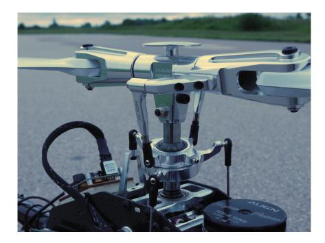
Figure 4.1: Swashplate mechanism of Align Trex-700, © MicroPilot
