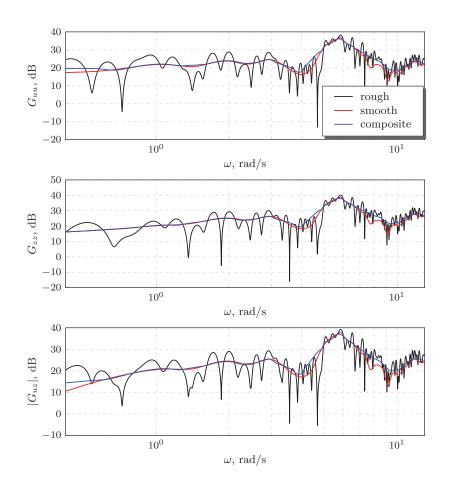
Figure 3.4: Estimated spectral functions for pitch motion
