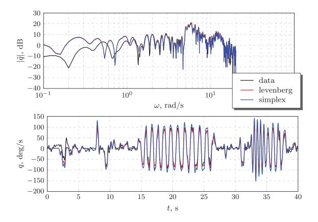
Figure 4.6: Identification results: OE method for short-period dynamics
