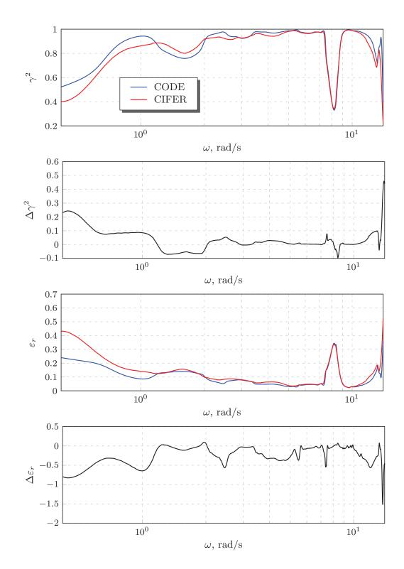
Figure 3.11: Accuracy metrics for lateral mode identification
