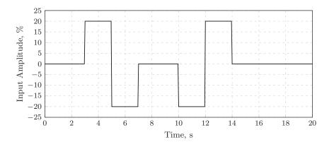
Figure 2.6: Schematic of the designed doublet input
