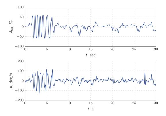
Figure 2.10: Flight test results: measured input-output for lateral mode
