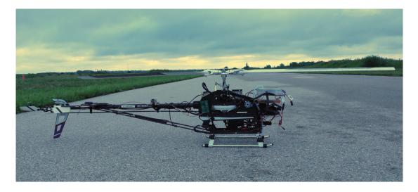
Figure 2.8: Armed Trex-700 used for identification experiment, © MicroPilot
