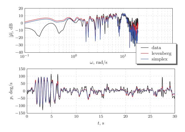
Figure 4.9: Identification results: OE method for roll dynamics
