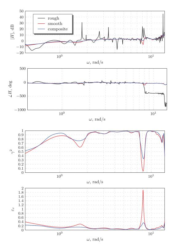
Figure 3.9: Estimated frequency-response function for roll motion
