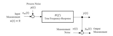
Figure 3.2: Measurement noise in input and output signals
