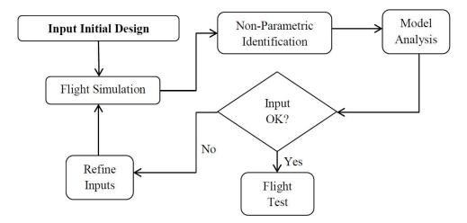
Figure 2.1: Iterative procedure of input design
