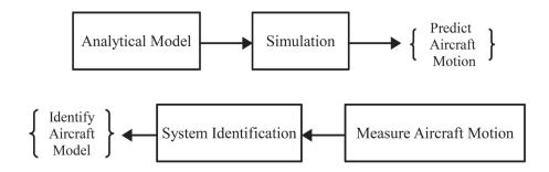
Figure 1.1: Schematic of system identification procedure
