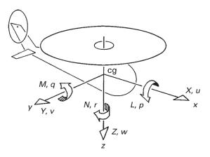
Figure 4.3: Helicopter body-fixed frame [4]
