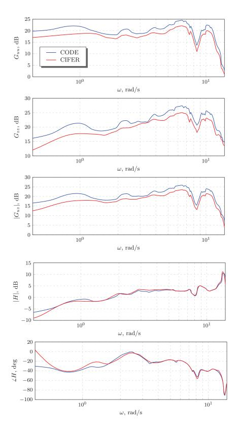
Figure 3.10: Identification results for lateral mode
