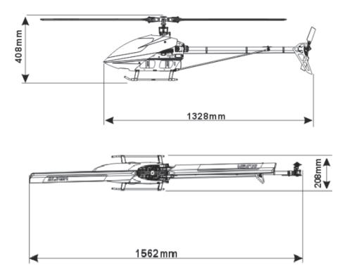
Figure 2.7: Trex-700 dimensions based on its operating manual
