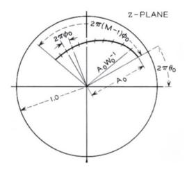
Figure 3.1: Illustration of CZT in z-plane [3]
