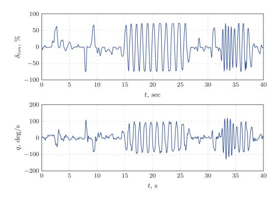
Figure 2.9: Flight test results: measured input-output for longitudinal mode
