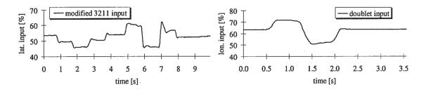
Figure 2.4: Examples of actual multi-step input: Excited lateral and longitudinal sticks of BO-105 helicopter used for hover model validation [2]
