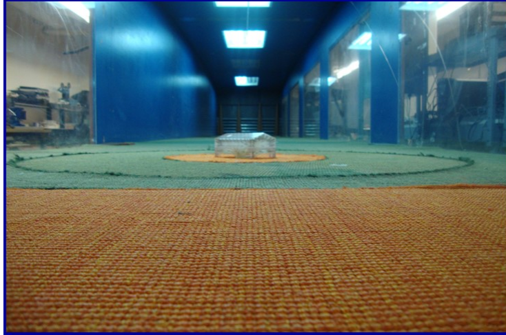
Figure 2-3. Front view section of the Boundary Layer Wind tunnel at Concordia University, Montreal, Canada
