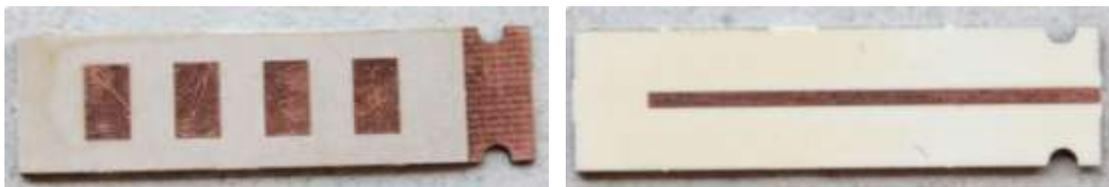
Figure 3.14 Prototype for Four element patch antenna structure
