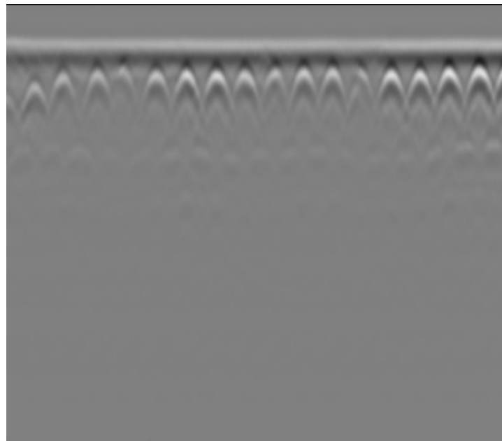
Fig. A. 18 Example of GPR image
