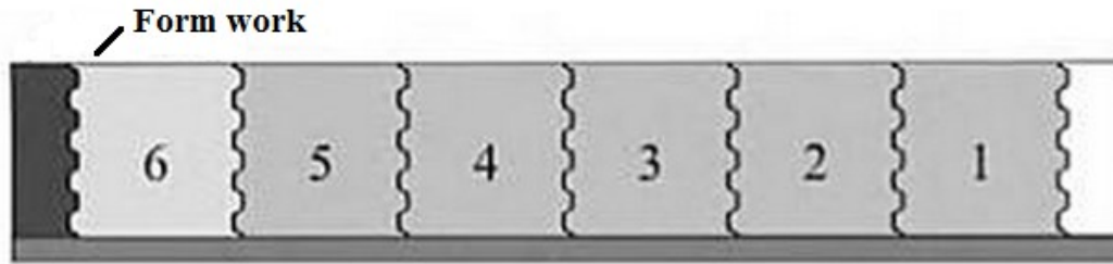
Figure 2-5: Long line casting method (Abendeh, 2006)
