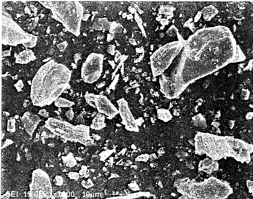
Figure 3. 4 SEM image of tailings, magnification 1000X, length of bar 10µm (Razavi, 2007)
