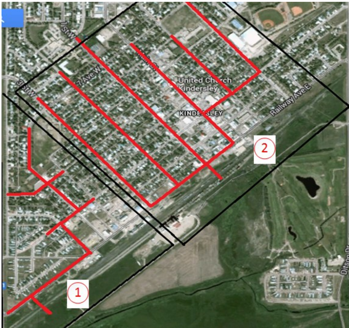
Figure 4-6: Storm Pipe network One and Two
