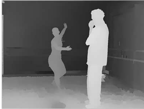
FIGURE 2.8: Depth map. Objects closer to the sensor are whiter.
