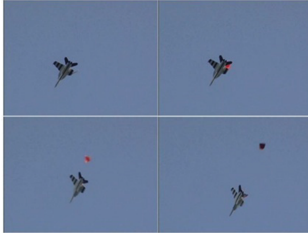
Figure 1.6: Simulated wing damage of 60% in F/A-18 subscale UAV [28]
