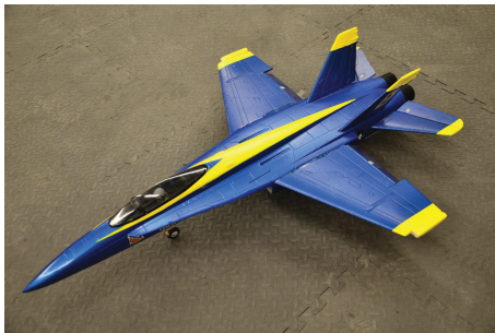
Figure A.9: F-18 UAV testbed
