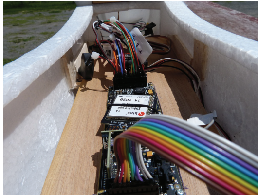
Figure A.3: MP2128H autopilot installed on A380 UAV
