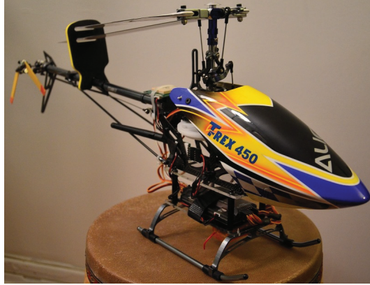
Figure A.8: T-rex 450 single rotor helicopter built for SI purposes
