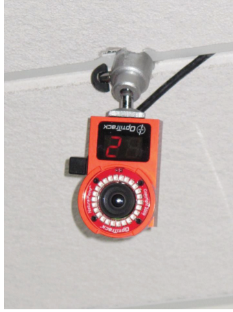
Figure 4.3: V100:R2 camera used for Optitrack positioning system
