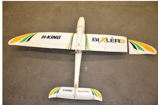
Figure A.5: Bixler 2 UAV with the split wing mechanism
