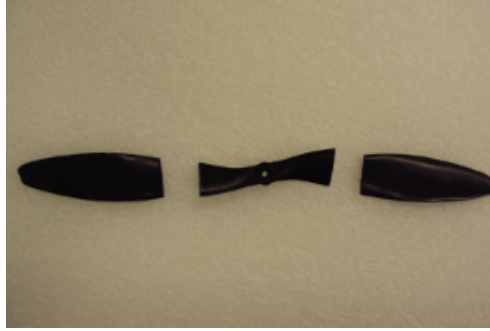
Figure 4.23: A 70% damaged propeller
