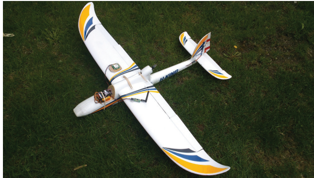
Figure 3.1: The HK Bixler UAV testbed with equipped avionics
