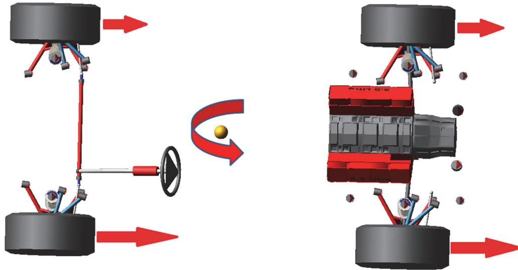
Figure 1. 8 Differential braking system
