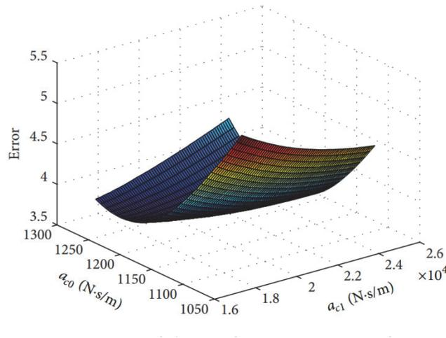
Figure 4. 4 Sensitivity of objective function to variation of viscosity parameters of MR damper in 1.5 Hz
