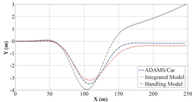
Figure 2. 6 Planar motion of vehicle in the double lane change maneuvering using ADAMS/Car, integrated and handling model (7-DOF)
