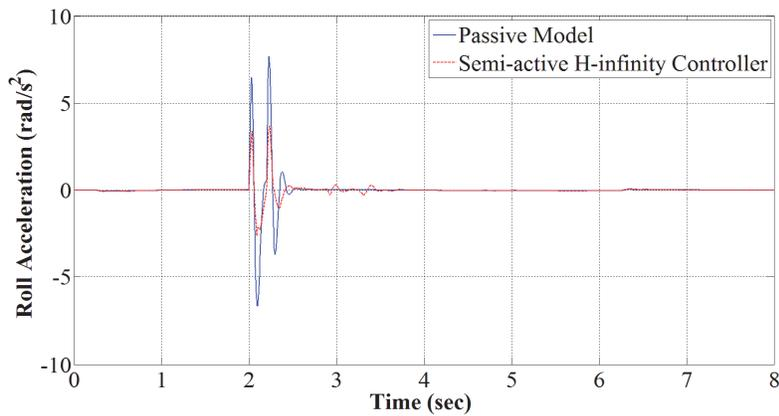
Figure 5. 23 Roll acceleration of vehicle body in dry asphalt condition  $\mu = 0.7$
