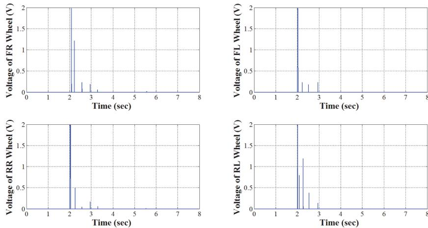
Figure 5. 27 Voltage of MR dampers in dry asphalt condition  $\mu = 0.7$
