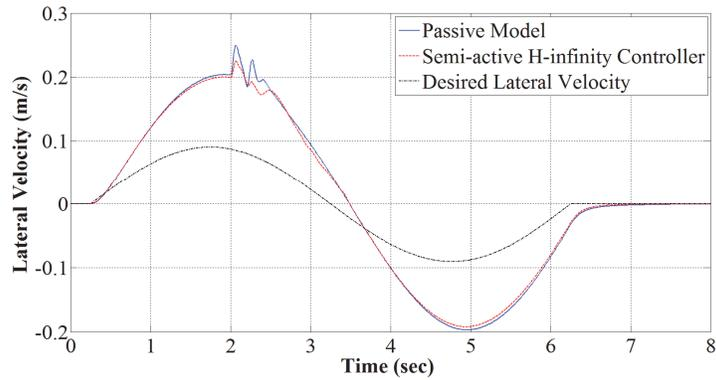
Figure 5. 10 Lateral velocity of vehicle in rainy asphalt condition  $\mu = 0.5$  for single lane change maneuver
