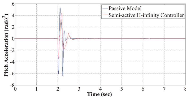
Figure 5. 26 Pitch acceleration of vehicle body in dry snowy condition  $\mu = 0.3$
