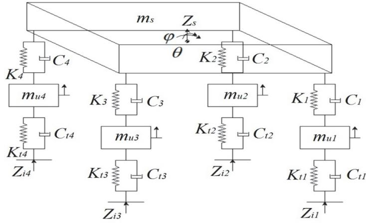
Figure 1. 3 Schematic of Full Car model
