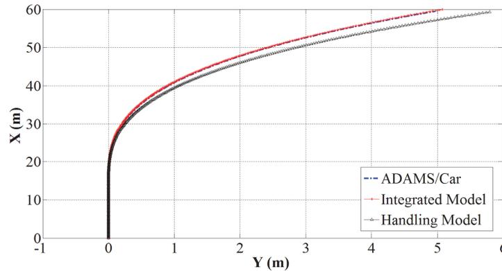
Figure 2. 7 Comparison of ADAMS/Car, integrated model and handling model in planar motion for ramp steering
