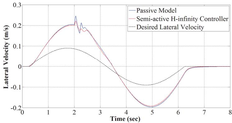
Figure 5. 9 Lateral velocity of vehicle in dry asphalt condition  $\mu = 0.7$  for single lane change maneuver
