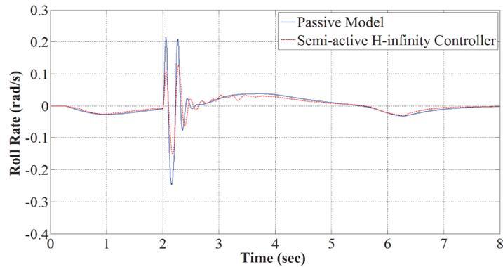
Figure 5. 18 Roll rate of vehicle body in snowy asphalt condition  $\mu = 0.3$
