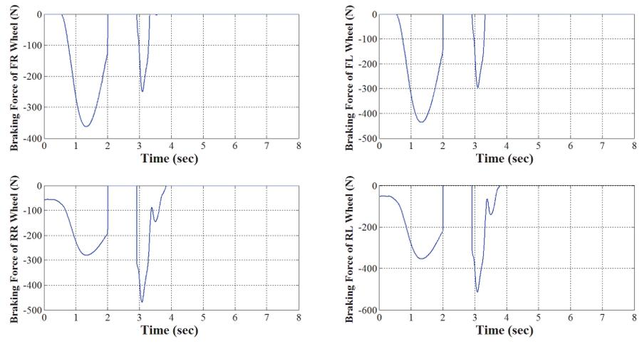
Figure 5. 14 Braking force acting on each wheel in snowy asphalt condition  $\mu = 0.3$  for single lane change maneuver
