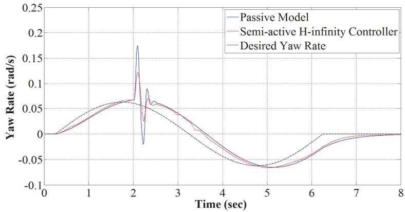
Figure 5. 7 Yaw rate of vehicle in rainy asphalt condition  $\mu = 0.5$  for single lane change maneuver
