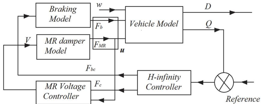
Figure 3. 1 Block diagram of the robust control algorithm.
