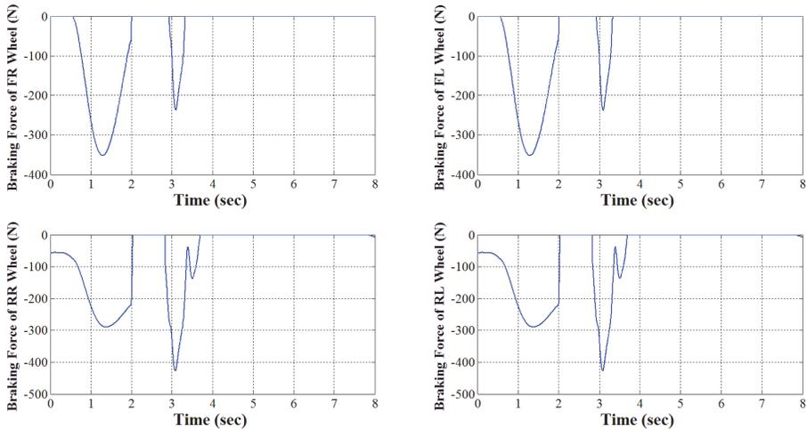
Figure 5. 12 Braking force acting on each wheel in dry asphalt condition  $\mu = 0.7$  for single lane change maneuver
