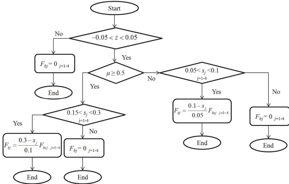
Figure 4. 11 The braking action algorithm
