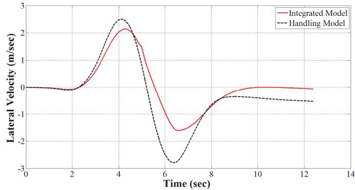
Figure 2. 12 Lateral velocity of integrated and the ride model
