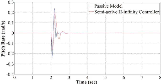
Figure 5. 19 Pitch rate of vehicle body in dry asphalt condition  $\mu = 0.7$
