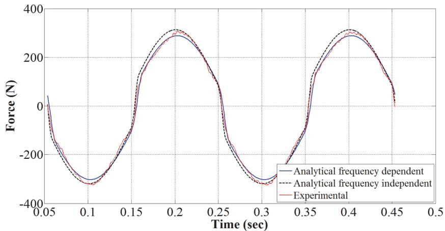
Figure 4. 9 MR damper force in frequency 2.5 Hz and zero current
