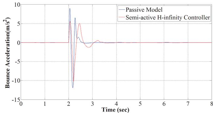
Figure 5. 22 Vertical acceleration of vehicle body in dry snowy condition  $\mu = 0.3$
