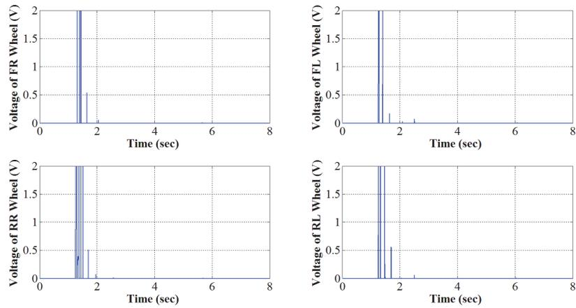
Figure 5. 28 Voltage of MR dampers in snowy asphalt condition  $\mu = 0.3$
