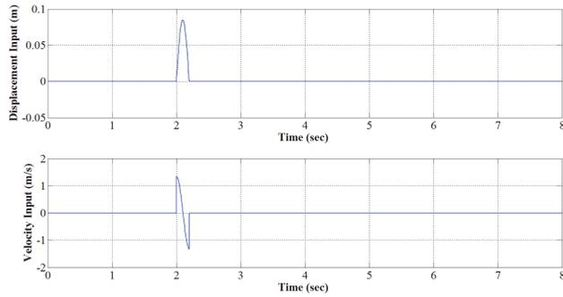
Figure 5. 2 Road input under front right wheel
