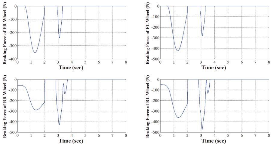
Figure 5. 13 Braking force acting on each wheel in rainy asphalt condition  $\mu = 0.5$  for single lane change maneuver
