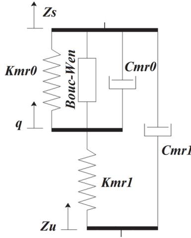
Figure 4. 1 Schematic of Spencer model
