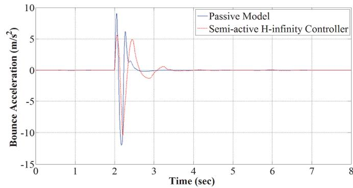
Figure 5. 21 Vertical acceleration of vehicle body in dry asphalt condition  $\mu = 0.7$
