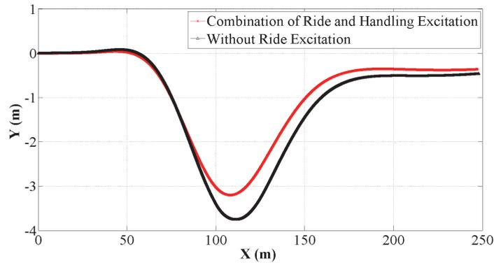
Figure 2. 8 Simulation of the double lane change motion of vehicle with and without ride excitation using integrated model
