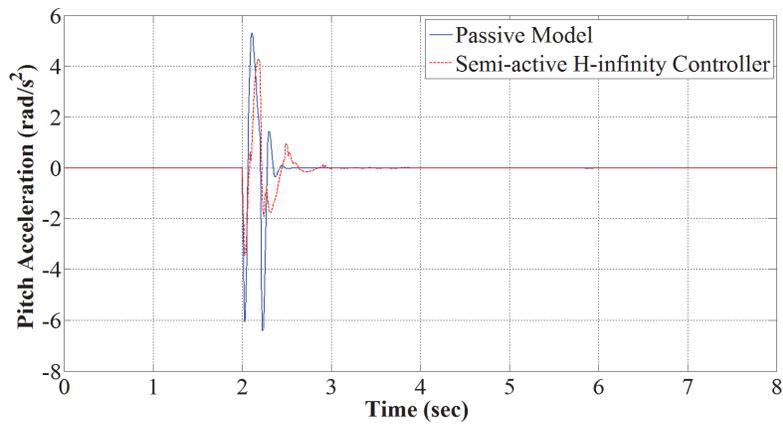
Figure 5. 25 Pitch acceleration of vehicle body in dry asphalt condition  $\mu = 0.7$
