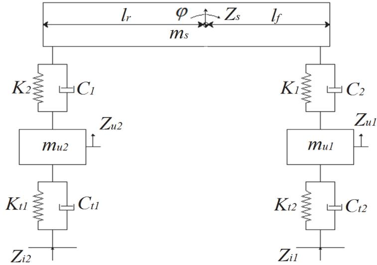
Figure 1. 2 Schematic of Half Car model
