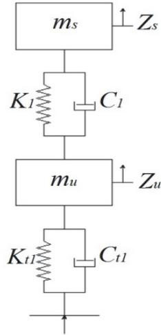
Figure 1. 1 Schematic of Quarter Car model
