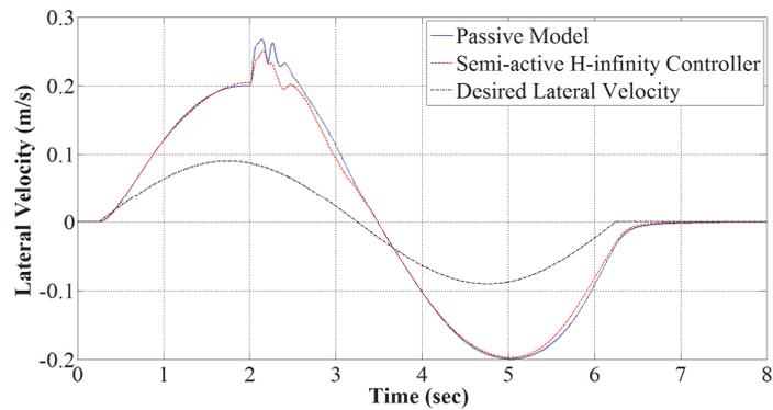
Figure 5. 11 Lateral velocity of vehicle in snowy asphalt condition  $\mu = 0.3$  for single lane change maneuver
