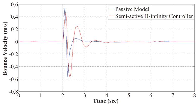
Figure 5. 16 Bounce velocity of vehicle body in snowy asphalt condition  $\mu = 0.3$
