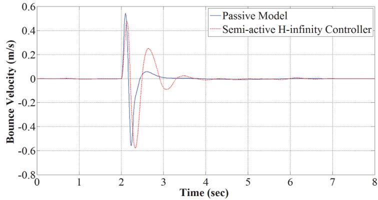
Figure 5. 15 Bounce velocity of vehicle body in dry asphalt condition  $\mu = 0.7$
