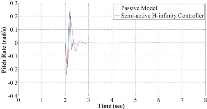
Figure 5. 20 Pitch rate of vehicle body in snowy asphalt condition  $\mu = 0.3$
