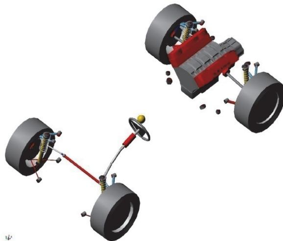
Figure 2. 4 Vehicle model simulated in ADAMS software
