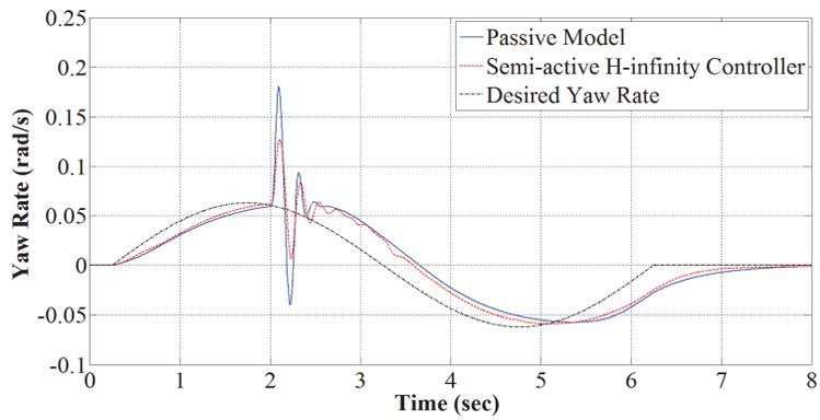
Figure 5. 8 Yaw rate of vehicle in snowy asphalt condition  $\mu = 0.3$  for single lane change maneuver
