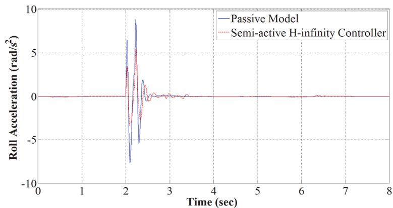
Figure 5. 24 Roll acceleration of vehicle body in dry snowy condition  $\mu = 0.3$
