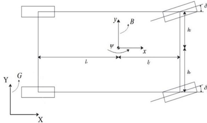
Figure 2. 3 Top view of the handling system model
