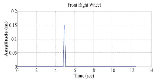
Figure 2. 5 (a) Steering angle for double lane-change based on ISO, (b) steering angle with amplitude of 3.5 (degree) and duration of 3 (sec), (c) bump speed with 5 (m) length and 0.15 (m) amplitude
