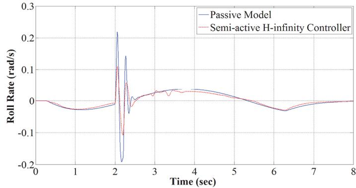
Figure 5. 17 Roll rate of vehicle body in dry asphalt condition  $\mu = 0.7$
