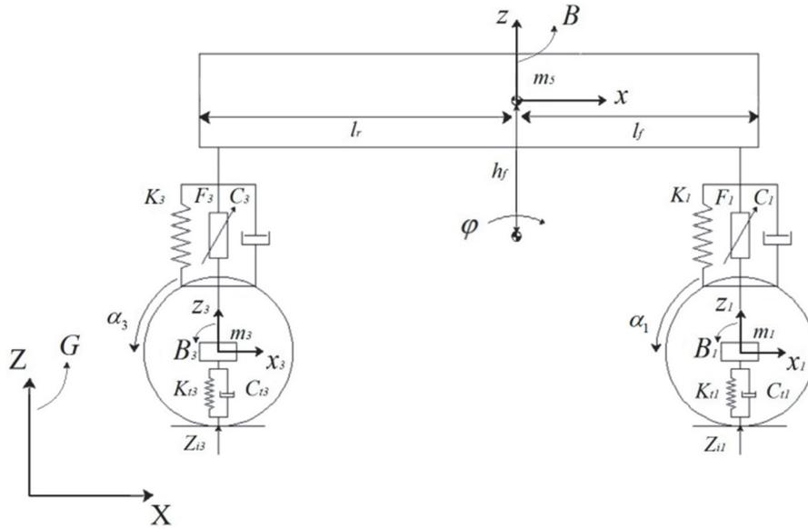
Figure 2. 1 Side view (right) of the suspension system model
