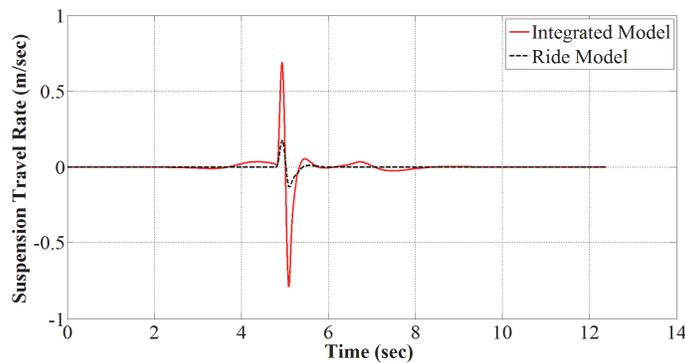
Figure 2. 9 Suspension travel rate of front left wheel
