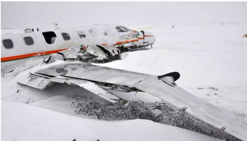
Figure 1.2 Accumulation of snow on the wing of an airplane leading to a deadly crash [30]
