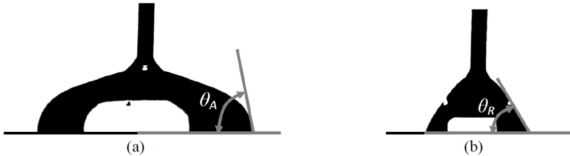
Figure 2.12 Real images of a 20 \mu\text{m} droplet (a) advancing and (b) receding contact angles
