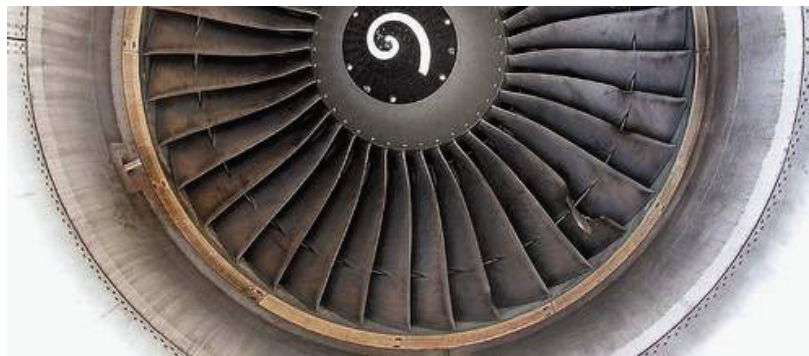
Figure 2.17: Turbine blade damage caused by foreign object [230].
