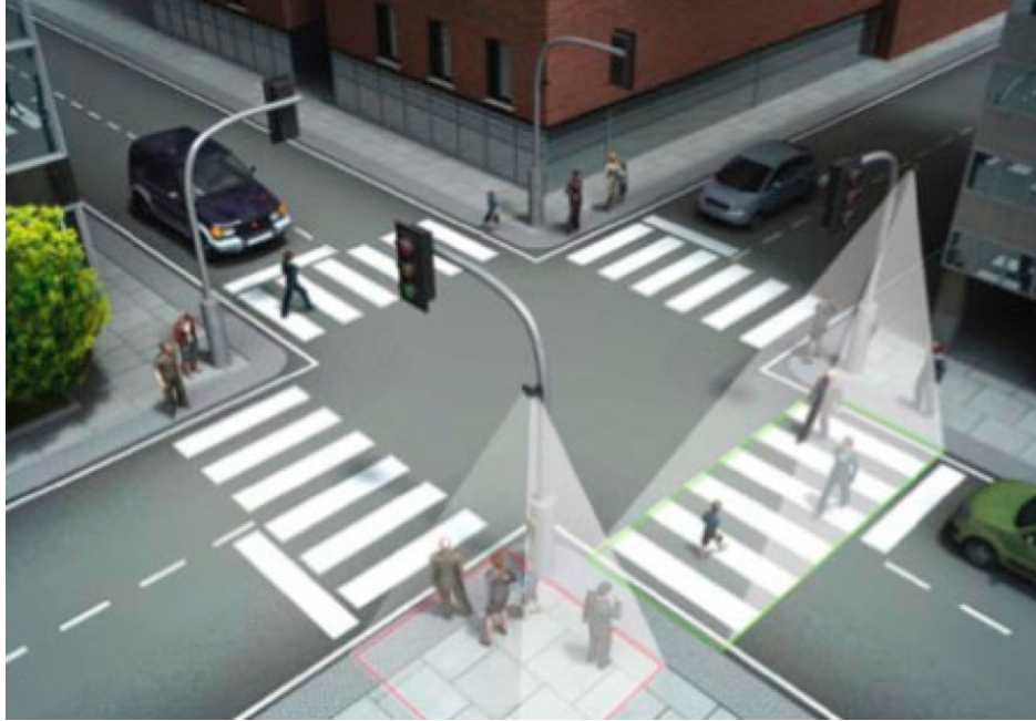
Figure 13: Pedestrian detector using video image processor [22]
