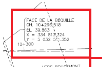
Figure 62 - Chainage and elevation of a bridge abutment
