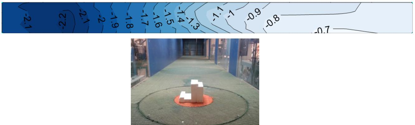
**Figure 3.10:** Mean pressure coefficient ( $C_{p\_mean}$ ) for 90° wind direction (top) and wind tunnel model placement (bottom).
