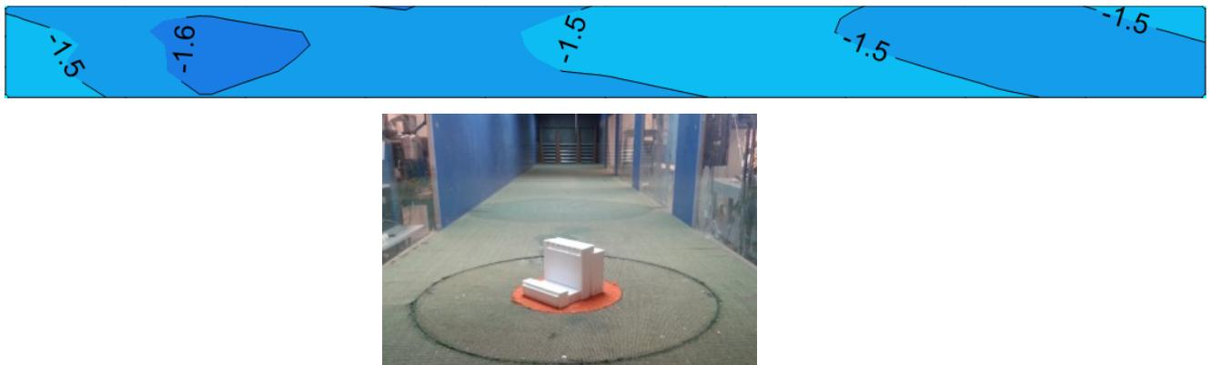
**Figure 3.11:** Mean pressure coefficient ( $C_{p\_mean}$ ) for 135° wind direction (top) and wind tunnel model placement (bottom).
