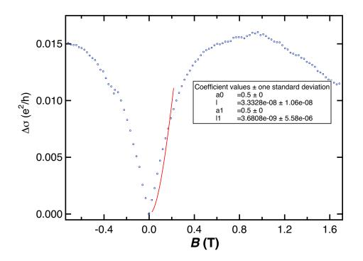
Figure 4.2.4: Fixing  $\alpha = 0.5$  we find the HLN model does not fit the data, suggesting the low-field peak is not due to WAL
