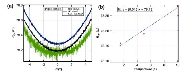
Figure 5.2.2: (a) Magnetic-field dependence of sample E at T = 1.5, 5, 10 K, (b) The 2-point resistance at B = 0 Tesla
