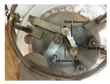
Figure 2.4.5: Current is passed through either a Chromium bar or a Gold nugget, creating metal vapour under vacuum
