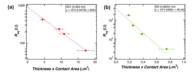
Figure 3.2.6: In two samples of thickness (a) t = 352 nm and (b) t = 38 nm, 22 nm, the contact resistance per unit area scales logarithmically with the volume of the contact, defined by contact area times sample thickness.
