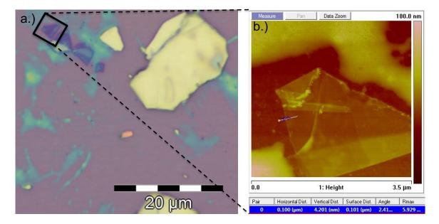
Figure 2.3.2: Thin flake characterization: a.) Optical and b.) Atomic Force Microscope images of a 6 nm-thick exfoliated  $Bi_2Se_3$  flake
