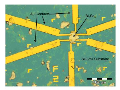
Figure 2.0.1: Photolithographically defined electrodes on a  $Bi_2Se_3$  crystal with a Hall bar geometry
