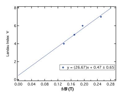
Figure 4.3.2: Landau fan diagram for sample C (t = 38 nm, T = 1.5 K) shows the filling fraction assignment vs 1/magnetic field
