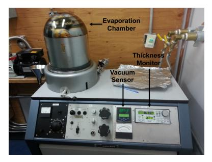
Figure 2.4.4: Metal deposition of the contacts is done using a diffusion pumped thermal evaporator
