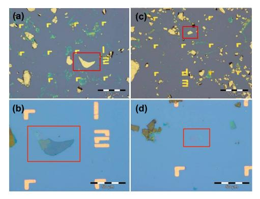
Figure 3.3.1: Non selective Argon plasma etches the surface of  $Bi_2Se_3$  crystals: (a) An opaque flake of a higher thickness is reduced to the point of becoming translucent, shown in (b). The smaller flake in panel (c) is reduced to effectively nothing in (d)
