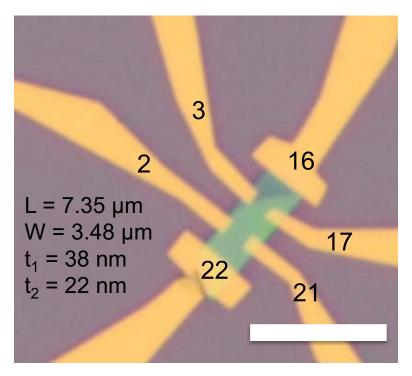
Figure 1.2.2: Mechanically exfoliated  $\rm Bi_2Se_3$  of 22 nm with lithographically defined Gold electrodes. Scale bar is 10  $\mu m.$
