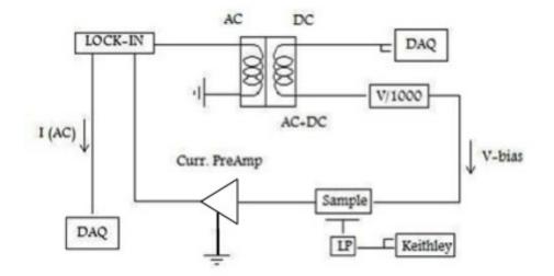
Figure 2.5.3: Our AC circuit uses a transformer to add an AC perturbation atop a DC source signal
