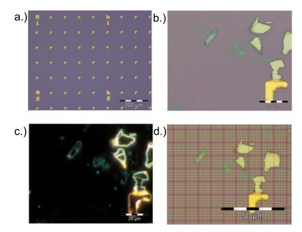
Figure 2.4.2: a.) Prepatterned Gold reference grid for flake location b.)  $Bi_2Se_3$  flakes are exfoliated onto the grid c.) Dark field imaging shows surface and edge uniformity, suggesting the crystalline nature of the flake d.) Optical image overlaid with a digital coordinate system for CAD design of EBL electrodes
