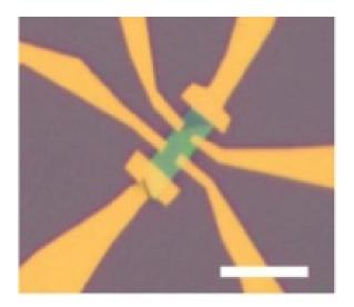
Figure 2.4.3:  $Bi_2Se_3$  flake with Hall bar geometry after metal electrode evaporation (scale bar is 10  $\mu$ m)
