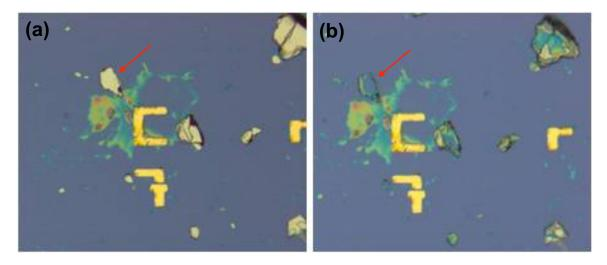
Figure 3.2.1: (a) Freshly exfoliated  $Bi_2Se_3$  crystal flakes, (b) Left in open air for 3 months, the crystals are severely degraded
