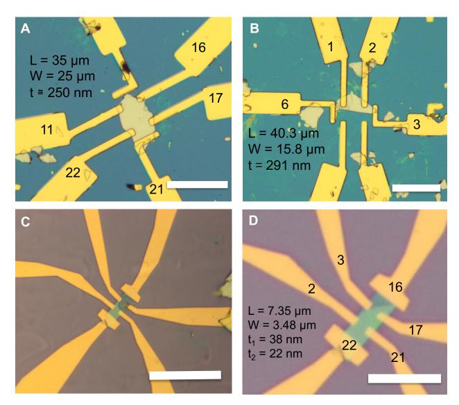
Figure 4.1.1: Samples to be discussed in this chapter a.) & b.) Scale bar = 50  $\mu$  m c.) & d.) Scale bar = 10  $\mu$  m
