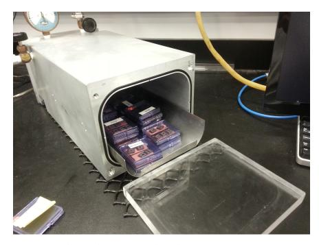
Figure 2.4.8: Prepared samples are stored under vacuum to minimize exposure to air
