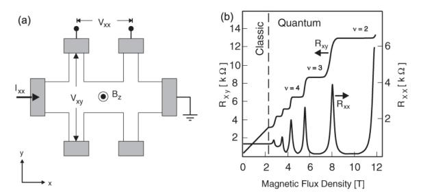
Figure 4.1.3: a.) 6-point Hall Bar geometry b.) Longitudinal and transverse Hall resistance. Figure from Janssen et al. [35]
