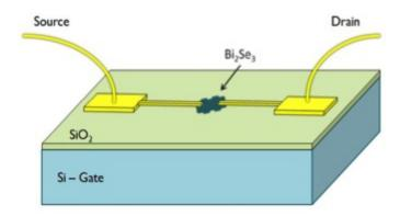
Figure 2.4.1: Source and drain electrodes physically contact the  $Bi_2Se_3$  crystal, while the gate is capacitively coupled via the  $SiO_2$  dielectric film.
