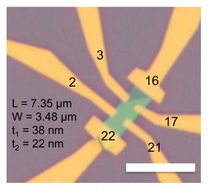
Figure 5.1.1: Mechanically exfoliated  $Bi_2Se_3$  of 22 nm with lithographically defined Gold electrodes. Scale bar is  $10\mu m$ .
