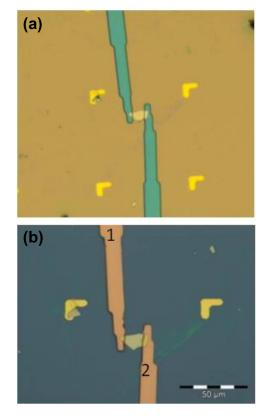
Figure 3.3.2: (a) After defining electrode positions using photolithography, a plasma etch is done to clean the exposed area of  $Bi_2Se_3$  under the contacts (b) Metal electrodes are evaporated and the photoresist is lifted off, resulting in a sample with gold contacts on the surface
