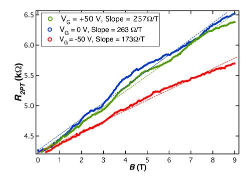
Figure 4.1.6: Resistance vs magnetic field for different gate voltages. The slope of linear fits: (+50V): 257  $\Omega/T$ , (0V): 263  $\Omega/T$ , (-50V): 173  $\Omega/T$
