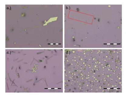
Figure 2.2.2: Vapor-Solid growth from powderized  $Bi_2Se_3$  a.) Interesting step-like growth results in a nanoribbon attached to a planar crystal with many corners b.) 50  $\mu$ m long nanoribbon c.) X-shaped crystals d.) Triangular and hexagonal stacked nano plates.
