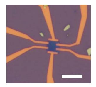
Figure 3.1.3: Ultrathin  $Bi_2Se_3$  crystal with EBL defined contacts (Scale bar = 10  $\mu$ m)
