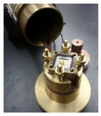
Figure 2.5.1: Sample testing: A packaged sample, loaded in the measurement probe of our  ${}^{3}$ He cryostat
