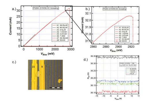
Figure 5.2.3: Joule Heating in suspended sample E: a.) Repeatedly ramping up the current b.) Current saturation leading to device failure c.) Optical image of suspended sample d.) Gatesweeps show resistance is converging with annealing
