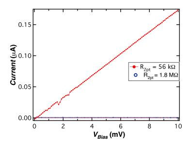
Figure 3.1.5: I - V plot shows a linear source/drain dependence. 2pt resistance is extracted from the slope
