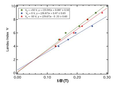
Figure 5.1.2: Landau fan diagram showing the filling fraction assignment vs 1/B, for sample C with thickness 38 nm, at T = 1.5 K
