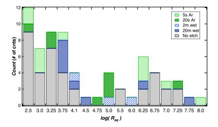
Figure 3.3.3: Number of contacts vs  $\log(R_{sq})$  for many devices whose contacts were made with 5s and 20s long Ar RIE etches, 2m and 20m TCE cleaning and without any additional contact cleaning
