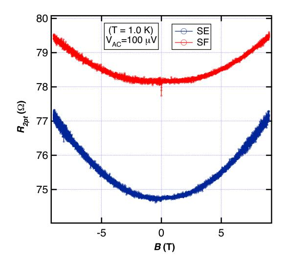
Figure 5.2.1: Magnetic-field dependence of suspended topological insulator transistors E and F at  $T=1~{\rm K}$
