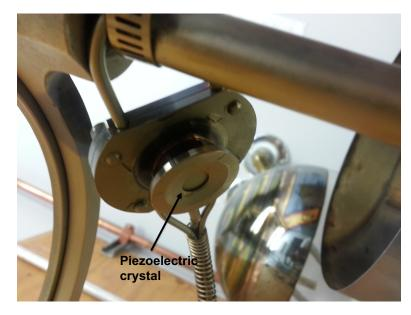
Figure 2.4.6: The resonance frequency of the crystal thickness monitor is measured by a RF circuit, and is sensitive to nanometer thick metal layers
