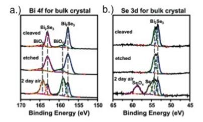
Figure 3.2.2: (a) Bi and (b) Se XPS Spectra for  $Bi_2Se_3$  shows the formation of an oxide layer over 2 days, with both Bi and Se binding to Oxygen in the air. Samples etched with an Argon plasma (middle panel) display a reduction in the level of oxidation [7]
