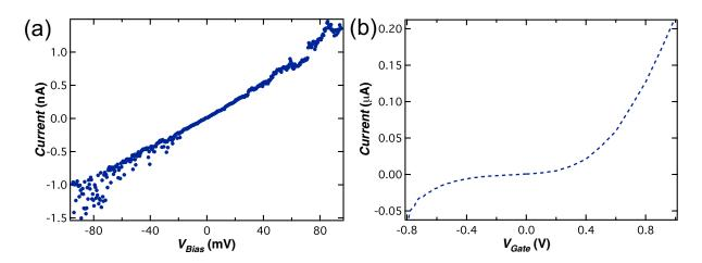
Figure 3.1.4: (a) A 2-point bias sweep reveals a large resistance  $R = 74 \text{ M}\Omega$ , and shows disorder, (b) With constant source/drain voltage, the gate voltage is swept over  $\pm 1 \text{ V}$ . A breakdown of the SiO<sub>2</sub> substrate leads to the backgate making a current connection directly to the gold electrodes
