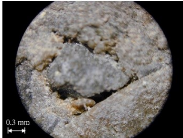
Figure 2-17: The cracks on the interface of the aggregate and cement paste with w/cm = 0.05 (Liu et al., 2006)
