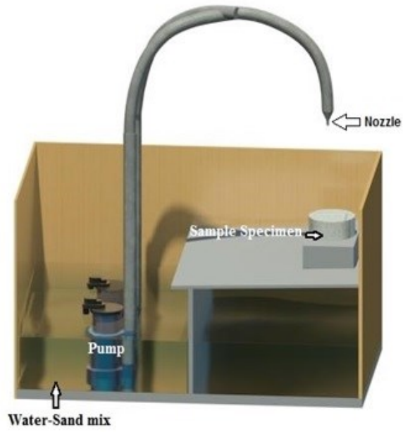
Figure 3-8: Schematic diagram of abrasion test apparatus.
