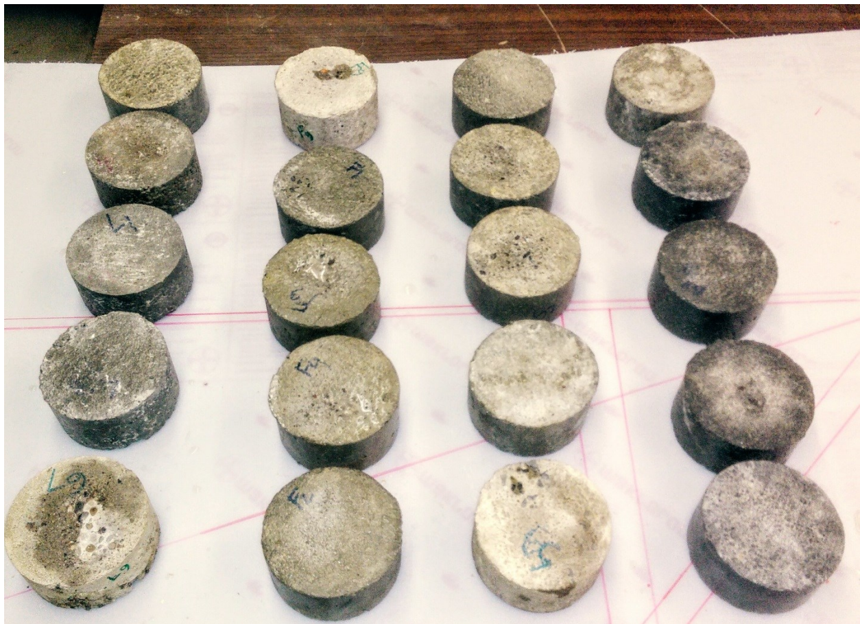
Figure 4-2: Image of sample specimens used in abrasion test. From left: a) Latex modified material, b) Fly ash modified material c) Concrete material d) Silica fume modified material
