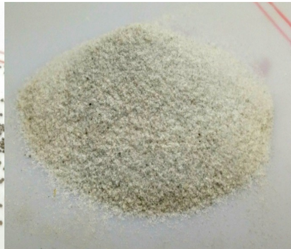
Figure 3-5: Fine Silica used in this study which is 40% of total abrasive particle.
