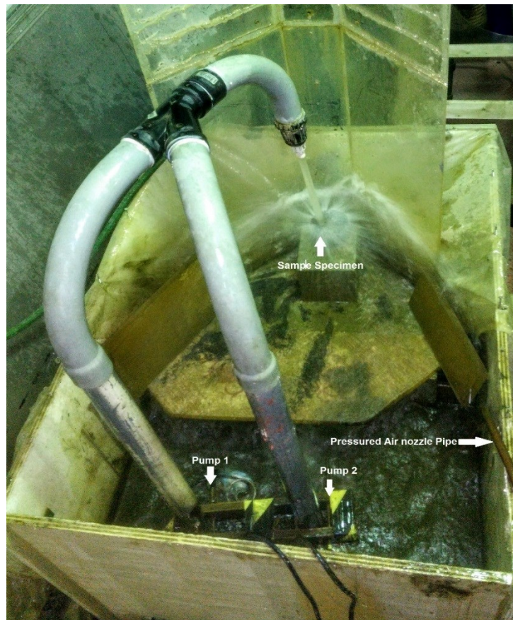
Figure 3-8: Schematic diagram of abrasion test apparatus.
