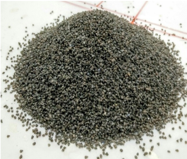
Figure 3-4: Aluminum Oxide particle used in this study which is 60% of total abrasive material
