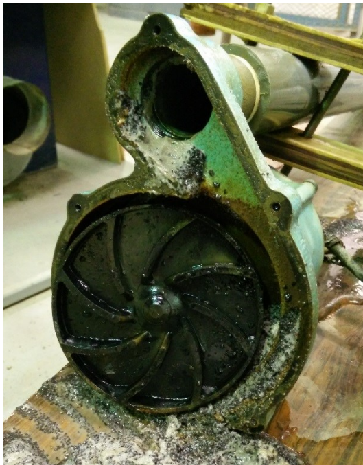
Figure 3-7: Blockage problem of the pump due to the usage of larger particles.
