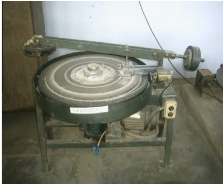
Figure 2-29: IS 1237-1980 Abrasion test machine (Siddique et al., 2012)
