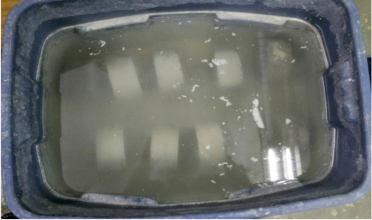
Figure 3-1: Curing of abrasion sample specimens in lime water.
