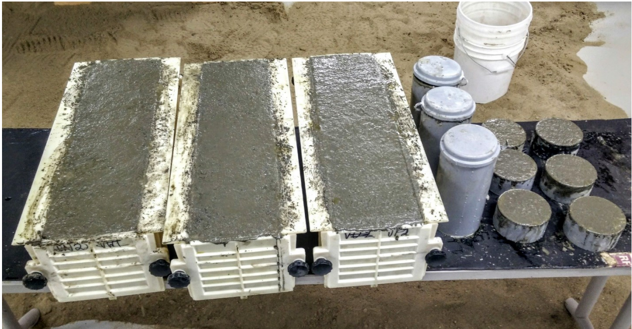
Figure 3-2: Casting of beam, cylinder, and abrasion test samples.
