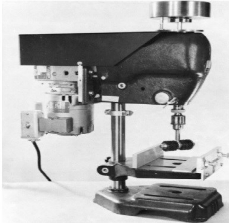
Figure 2-6: The Rotating cutter drill press (ASTM C944, 2012).
