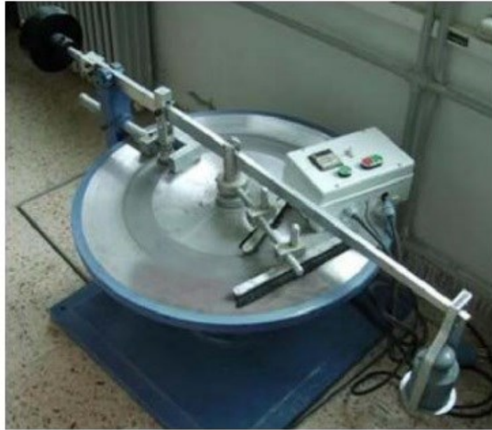
Figure 2-13: Abrasion Test apparatus as specified in TS699 (Gencil et al., 2011)
