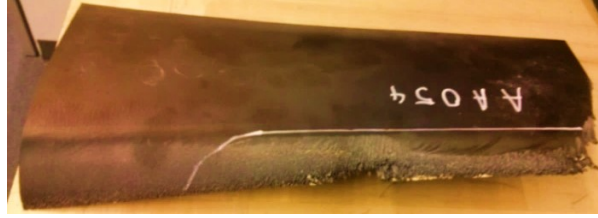
Figure 1.2 Eroded ex-service turbine blade
