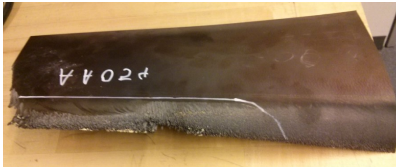
Figure 3.12 Eroded blade with sever erosion marks
