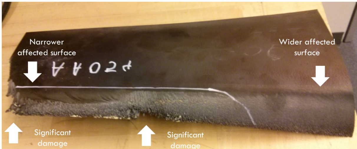
Figure 6.2 Eroded surface area of Blade 2
